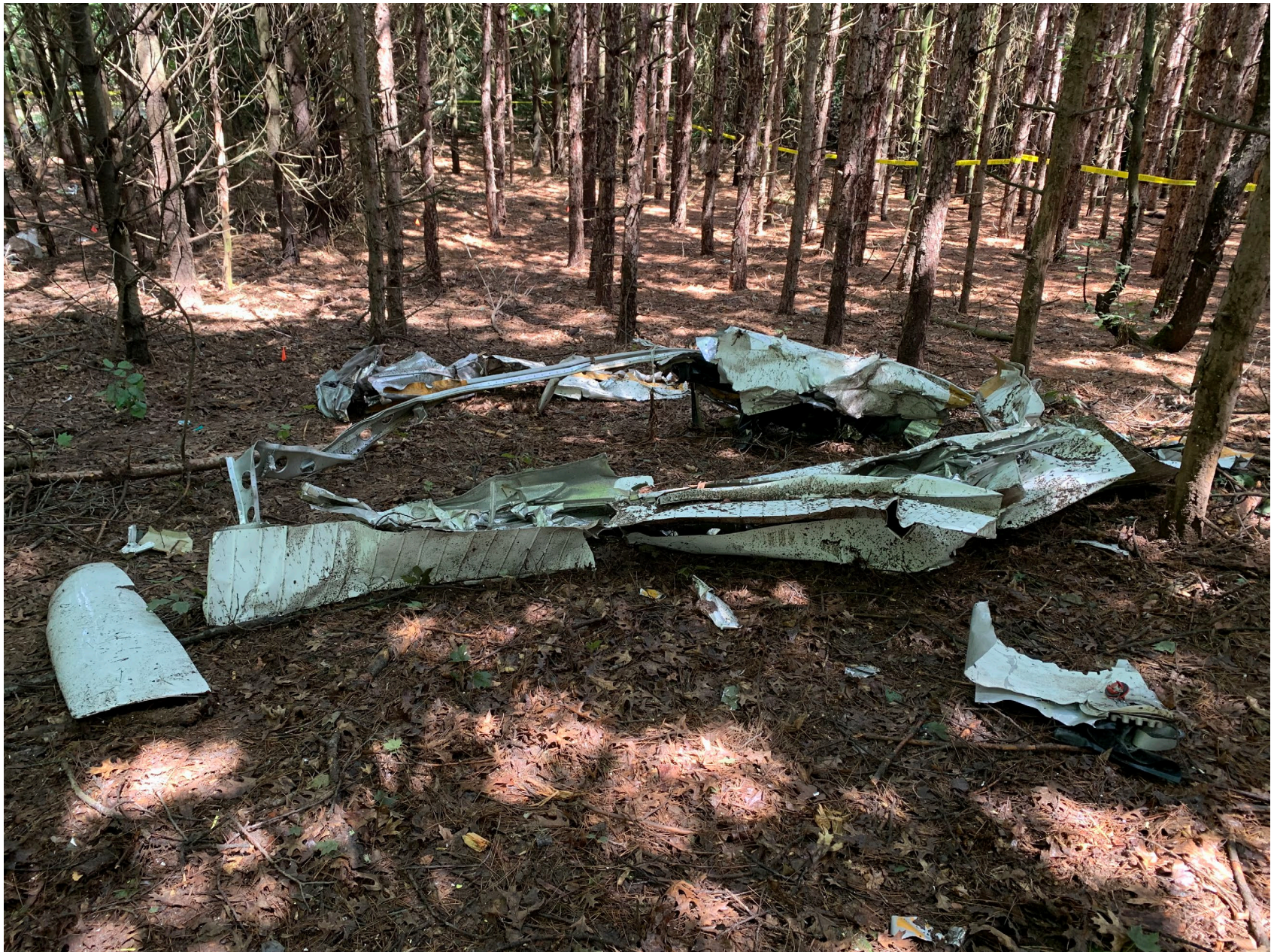
Photo 4 – Left Wing Fragments (NTSB Photo)
