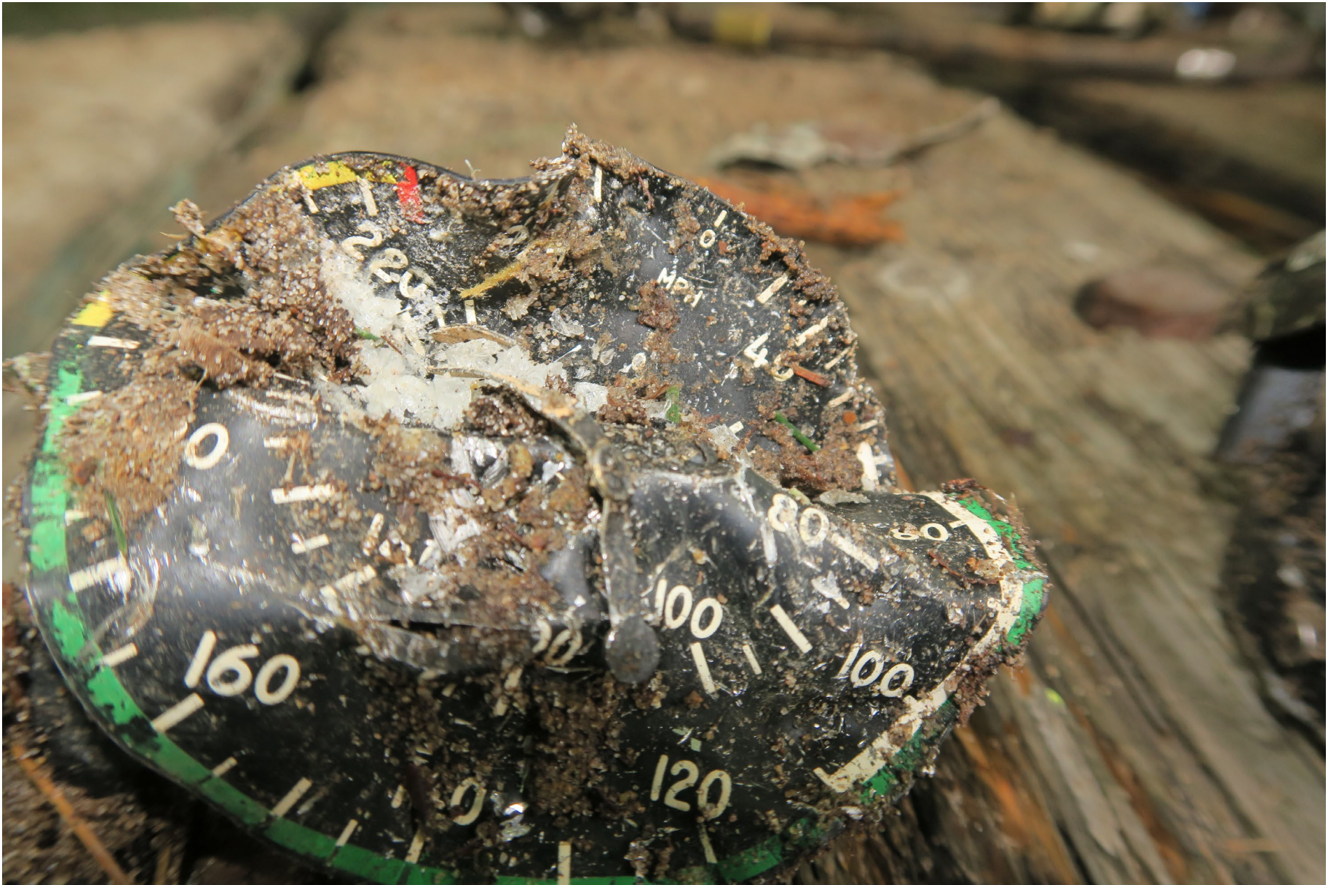
Photo 10 – Airspeed Indicator Face (Textron Aviation Photo)
