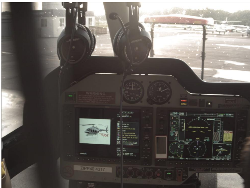
Figure 2. The field of view of the Appareo Vision 1000 device, as installed on the accident helicopter N98ZA.
