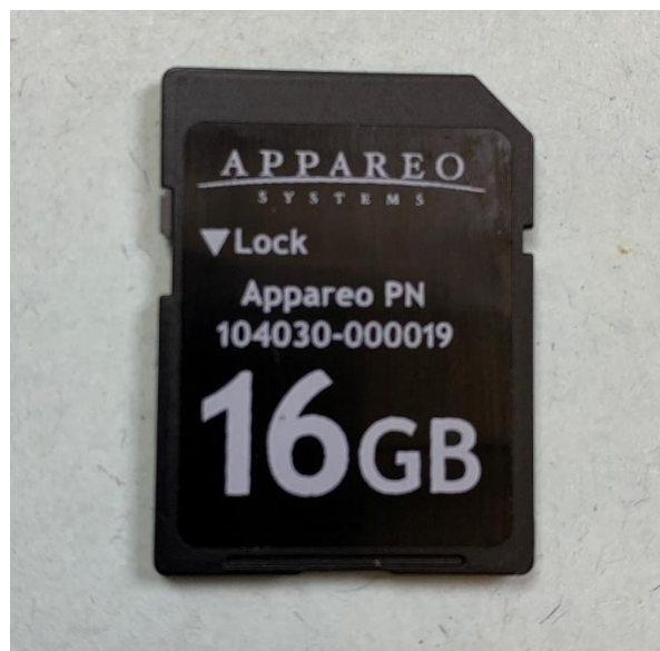
Figure 1. The device's internally mounted, externally removable SD card.
