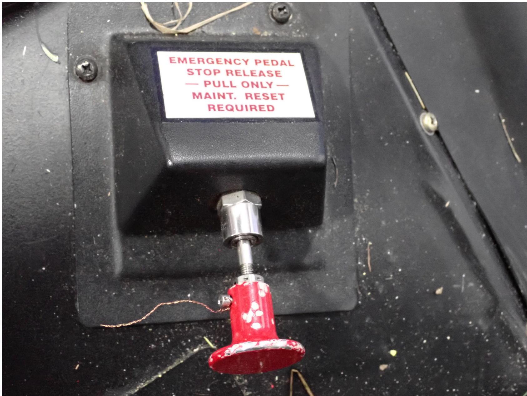
Photo 2 – View of Emergency Pedal Stop Release in Deployed Position (Bell)
