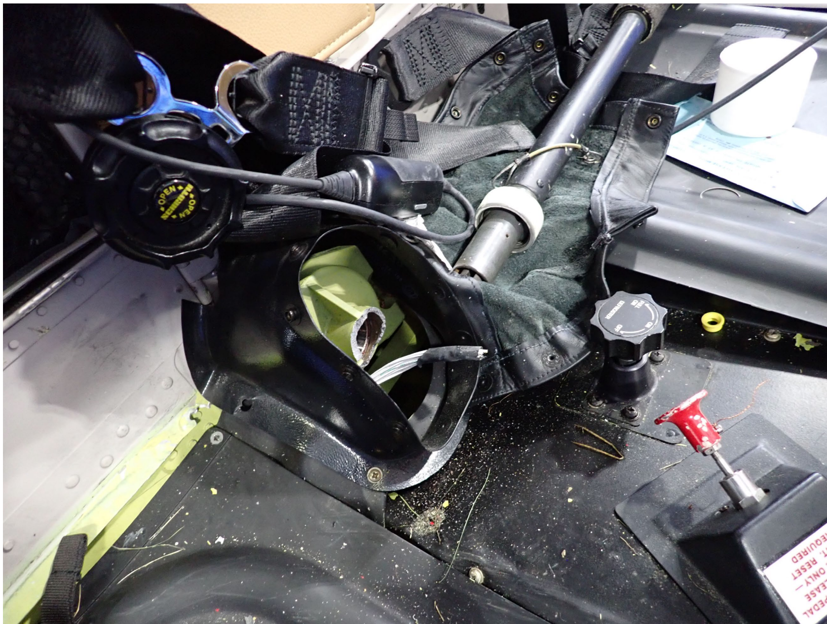
Photo 3 – View of Emergency Pedal Release Proximity to Pilot’s Collective Control (Bell)
