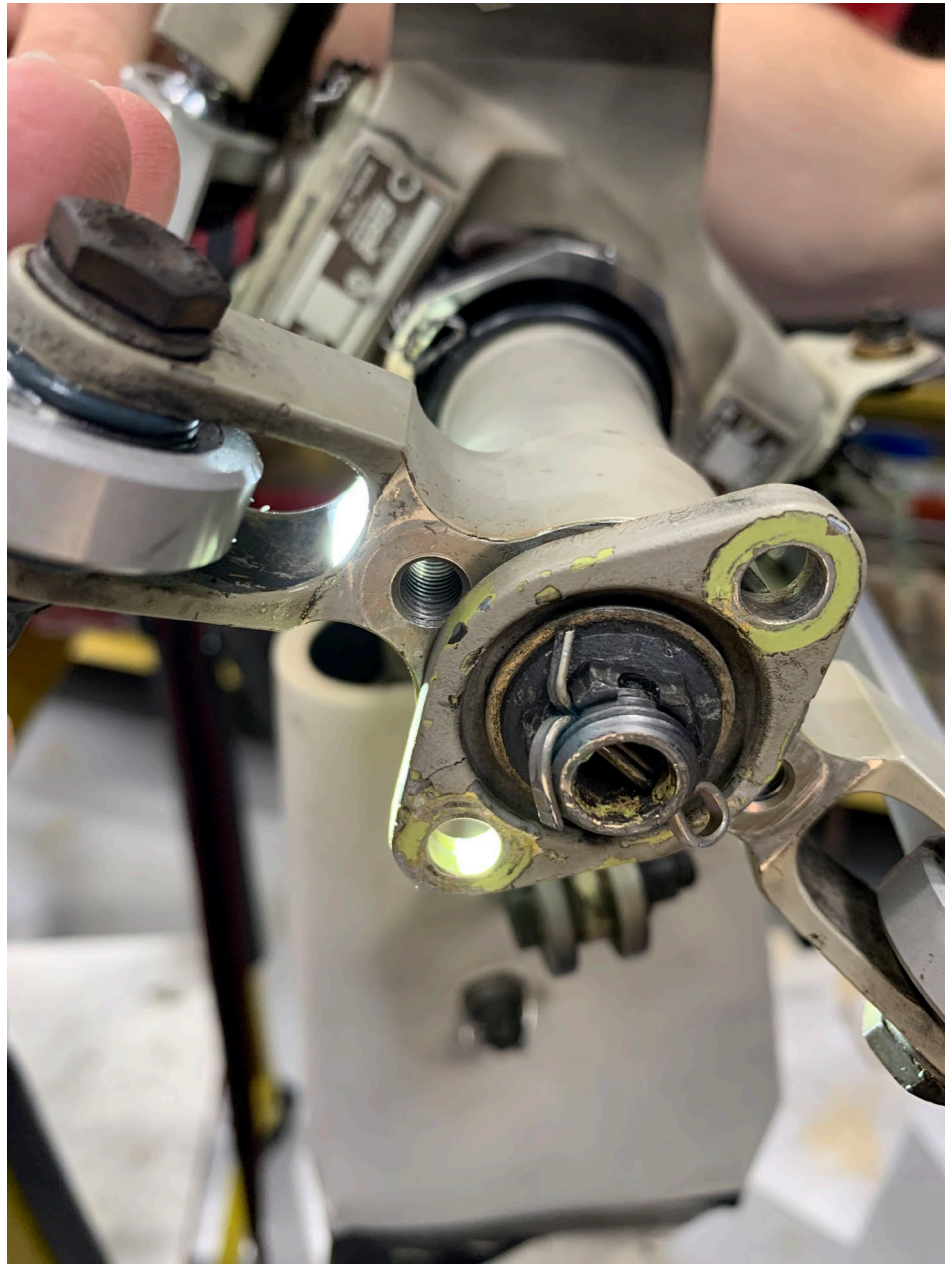
Photo 5 – View of Tailrotor Crosshead/Driveplate Assembly as Found (Bell)
