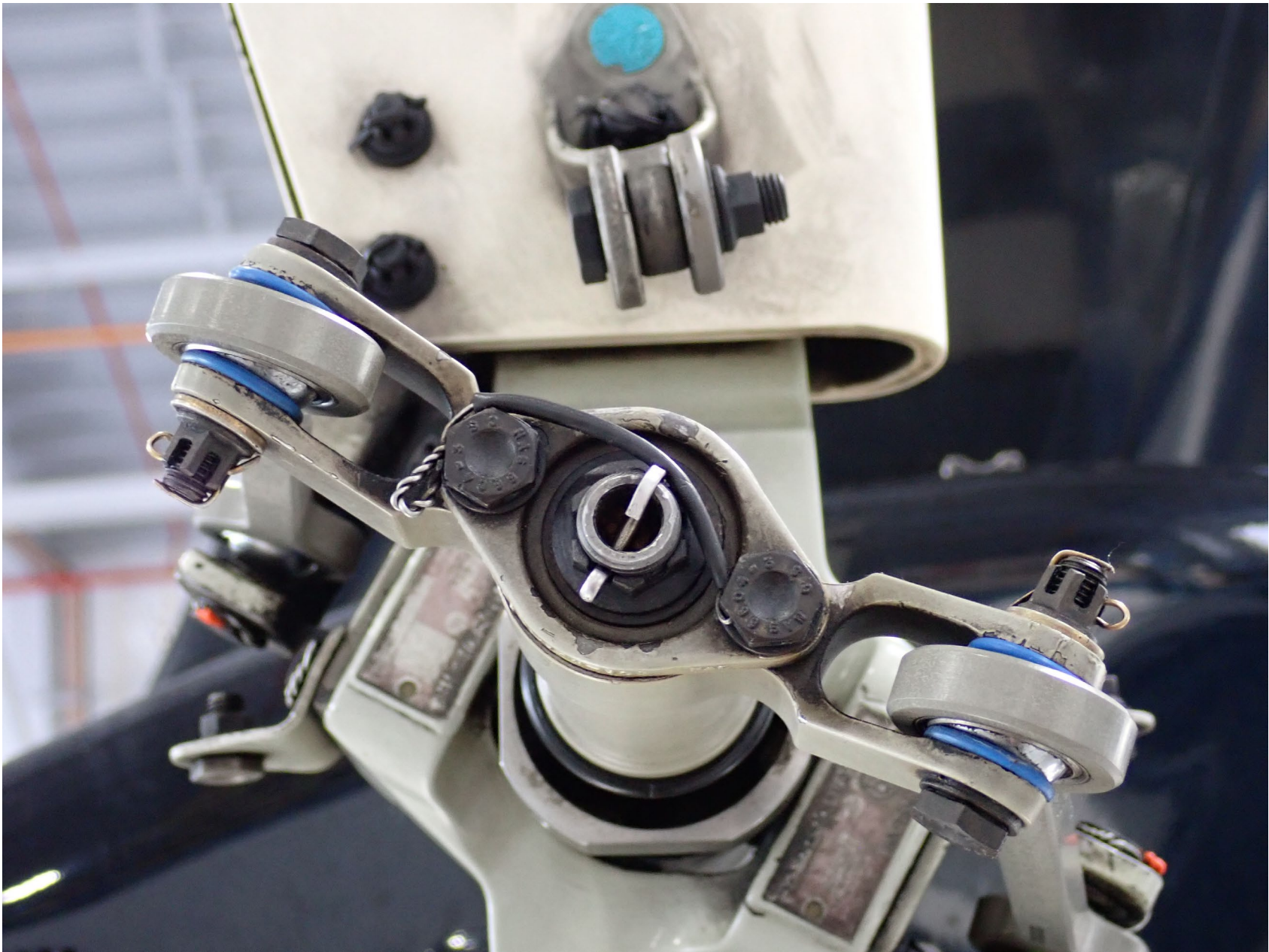
Photo 4 – View of Exemplar Tailrotor Crosshead Fully Assembled and Safety-Wired (Bell)
