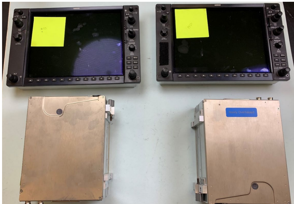
Figure 1. Two Garmin G1000's and the associated LRU's in good condition.
