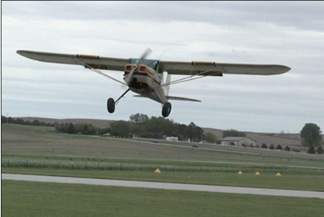
Figure 16: Image of the accident airplane approaching for its second STOL landing, which was the approach and landing preceding the accident approach. Note the visual appearance of the extension of the flaps.
