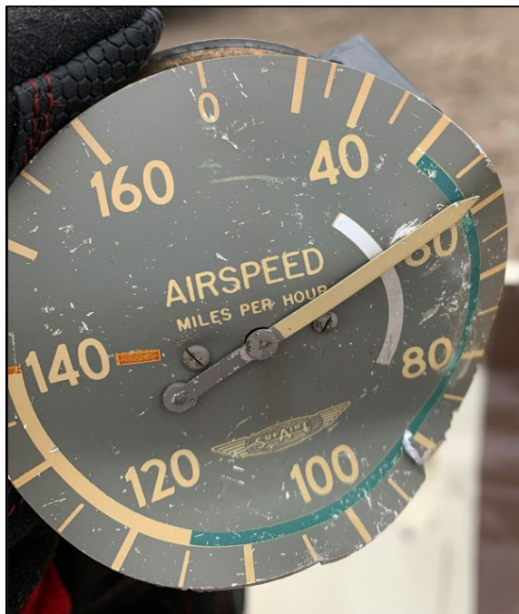
Photo 5: View of the airspeed indicator as found indicating about 57 MPH.
