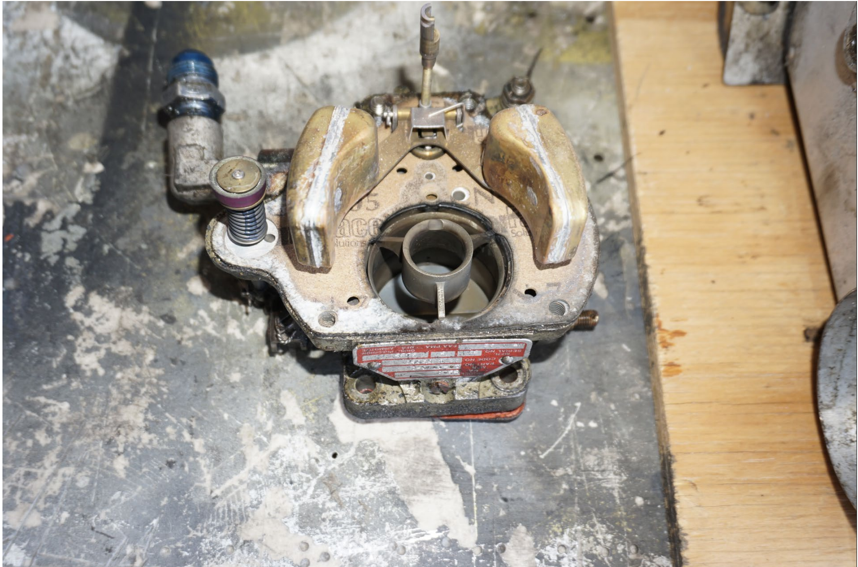
Photograph 19 - Carburetor Floats and Accelerator Pump
