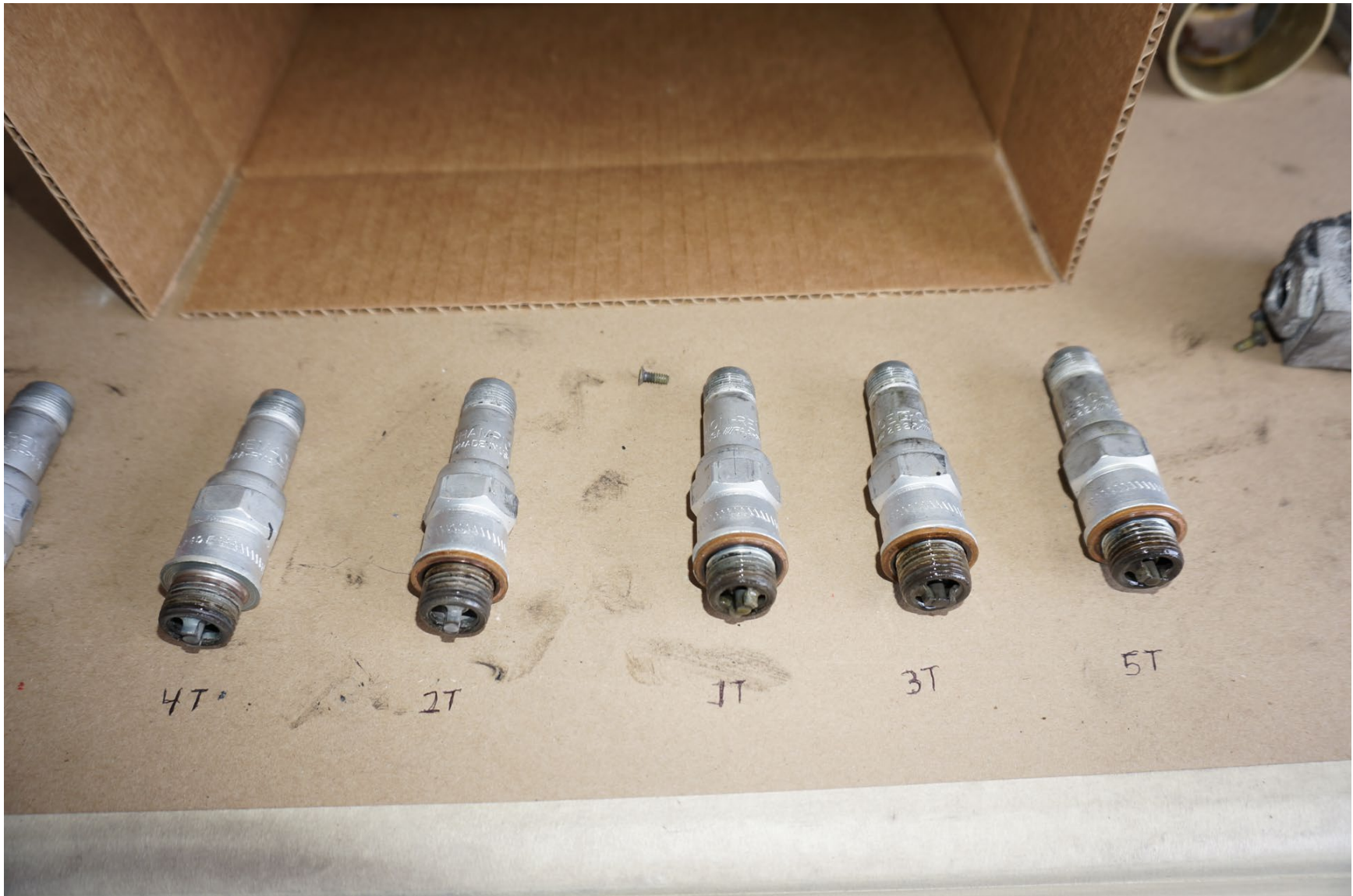
Photograph 23 - Top Spark Plugs (Second Photo)
