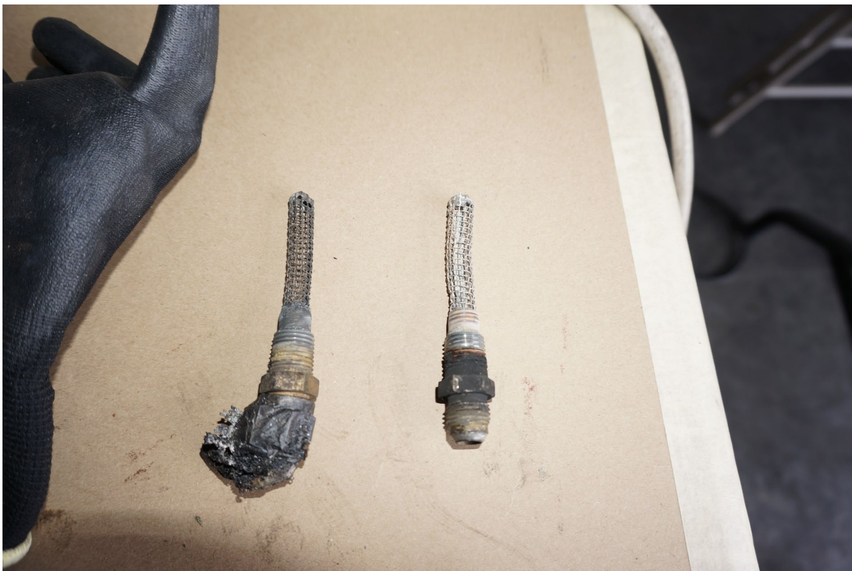
Photograph 28 - Fuel System Finger Screens
