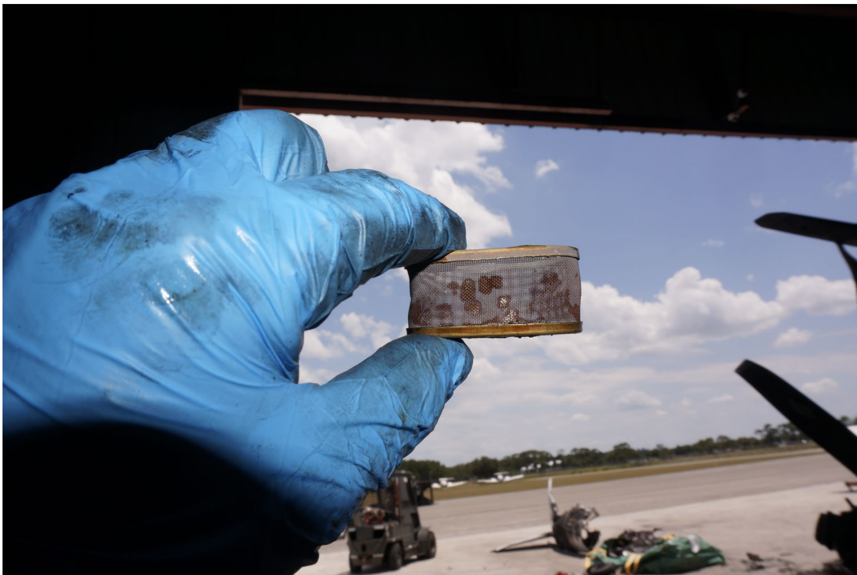
Photograph 25 - Fuel Strainer Screen
