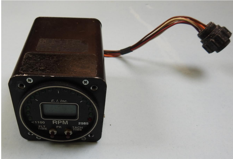
Figure 1. EI R-1 tachometer as received.
