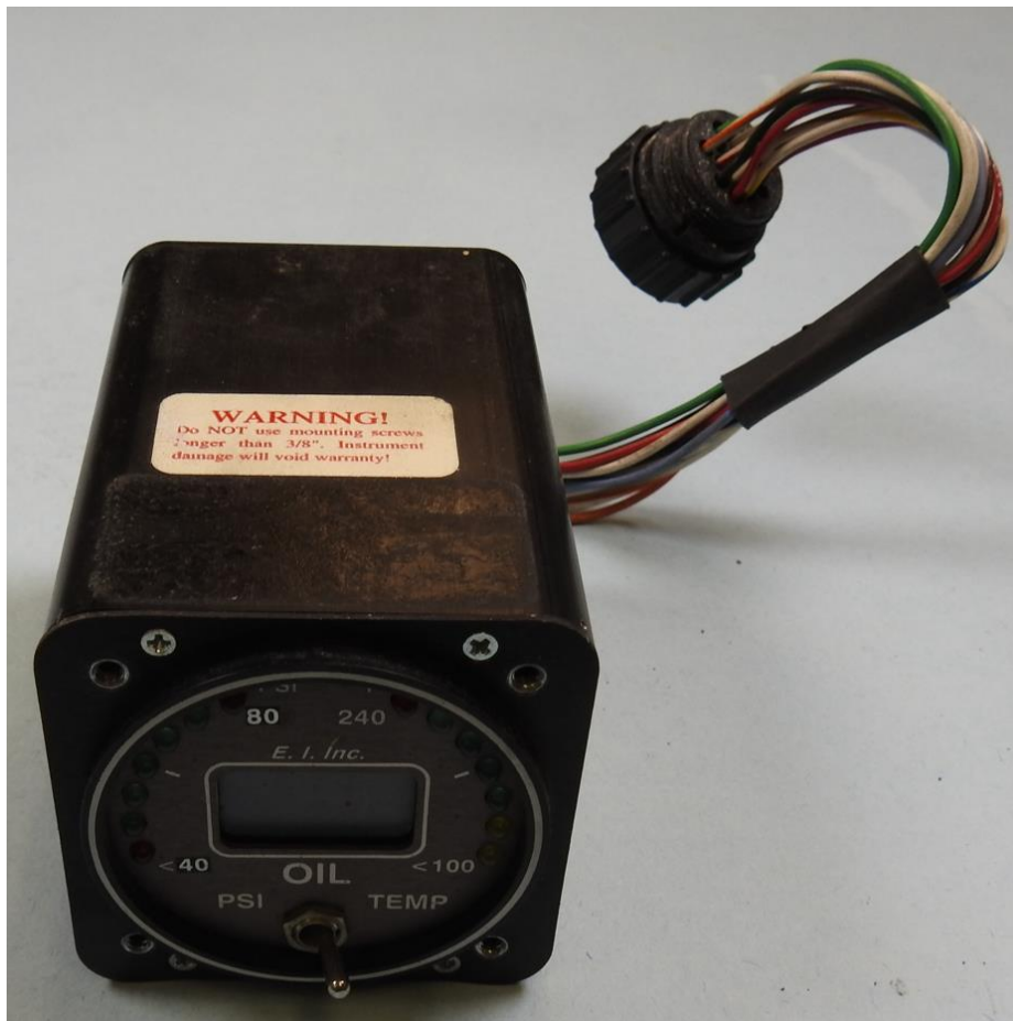
Figure 2. EI OPT-1 Oil Pressure and Temperature gauge as received.
