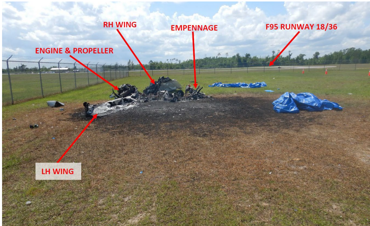
N6413B Wreckage Pattern (Provided by Textron Aviation)
