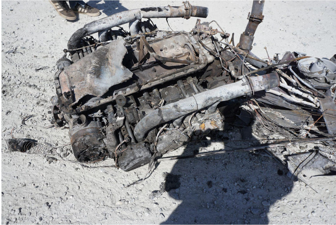
Photograph 4 - Left engine showing fire damage
