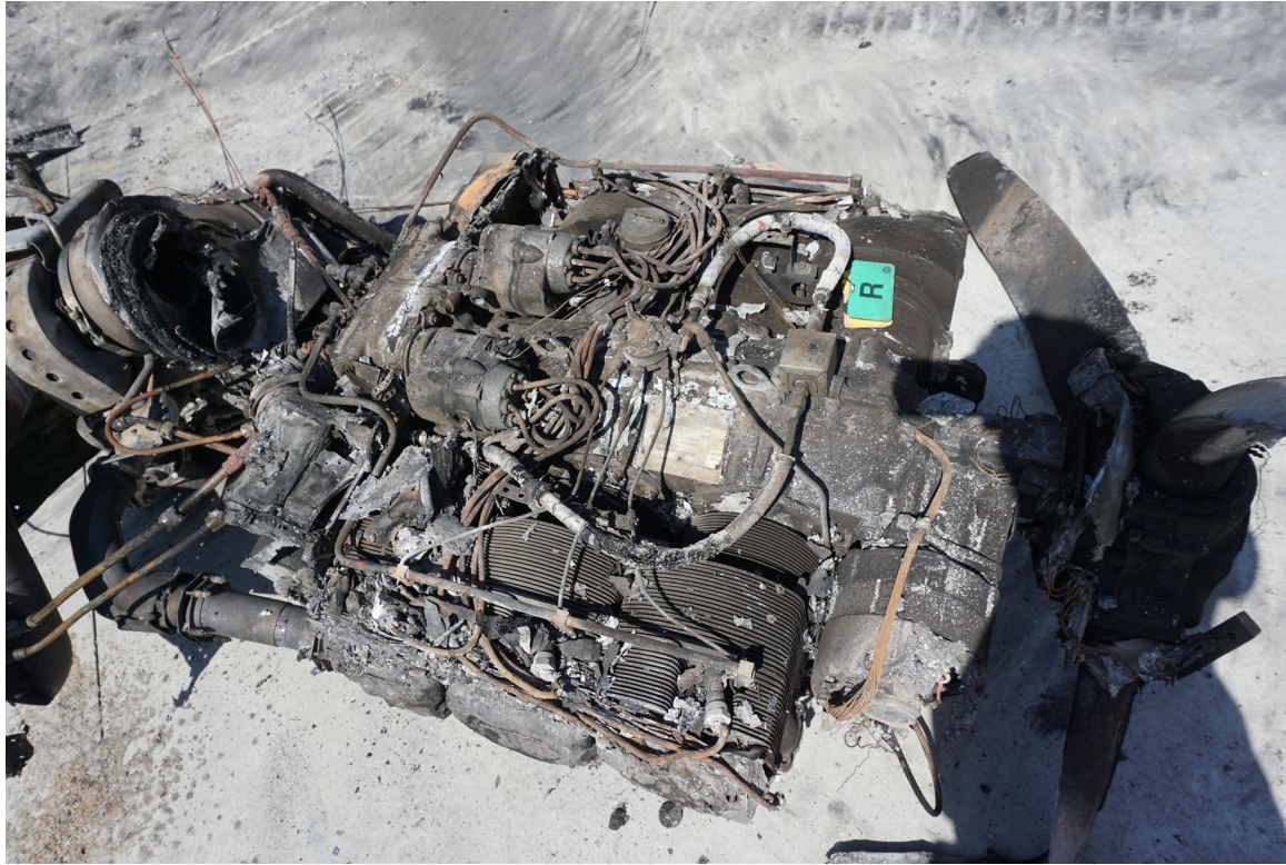
Photograph 3 - Right engine showing fire damage
