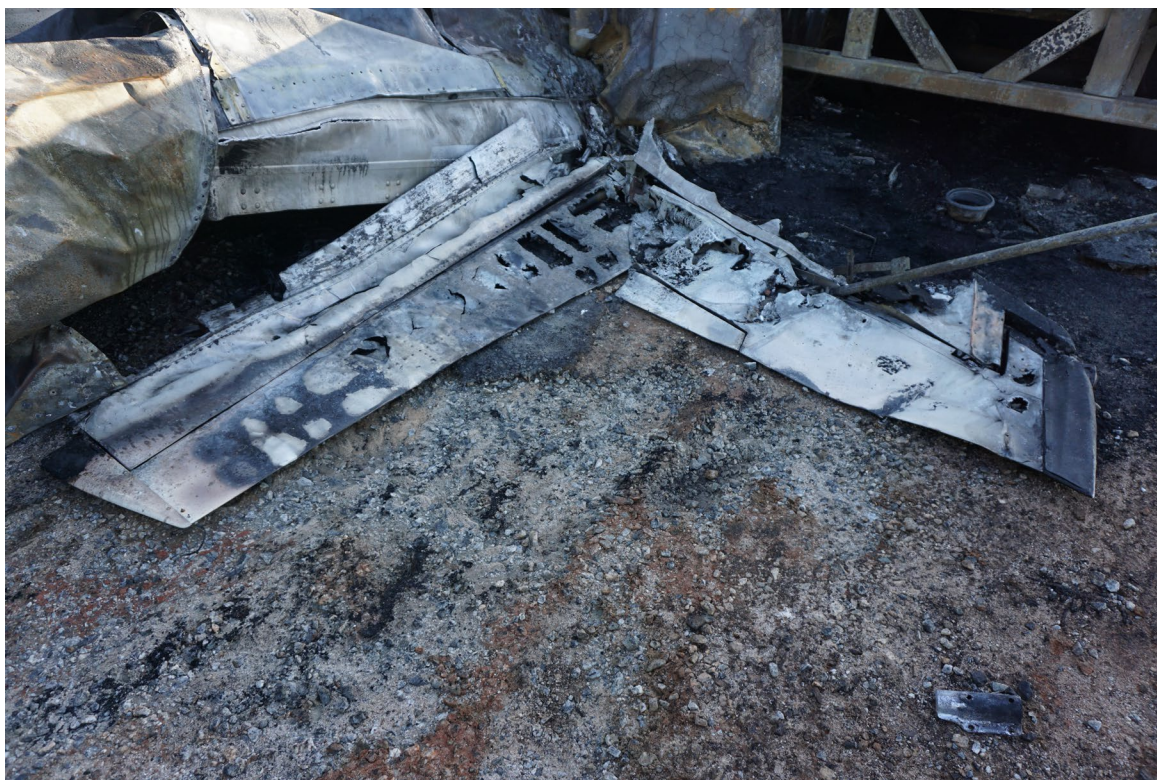
Photograph 5 - Fire damaged vertical and horizontal stabilizer
