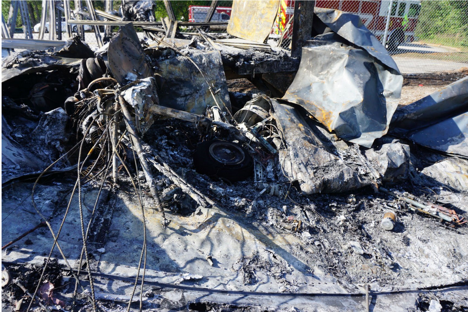
Photograph 1- Fire damaged airplane hull.
