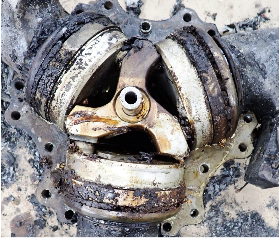
Photo #8 - Left propeller internal heat damage
