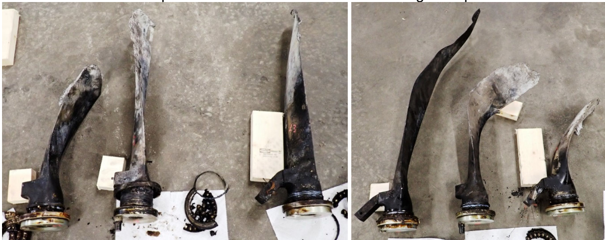
Photo #1 – Propeller blade damage comparison Left Propeller Right Propeller
