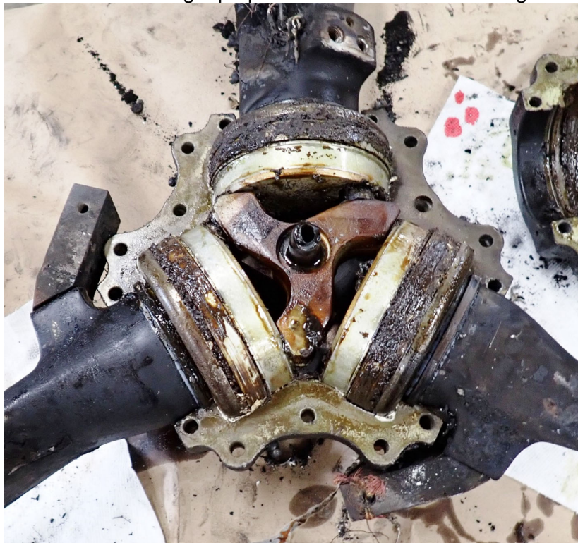
Photo #19 - Right propeller internal hub heat damage
