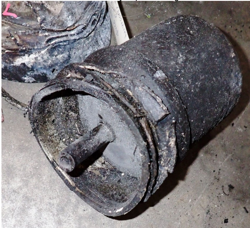
Photo #5 - Left propeller hydraulic unit (cylinder, piston, feathering spring) cut from assembly at pitch change rod
