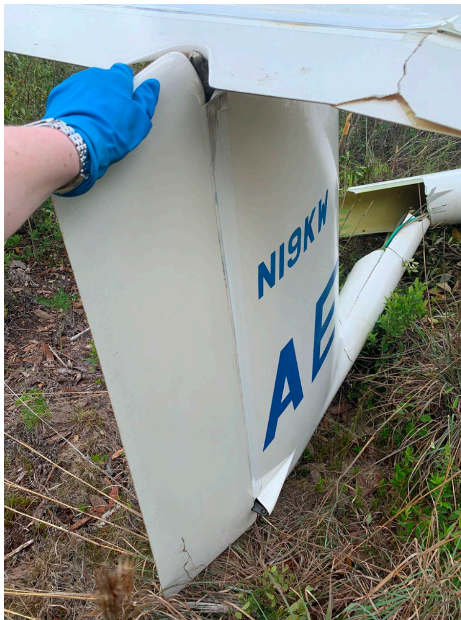
Photo 4 -Tail section with up end of the elevator connection visible between elevator and horizontal stabilizer
