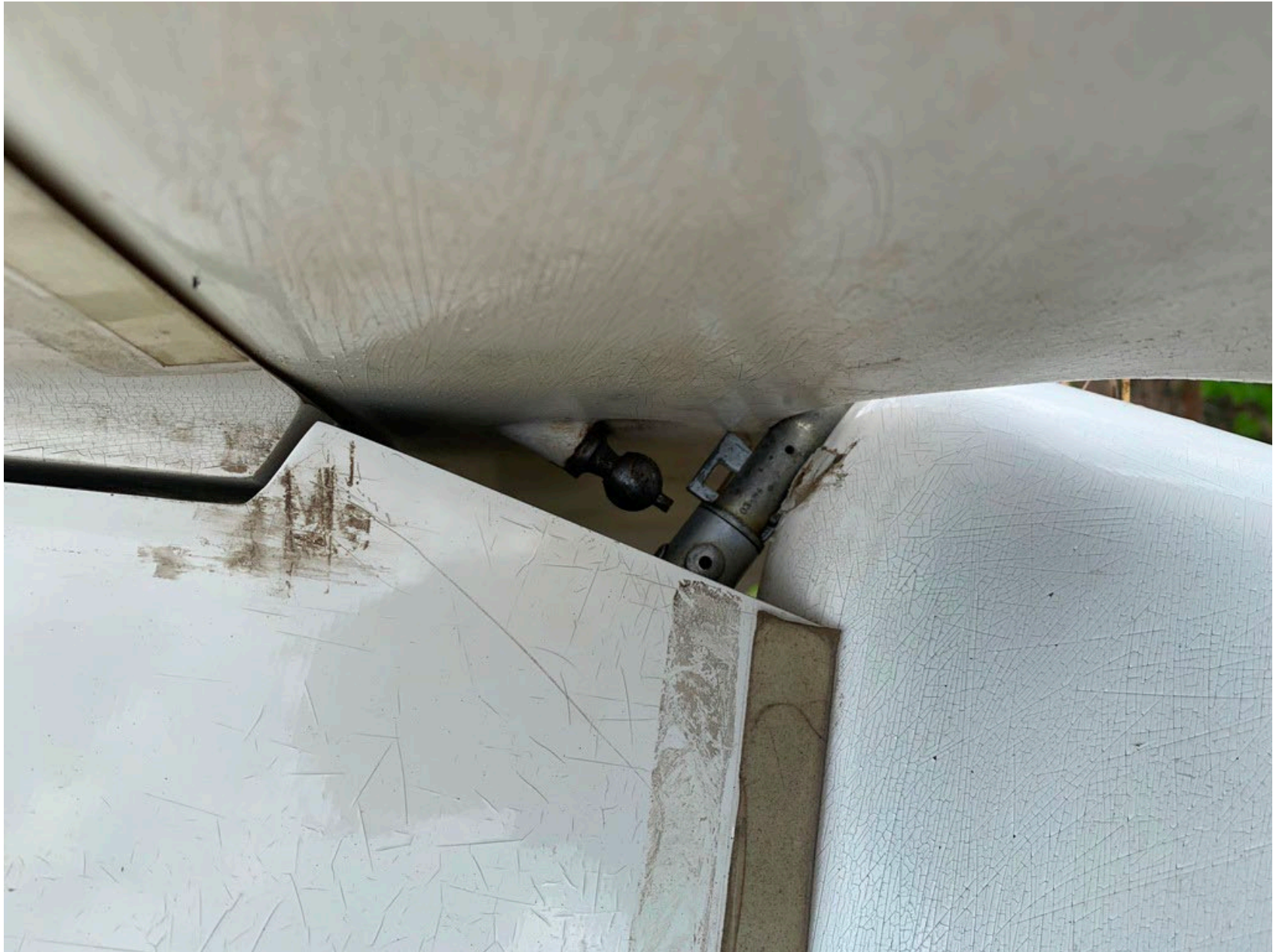
Photo 5 - Left side view of elevator connection (not connected)
