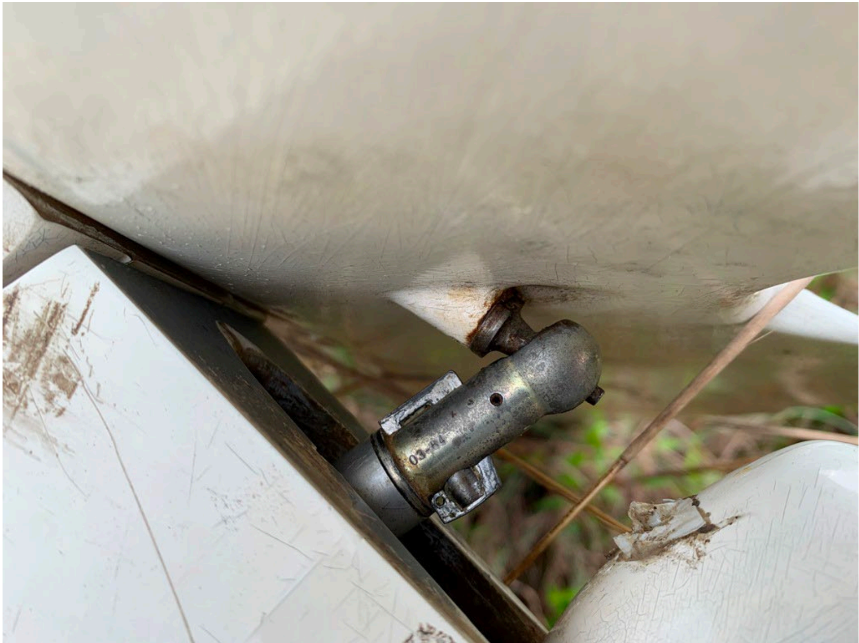
Photo 6 - Left side view of elevator connection (connected by NTSB IIC). Note: the drill hole for the spring clip is visible below the number stamps.
