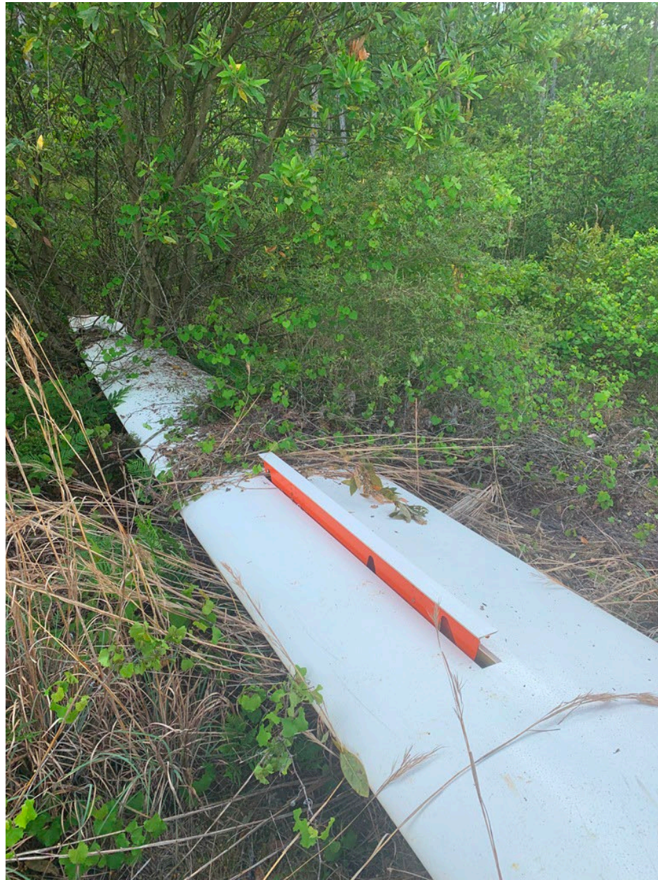
Photo 3 - Right wing with speed brake deployed
