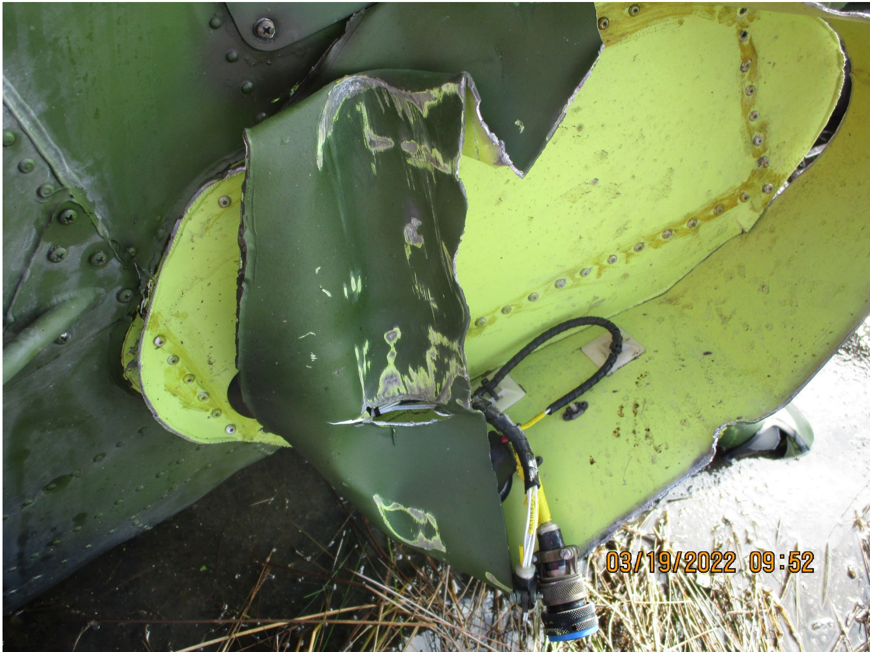
Photo 5 – Powerline impression mark on landing light housing
