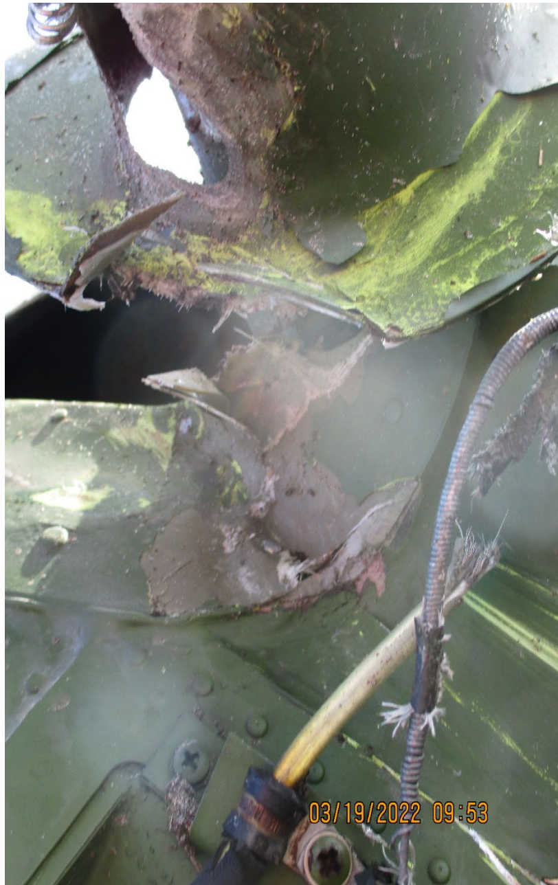
Photo 7 – powerline impression mark on bottom of helicopter
