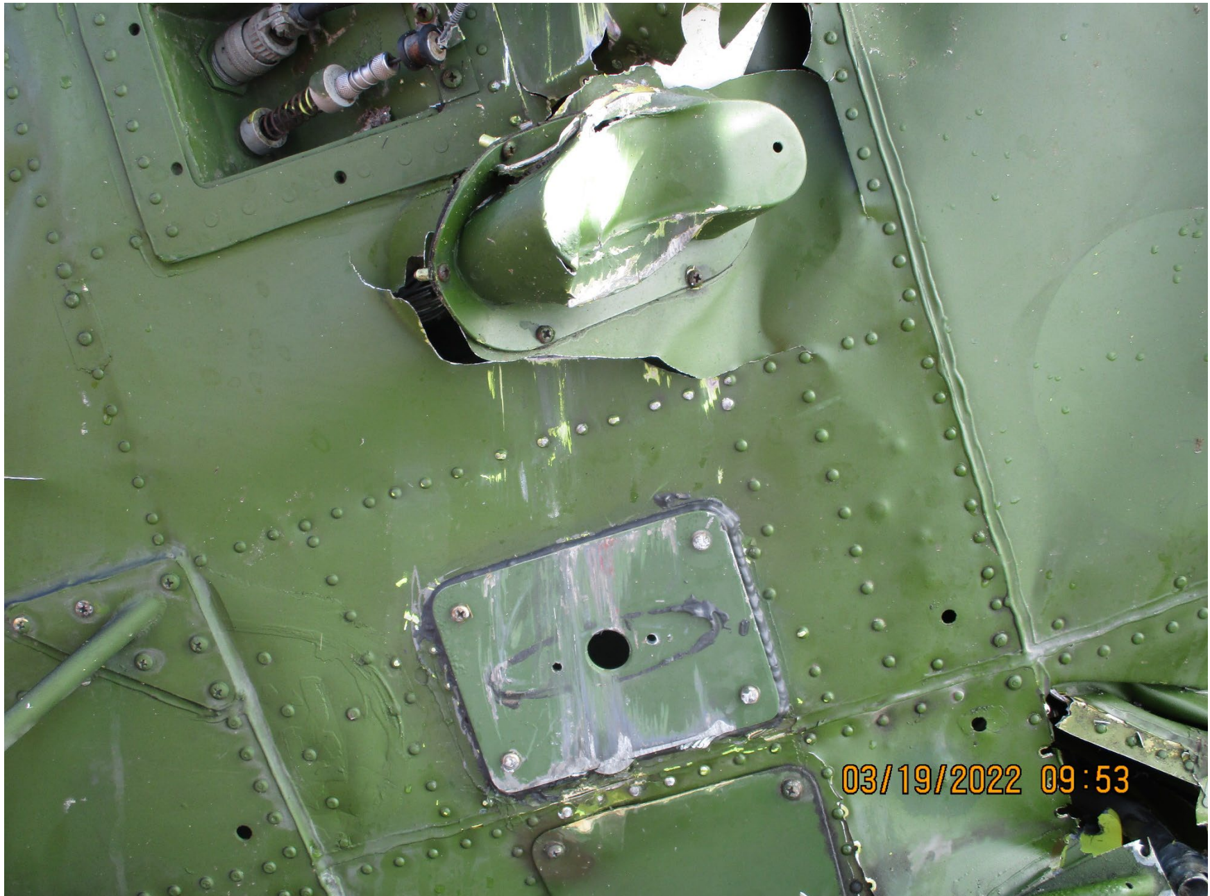
Photo 6 – Powerline impression mark on bottom of helicopter
