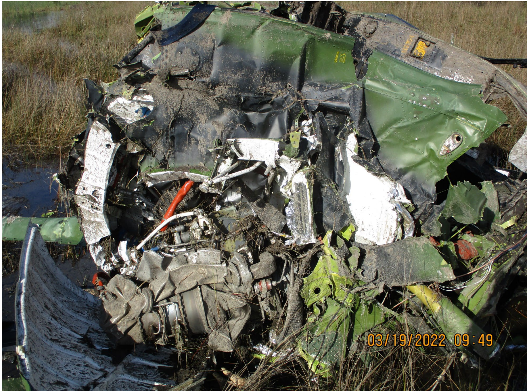
Photo 4 – Main wreckage, engine
