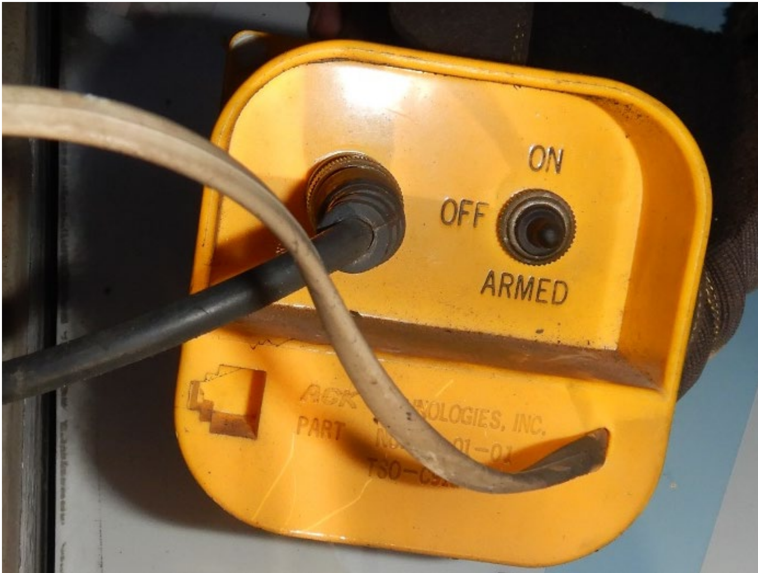
Photo 16 – ELT with Switch in “OFF” Position (As Found)
