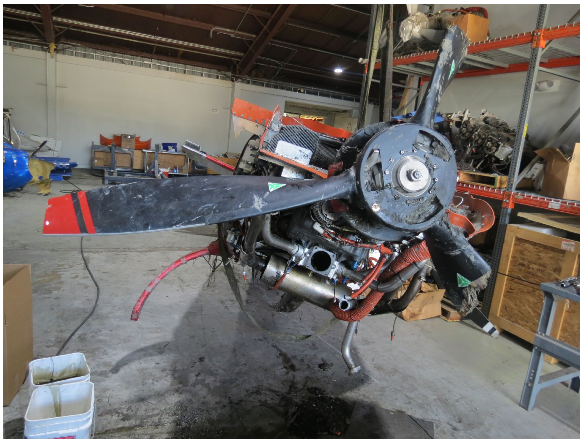
Photograph 9 - View of the remaining propeller blade and two partial blades. (Courtesy of Lycoming)
