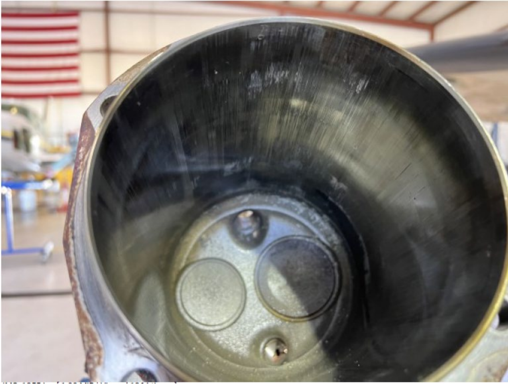
IMG_1255.jpg. View of the Damaged #1 Cylinder. Note the damage to the heads of the intake and exhaust valve and the same damage to the upper portion of the cylinder.
