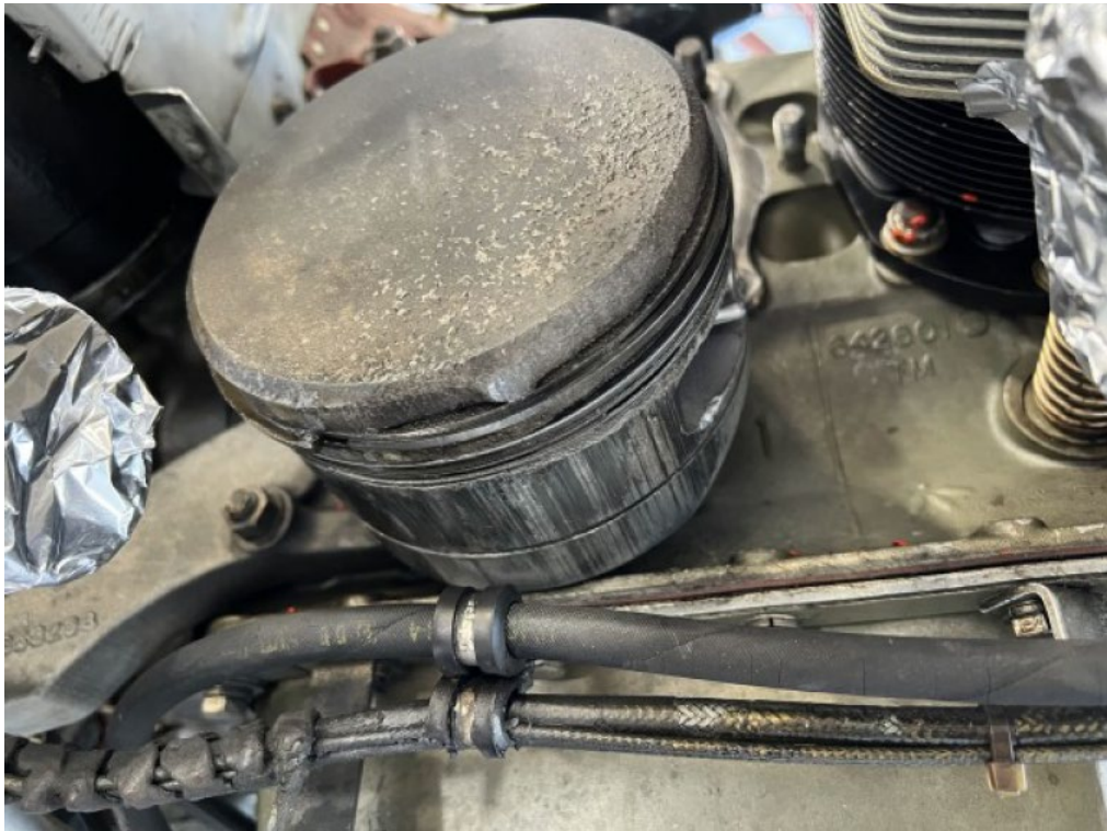
IMG_1253.jpg. View of the Damaged #1 Piston.
