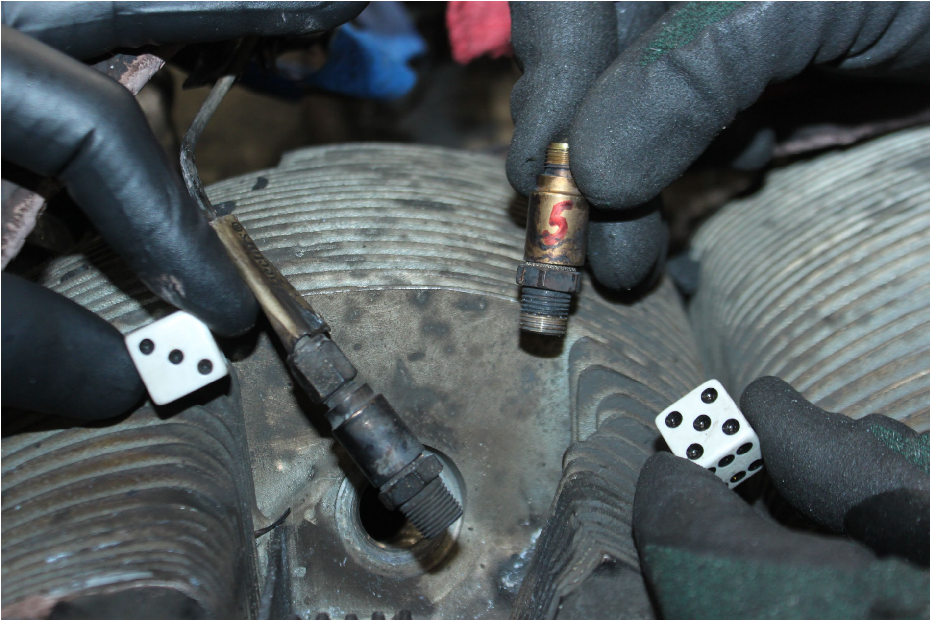
Photo 10 – NTSB Digital Photograph. View Showing the Nos. 3 and 5 Fuel Injector Nozzles of the Left Engine. Note the Completely Sooted Threads of the No. 3 Nozzle and the Clean and Sooted Line of the Threads of the No. 5 Nozzle.
