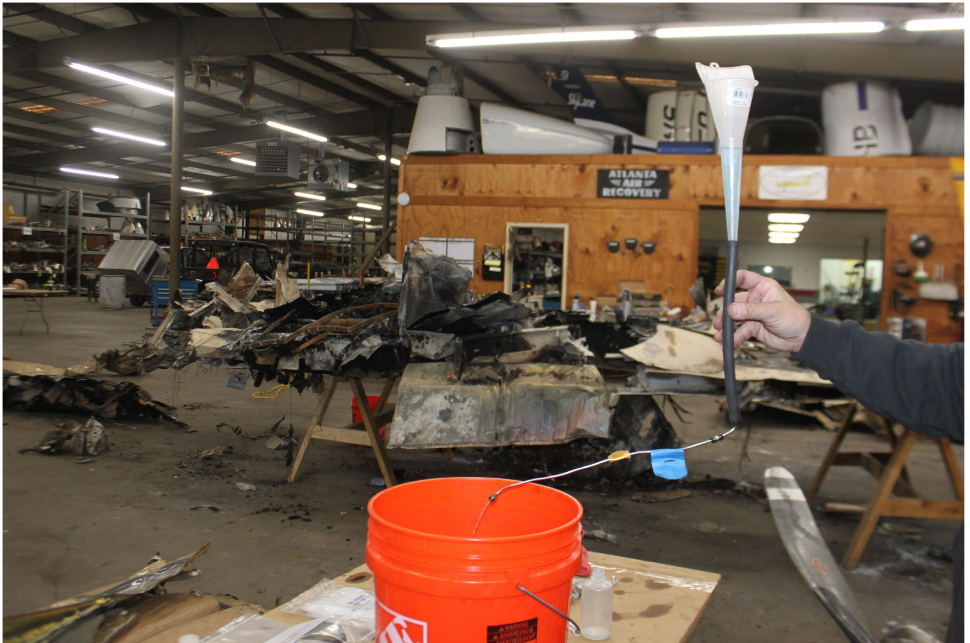
Photo 15 – NTSB Digital Photograph. View Showing the Flow Testing of the No. 1 Cylinder Fuel Injector Line of the Right Engine.
