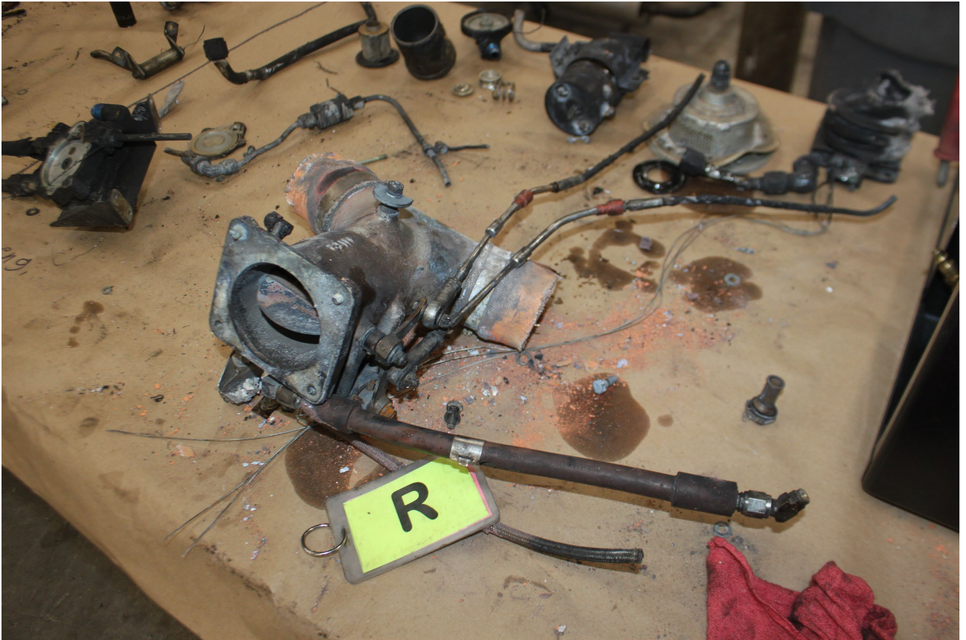
Photo 16 – NTSB Digital Photograph. View of the Right Throttle Body and Metering Valve. Note the Extensive Heat Damage.
