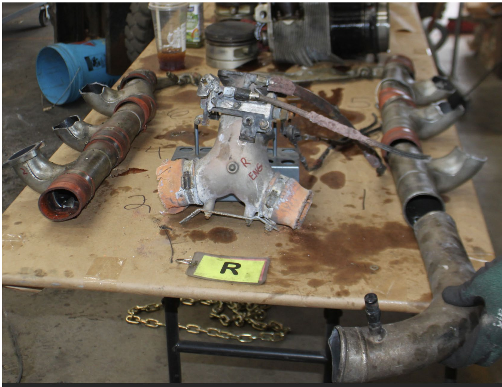
Photo 17 – NTSB Cropped Digital Photograph. View of the Layout of the Right Engine Air Induction and Throttle Body and Fuel Metering Valve. The No. 1 Cylinder Is On the Lower Right Portion of the Photograph.
