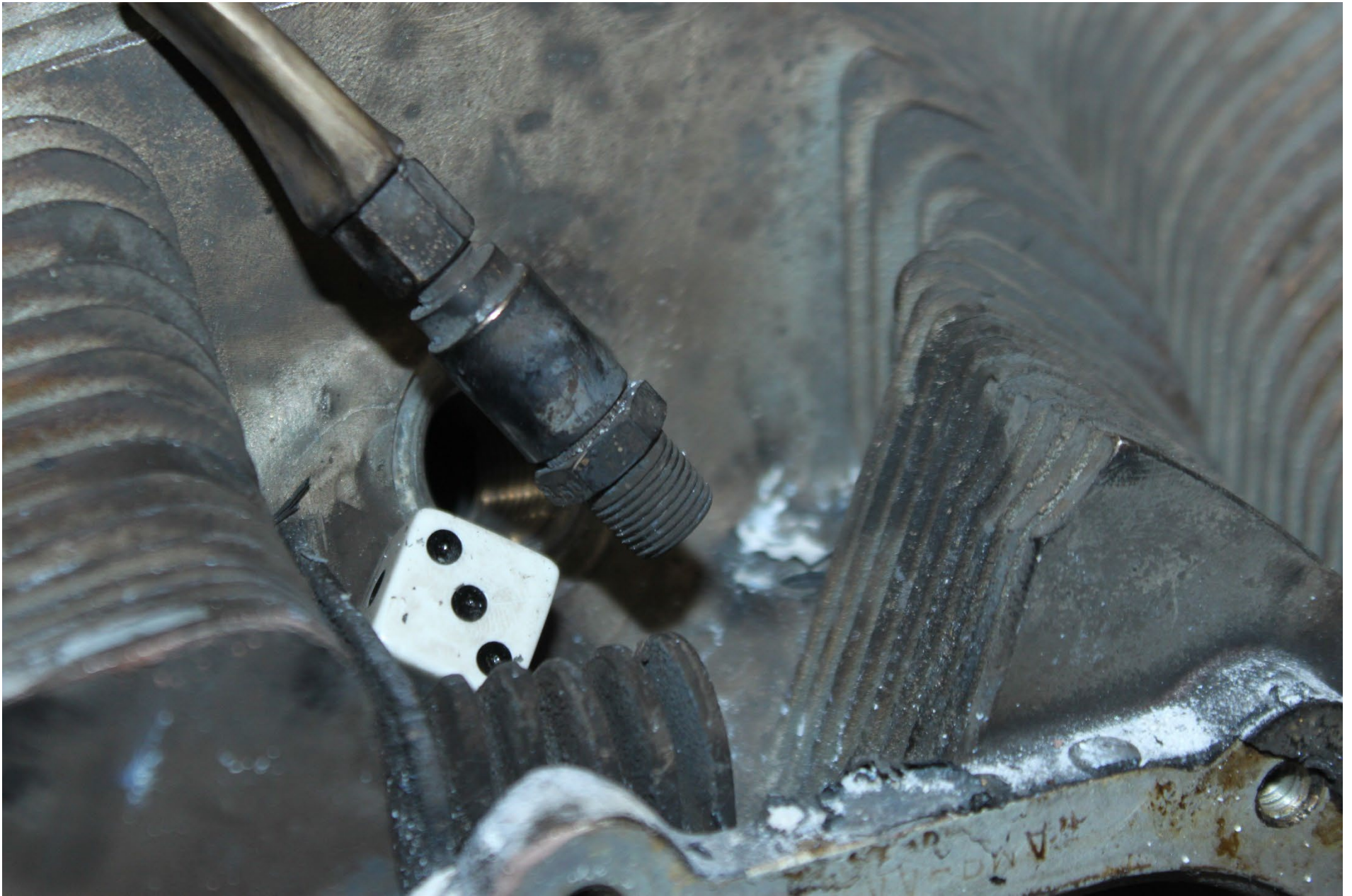
Photo 9 – NTSB Digital Photograph. View of the No. 3 Cylinder Fuel Injector Nozzle of the Left Engine As Found Not Installed in the Cylinder. Note the soot Along the Length of the Threads.
