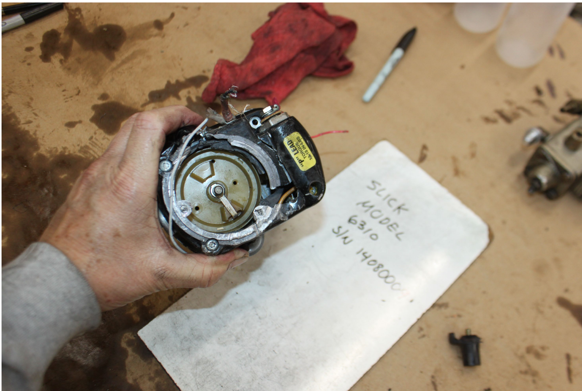
Photo 14 – NTSB Digital Photograph. View up the Aft Portion of the Impact Separated Right Magneto of the Right Engine Showing the Impact Separated Distributor Block and Cover.
