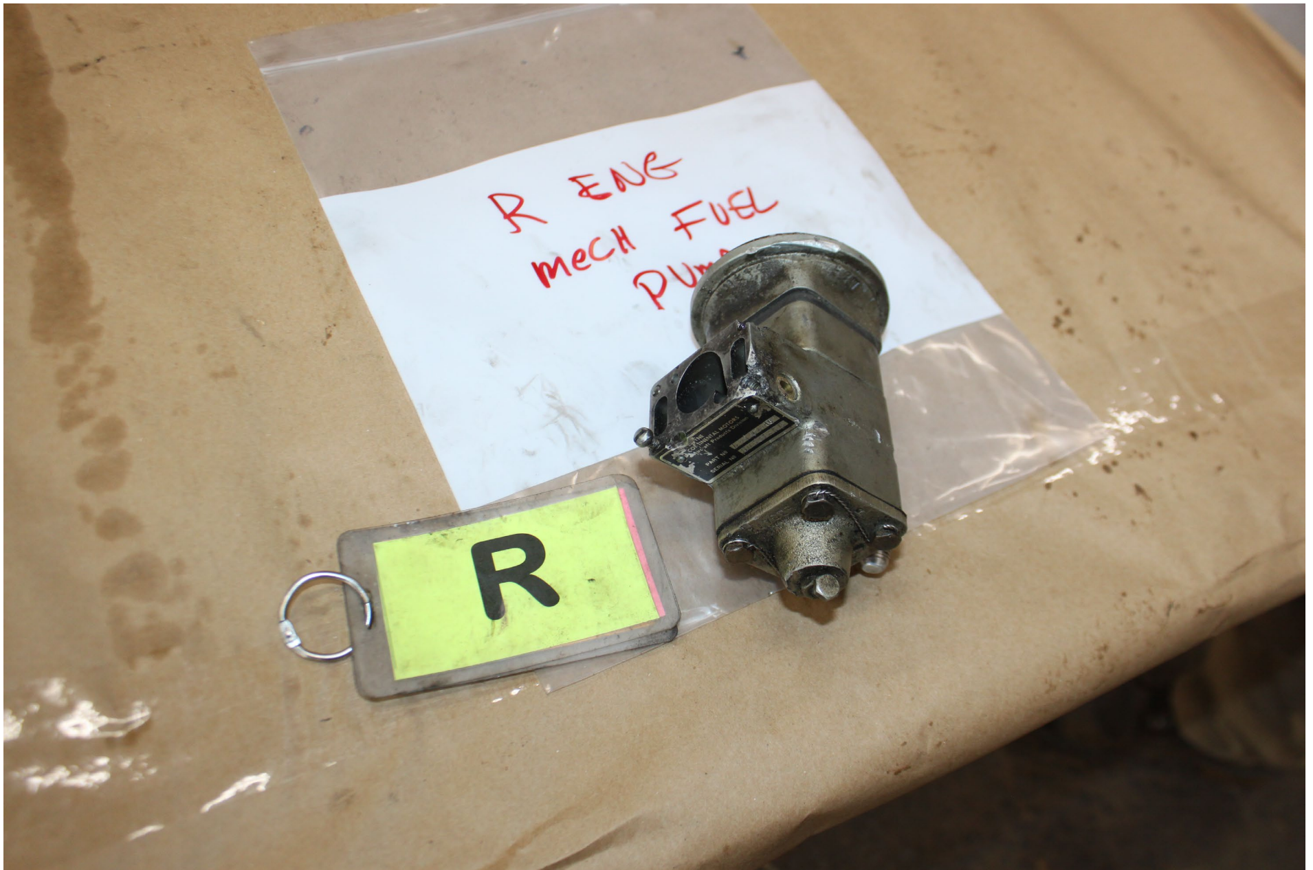
Photo 18 – NTSB Digital Photograph. View of the Impact Separated Right Engine-Driven Fuel Pump.
