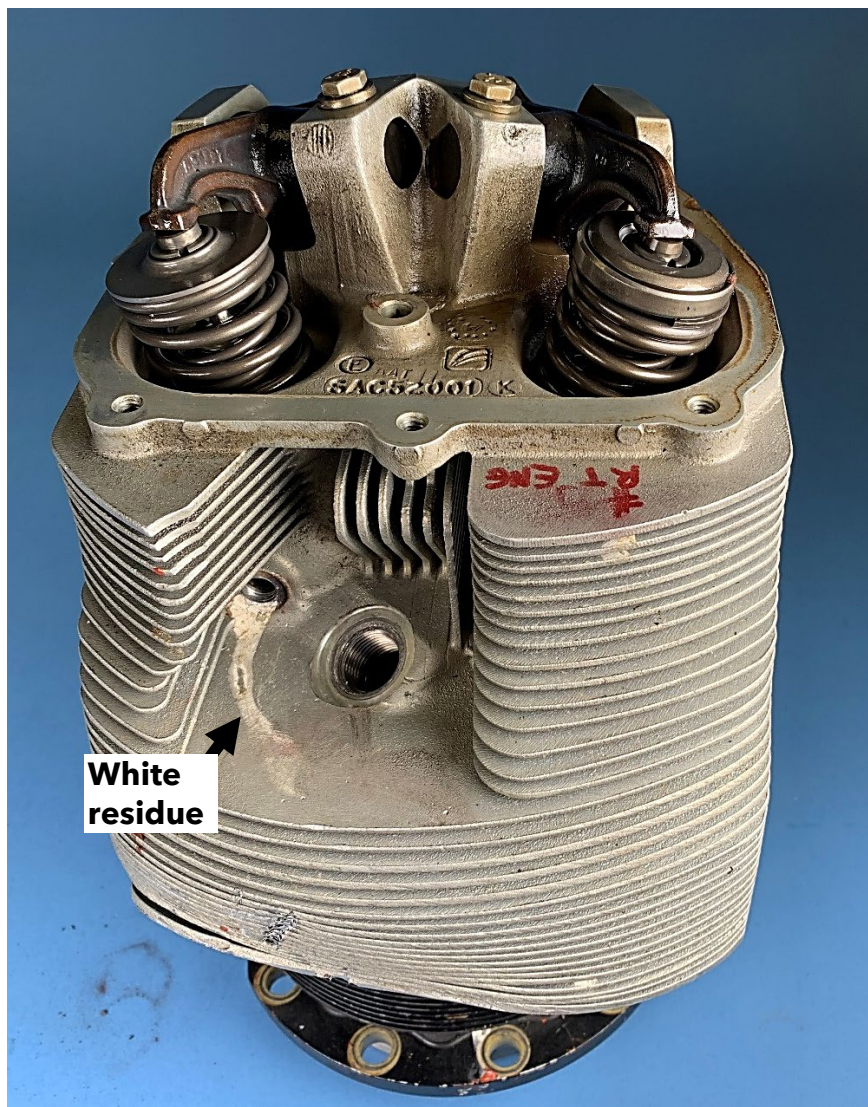
Figure 5. View of the #5 cylinder showing white residue at the entry port for the injector nozzle.
