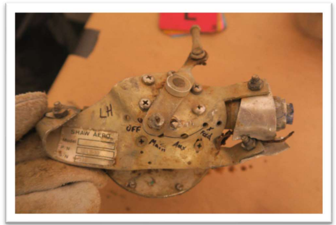
Photo 2 - Left fuel selector valve
