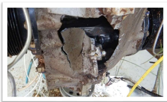
Photo 10 - Damage of forward crankcase
