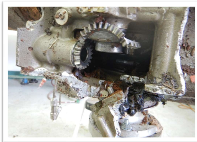
Photo 19 - Front camshaft drive gear impact damage
