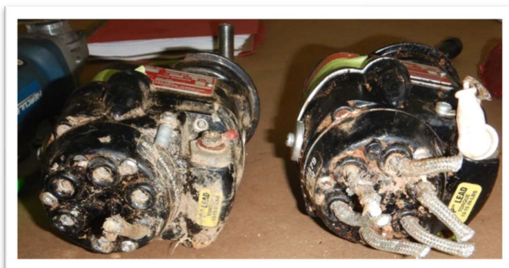
Photo 13 - Left engine magnetos before testing
