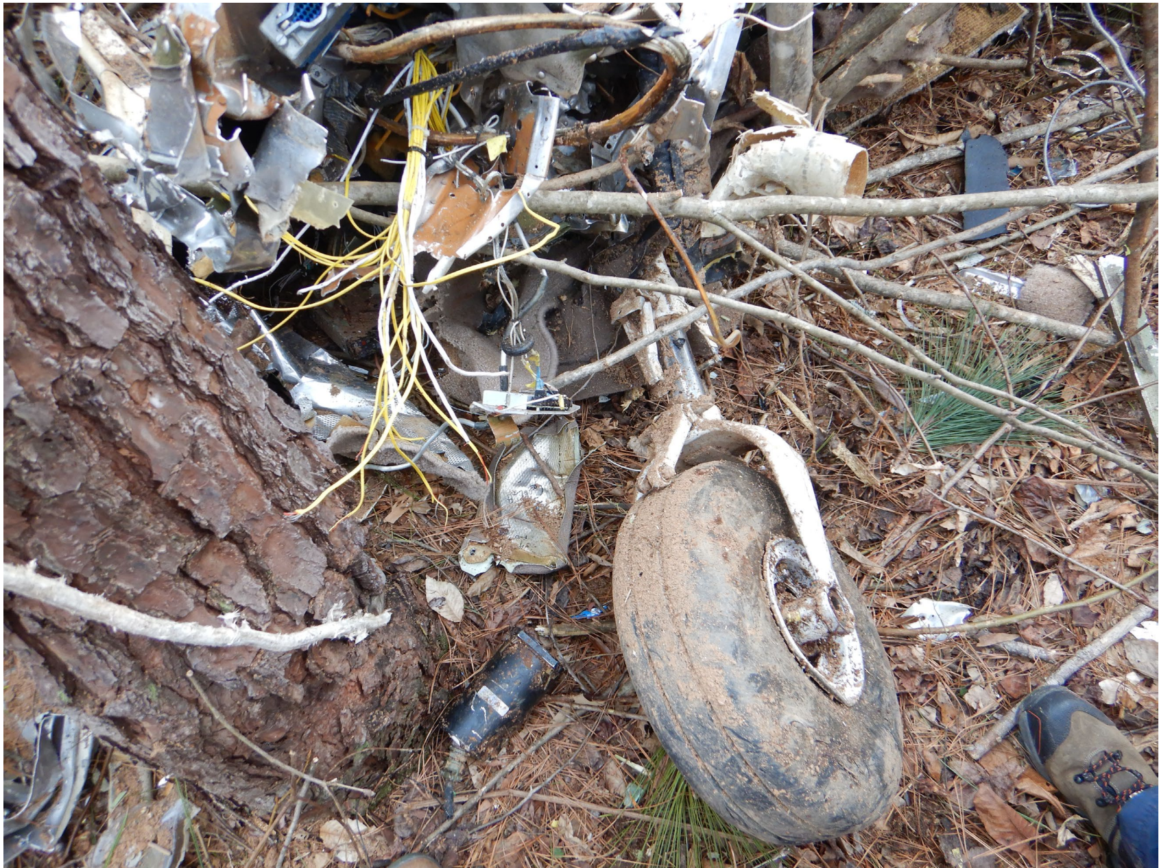
Photo 15 – View of nose landing gear near remnants of cockpit
