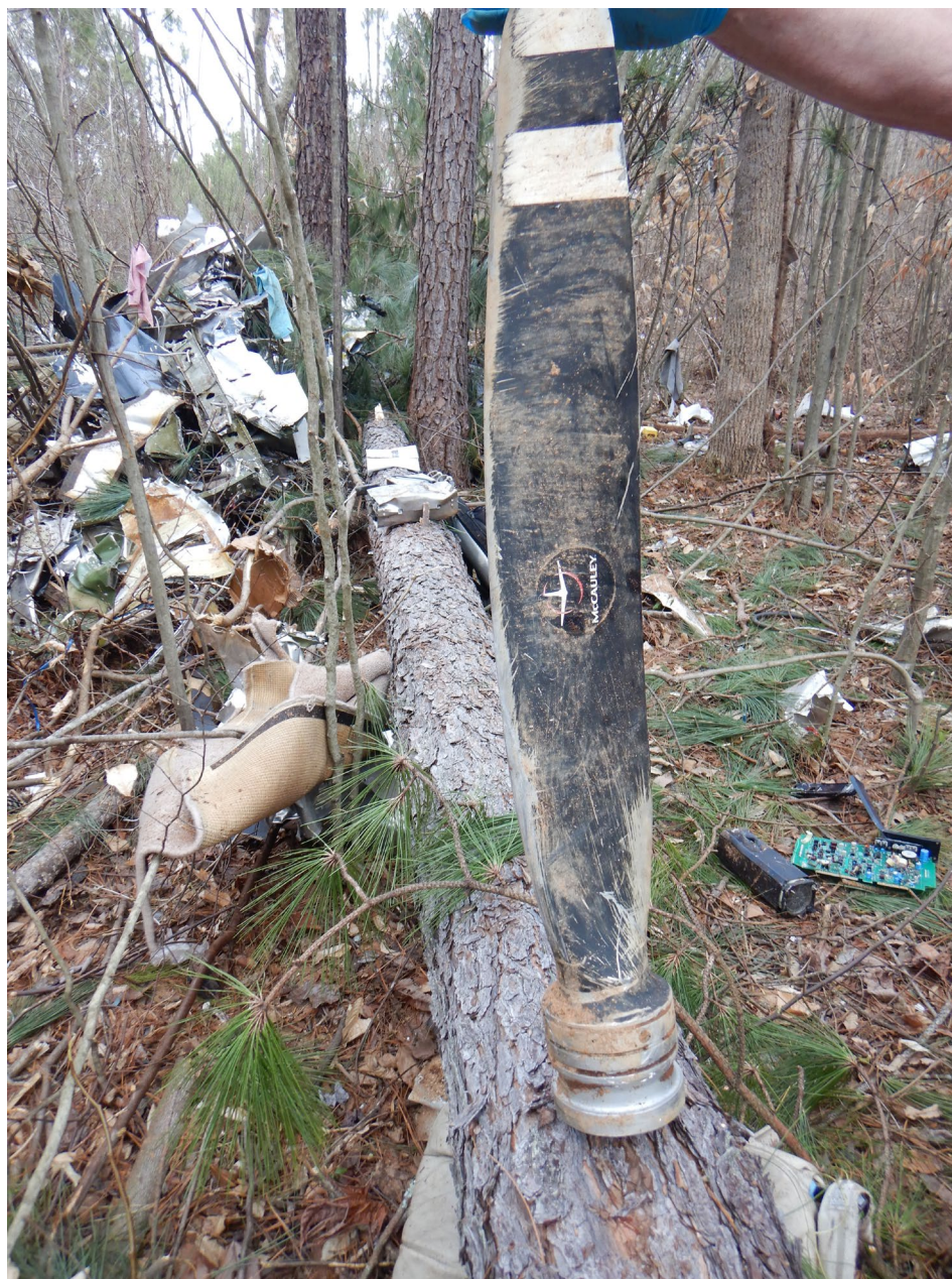
Photo 17 – View of propeller blade separated from hub with chordwise abrasion on face
