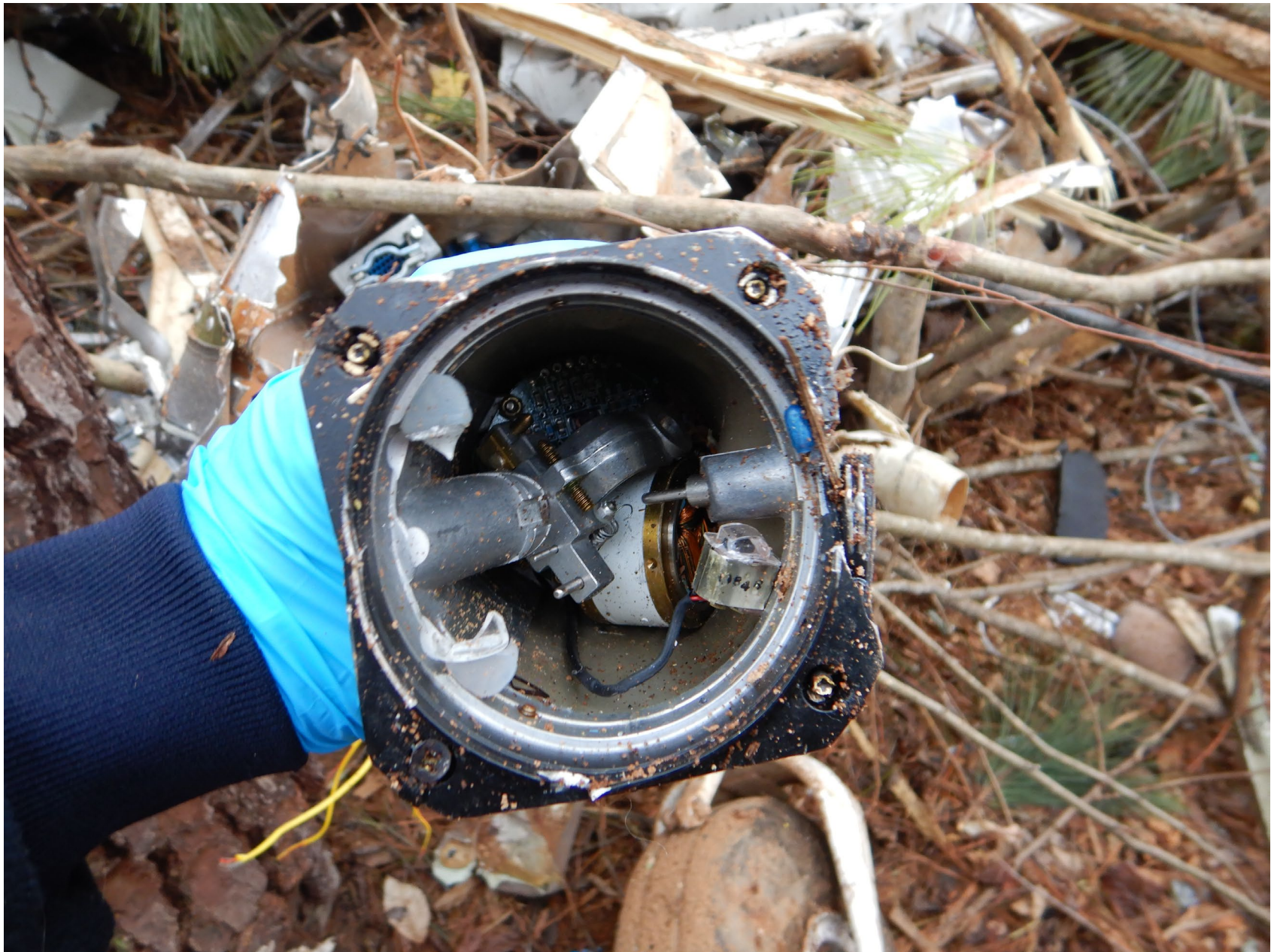
Photo 16 – Housing of gyroscopic instrument separated from cockpit control panel
