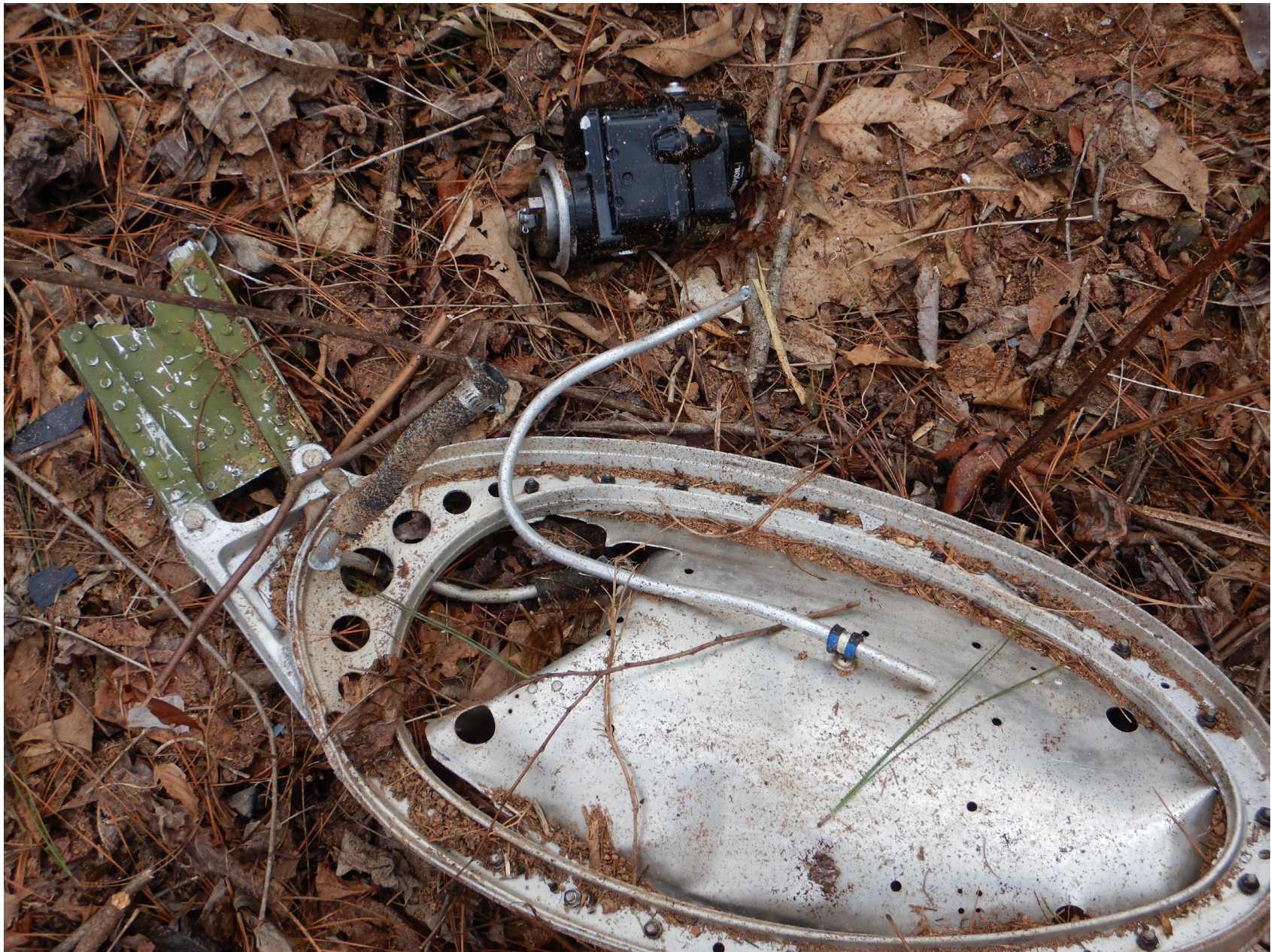
Photo 11 – View of fractured magneto and wreckage
