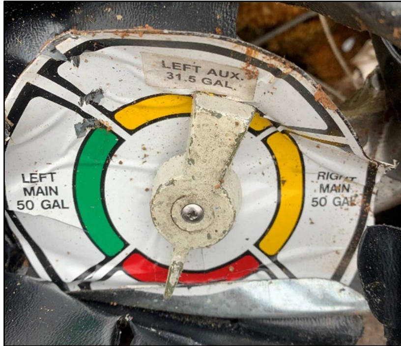
Figure 6: Left Engine Fuel Selector set to "LEFT ENGINE OFF"
