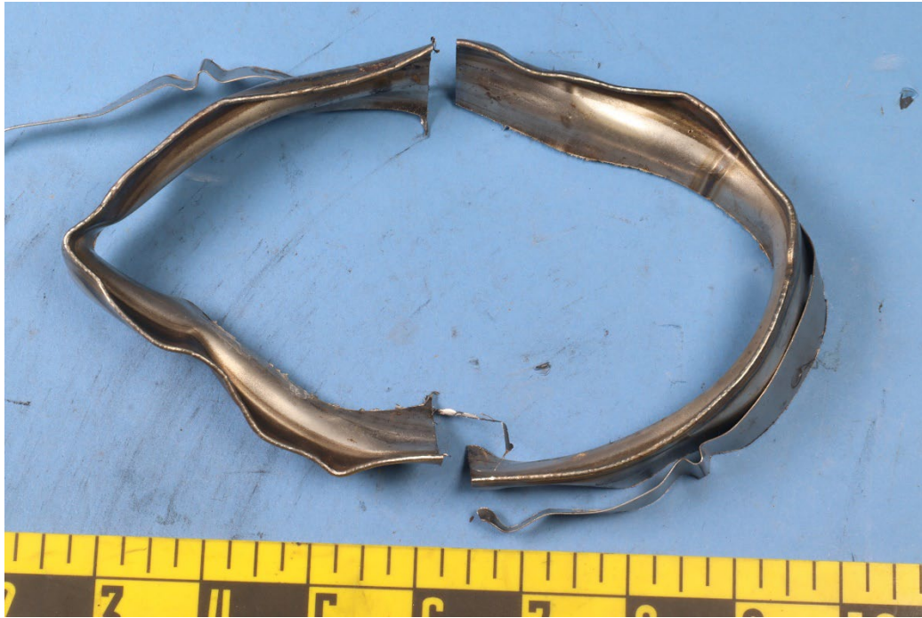
Figure 9: Weld seam of the outer hot section layers.
