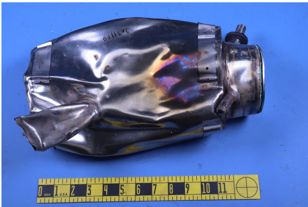
Figure 4: Exterior surface of outer hot section.
