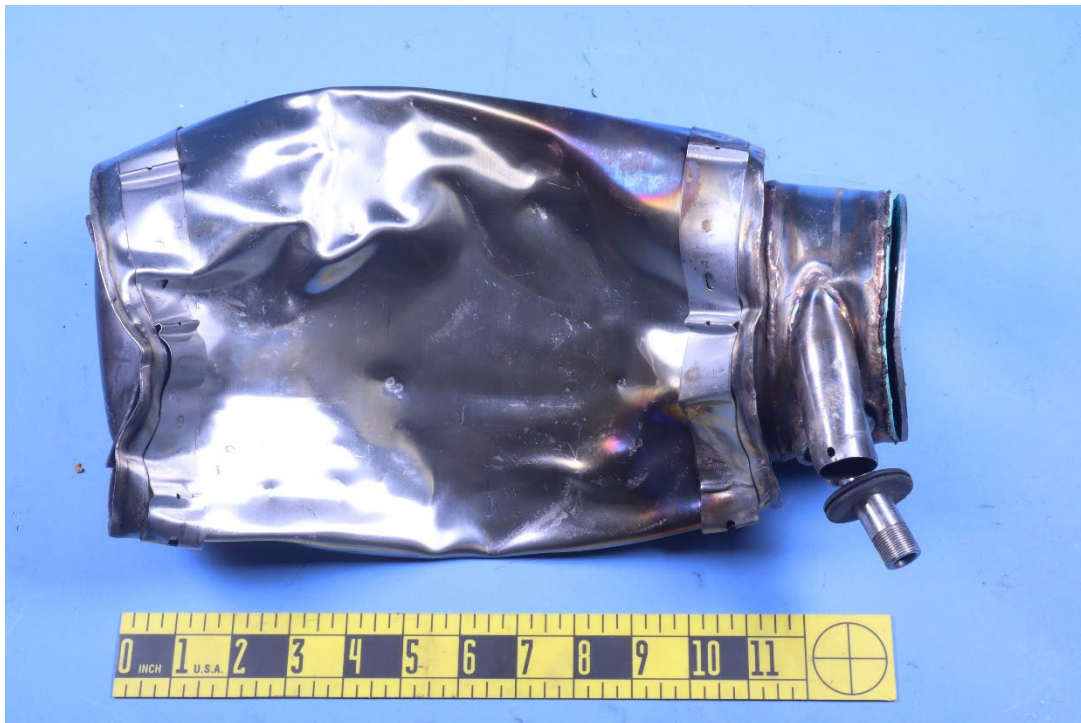
Figure 3: Exterior surface of outer hot section.
