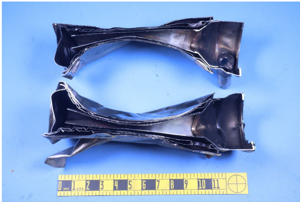
Figure 5: Heat exchanger and combustor assembly sectioned.
