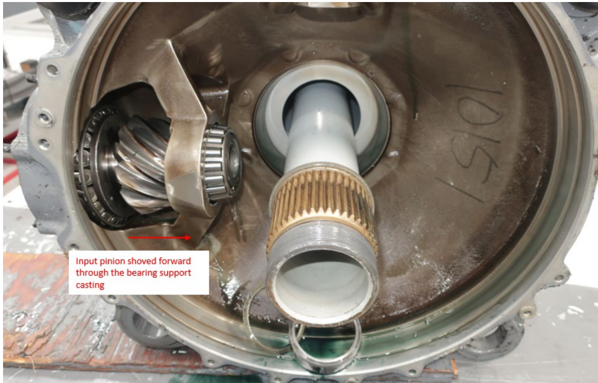
Photo 3 - Input pinion, support casting, and main rotor drive shaft.
