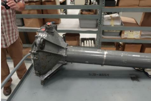
Photo 1 - Main gear box with mast tube attached.
