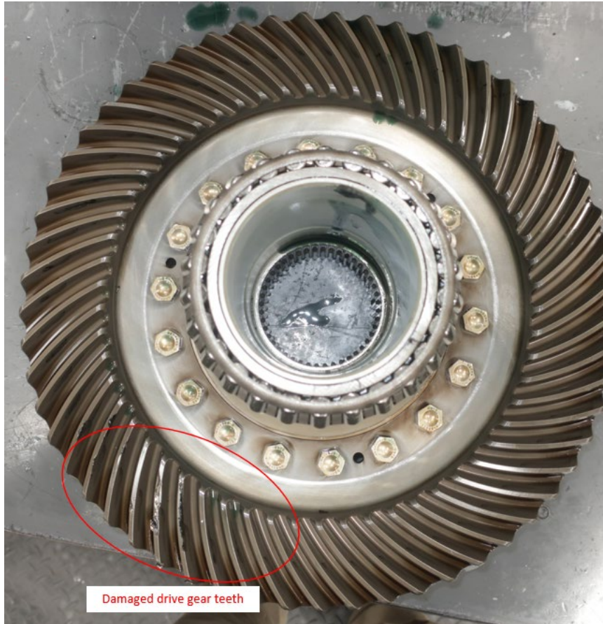
Photo 5 - Area of damaged ring gear teeth.
