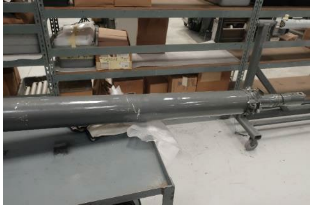
Photo 2- Mast tube with drive shaft extended out the top.
