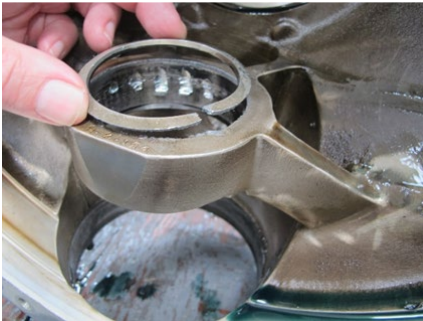
Photo 4 - Input pinion support casting showing cast retaining flange separation.
