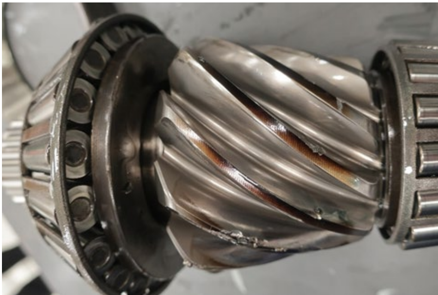
Photo 6 - Damaged input pinion teeth.
