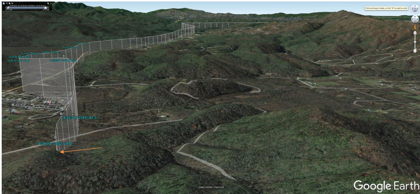
Figure 22. The helicopter's groundtrack created from the GoPro's metadata. This figure shows the last recorded points leading up to the impact with terrain. An arrow has been added to show the vicinity of the wreckage.
