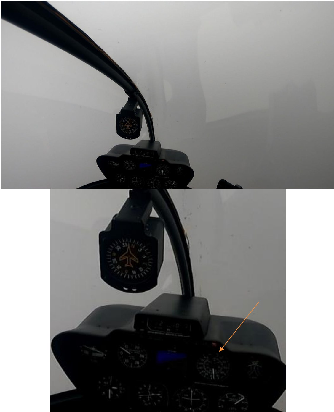
Figure 17. A screenshot of the GoPro recording at 2:25:20. An arrow points to the low rotor RPM warning light.
