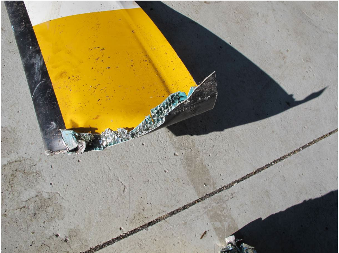
Above and below: Disconnect surfaces of main rotor blade serial number 12227.
