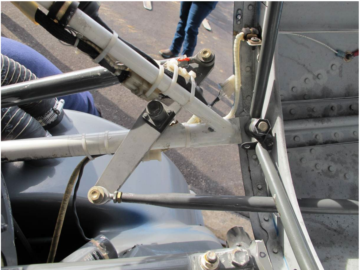
Forward end of C121-17 push pull tube.
