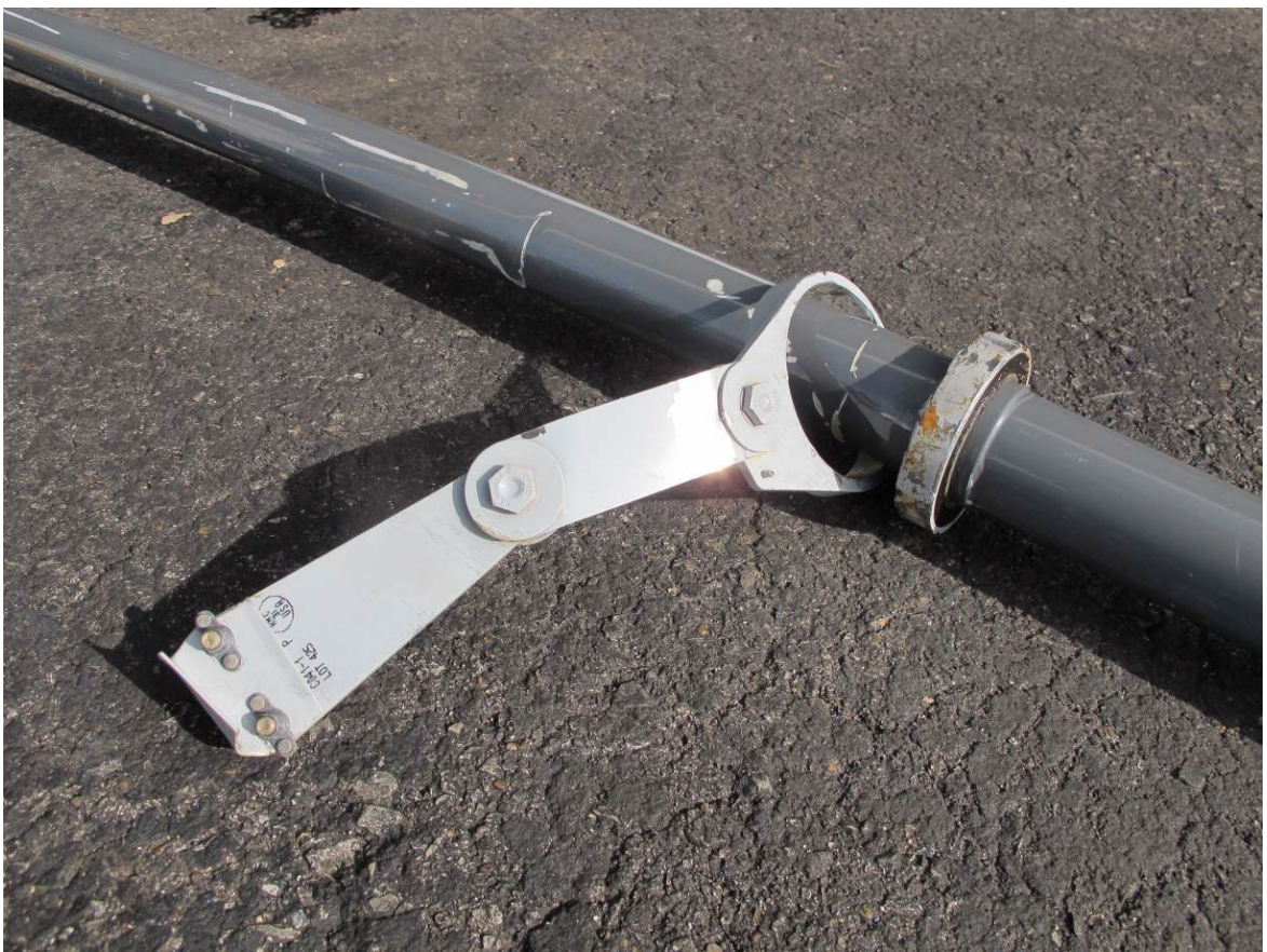
Tail rotor driveshaft damper bearing and hanger support.
