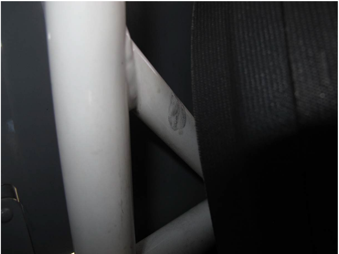
Rubber transfer on left side of upper frame.
