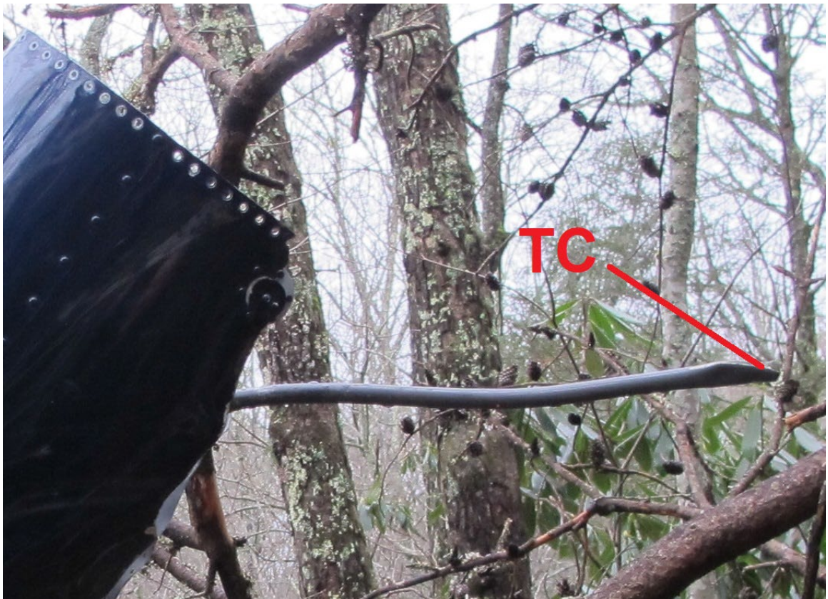
Disconnect TC in forward section of C121-17 push pull tube.
