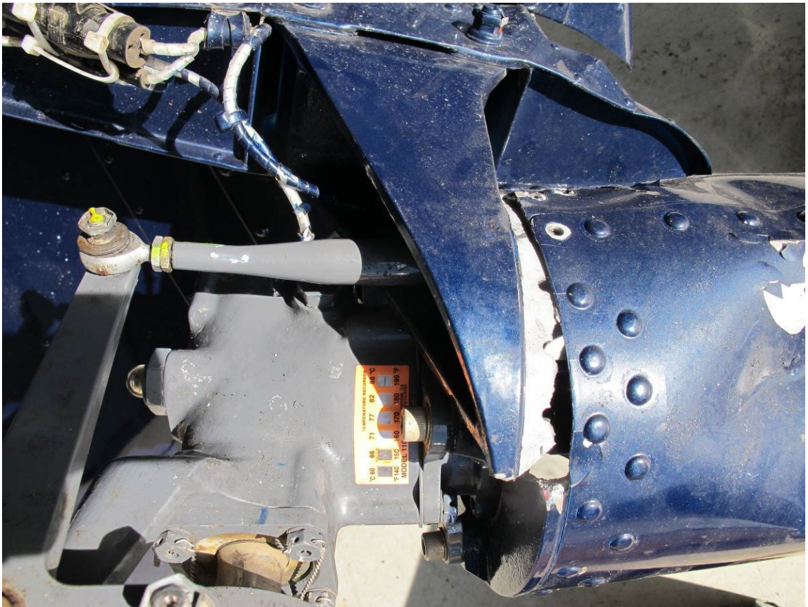
Separation between tailcone bay 7 and aft bulkhead casting.
