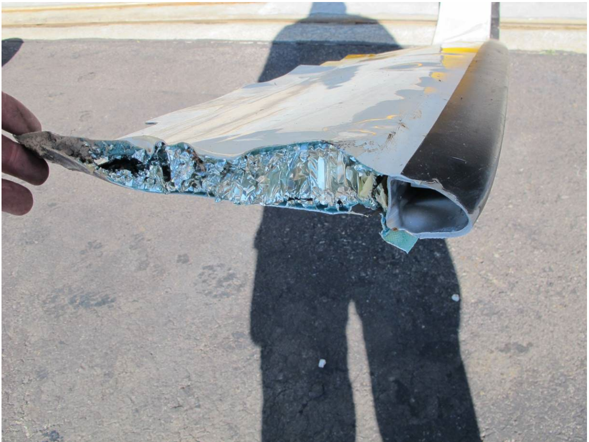
Above and below: Disconnect surfaces of main rotor blade serial number 12234.
