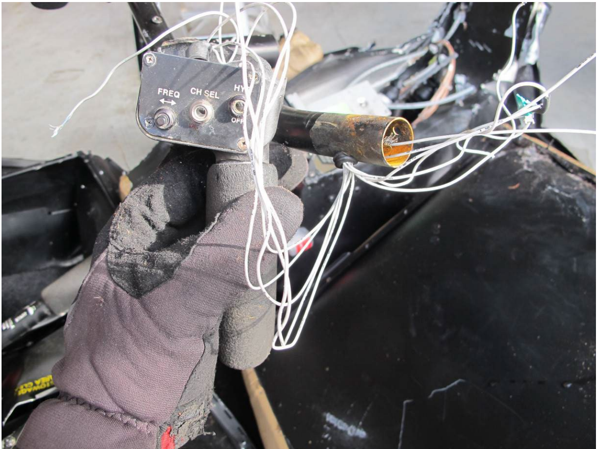
Above and below: Disconnect A in pilot's cyclic grip.
