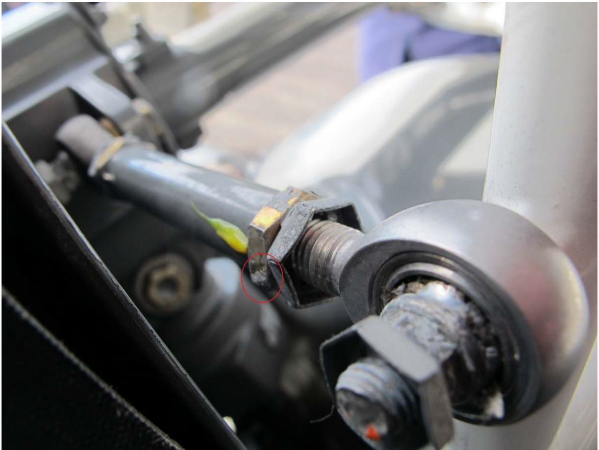
Paint transfer on jam nut of clutch centering strut.
