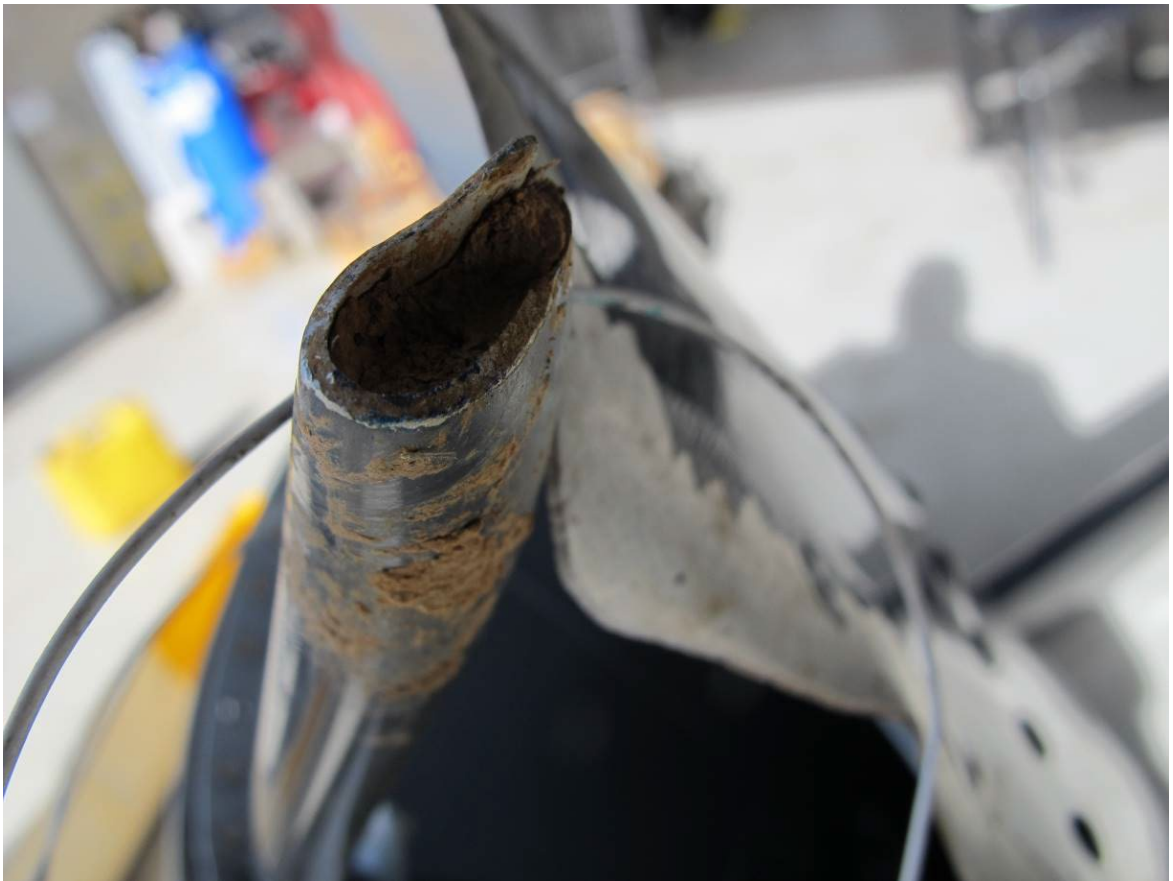
Disconnect TC in aft section of C121-17 push pull tube.
