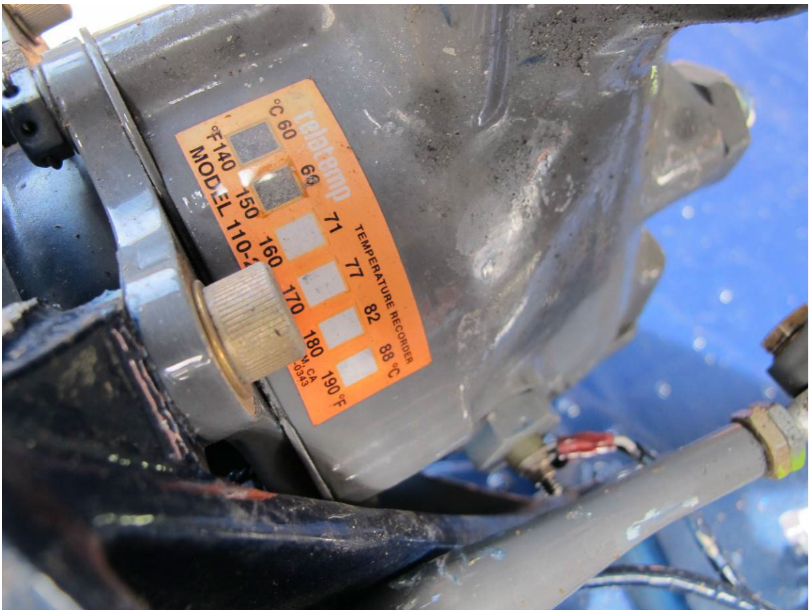
Tail rotor gearbox temperature sensor.
