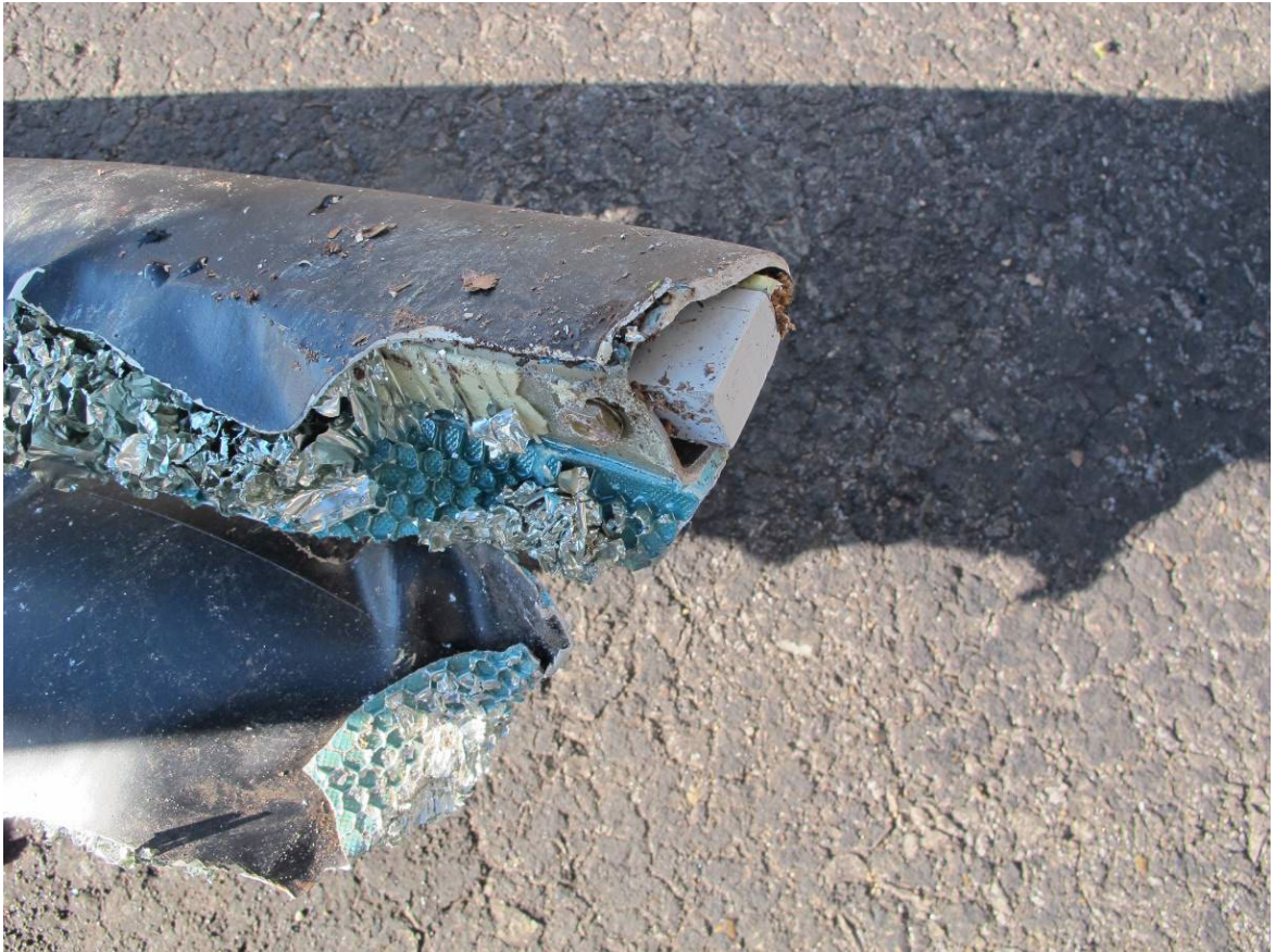
Above and below: Disconnect surfaces of main rotor blade serial number 12234.
