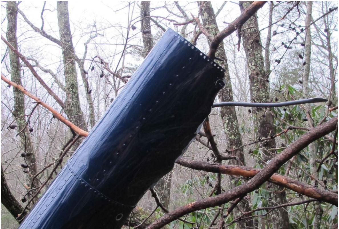
Separation between tailcone bays 5 and 6.
