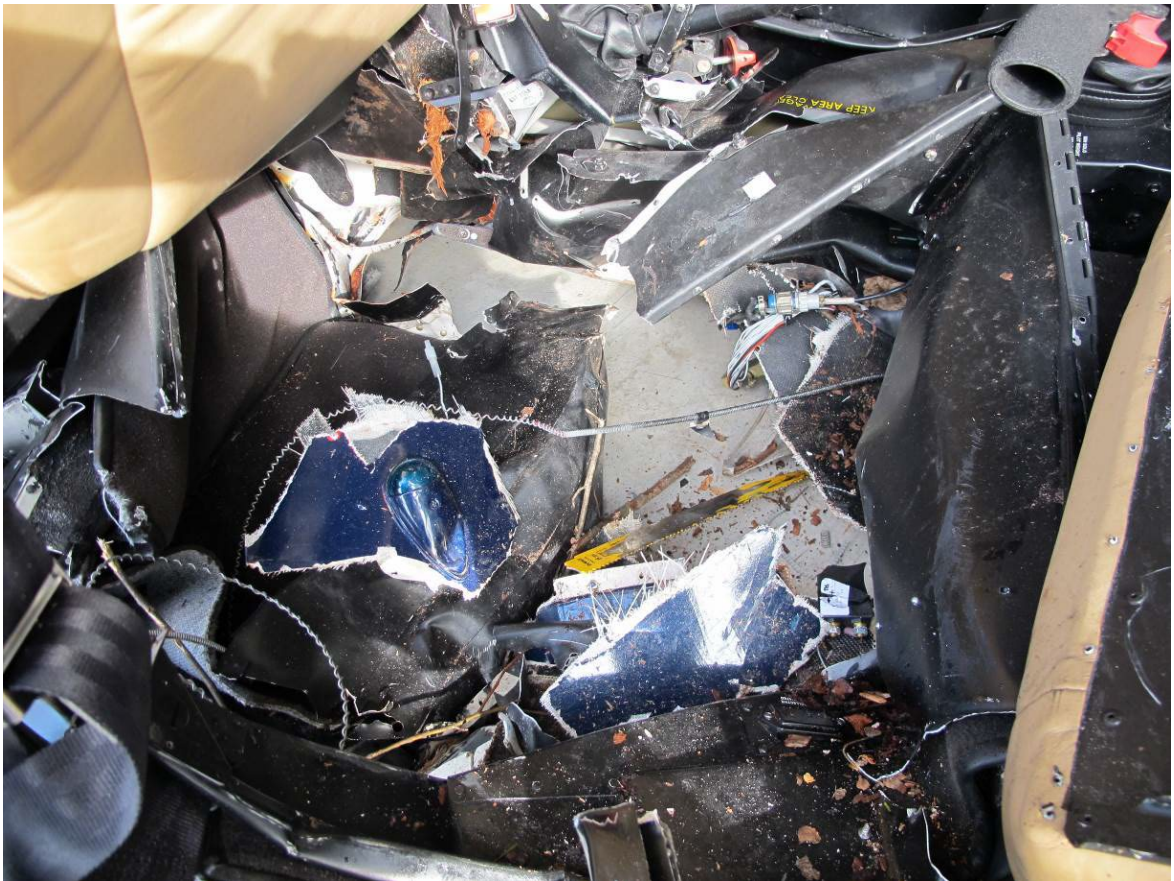
Fuel mixture control wire sheathing stretched.
