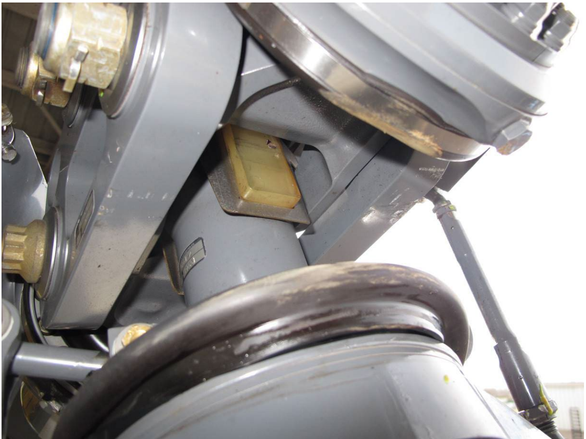
Elastomeric teeter stop for main rotor blade serial number 12227.
