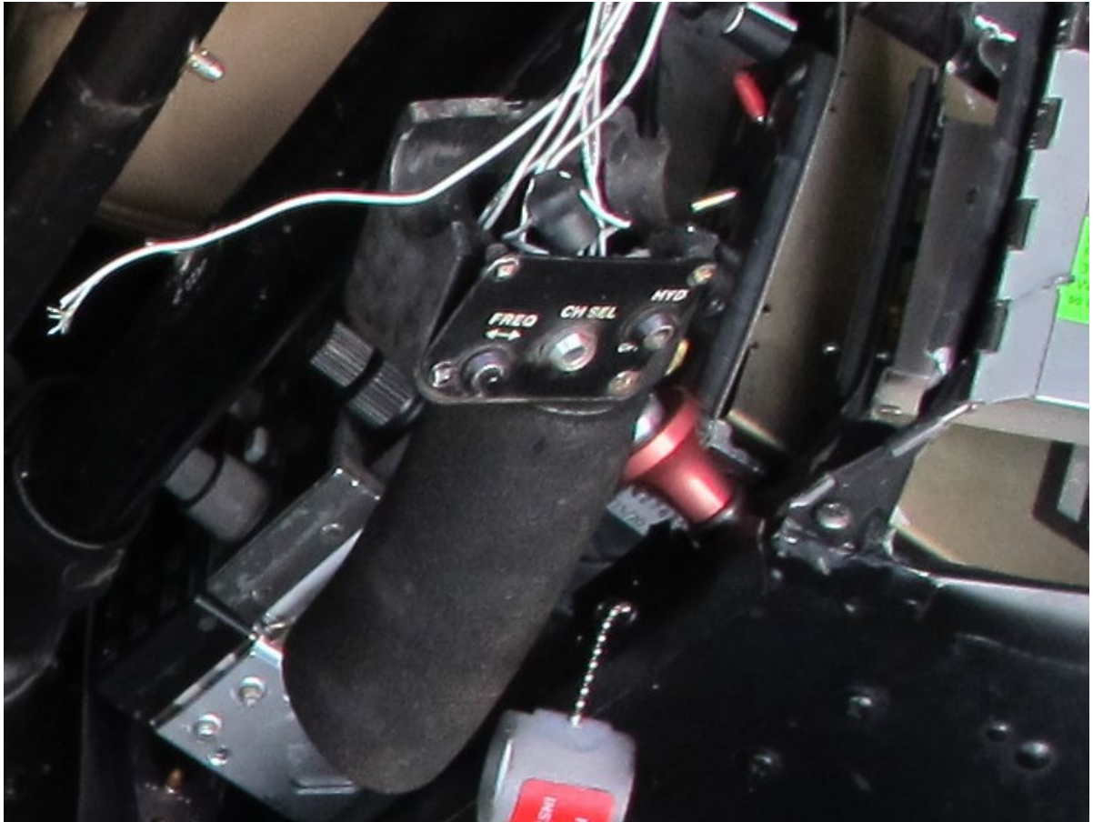
Above and below: Disconnect A in pilot's cyclic grip.
