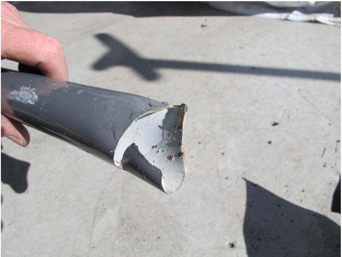
Disconnect surface on aft section of tail rotor driveshaft.
