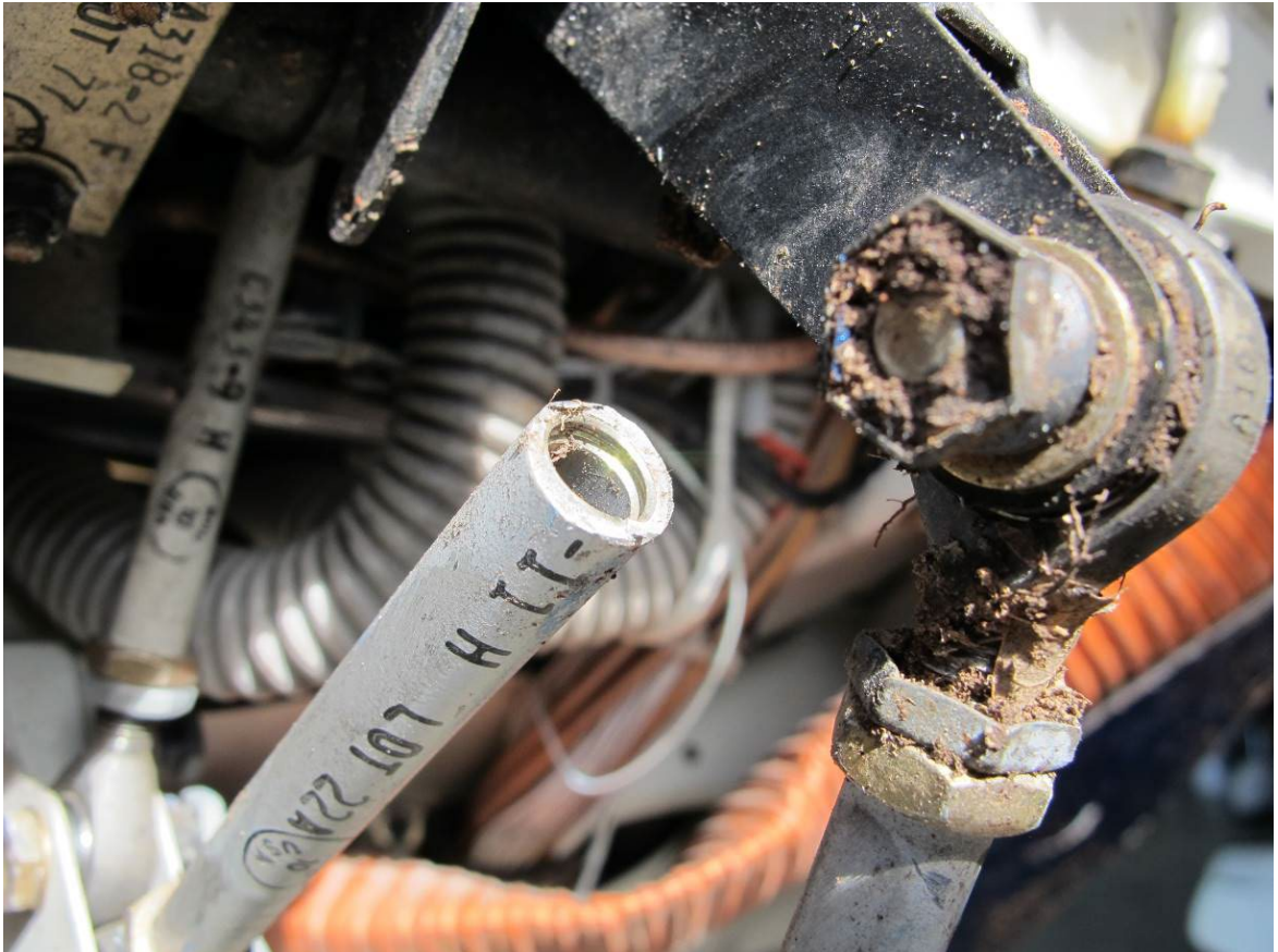
Above and below: Disconnect TA at forward end of C343-11 push pull tube.
