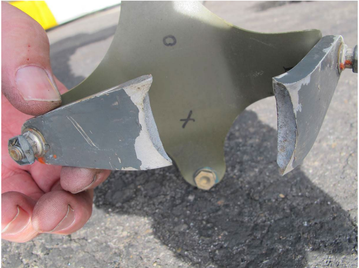
Above and below: Disconnect in intermediate flex coupling.
