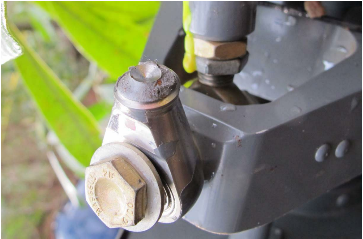
Disconnect C in lower rod end of C258-6 pitch link.
