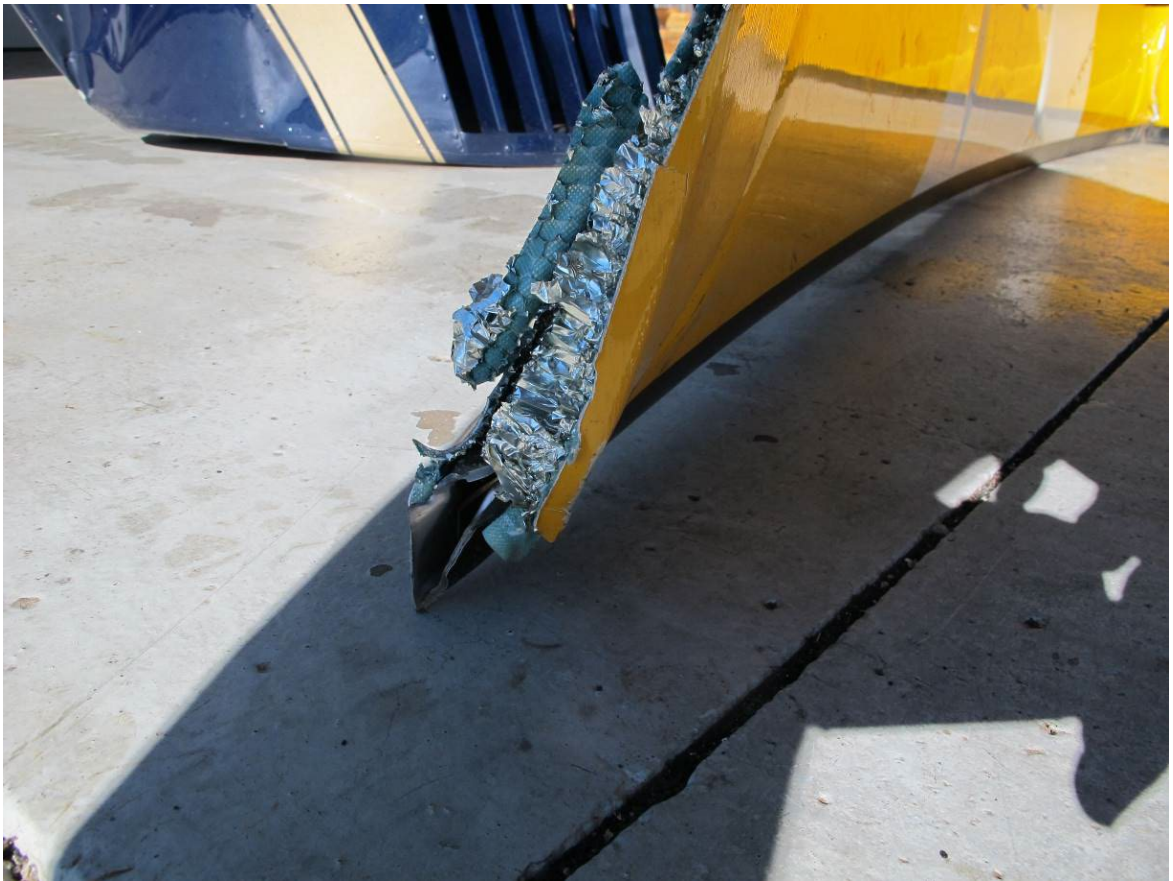
Above and below: Disconnect surfaces of main rotor blade serial number 12227.
