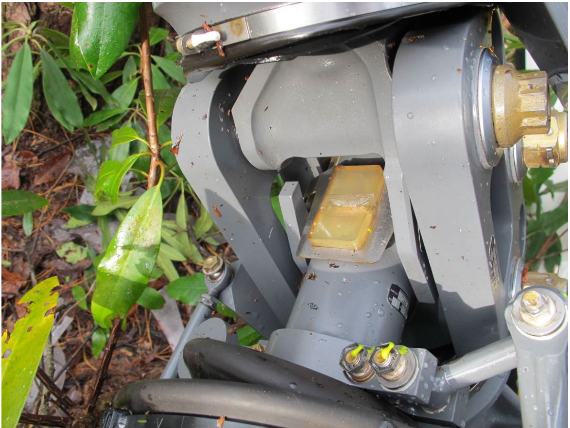
Elastomeric teeter stop for main rotor blade serial number 12234.
