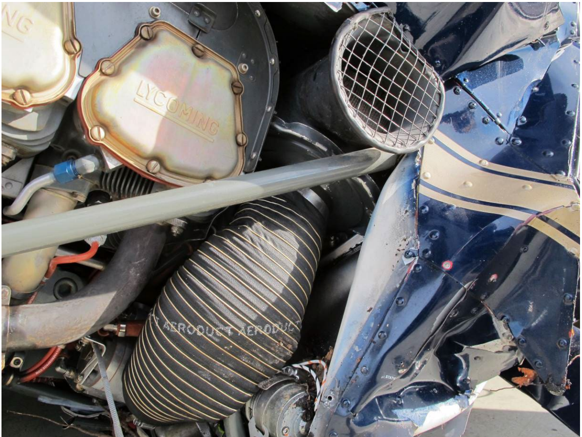
Intake screen and hose.
