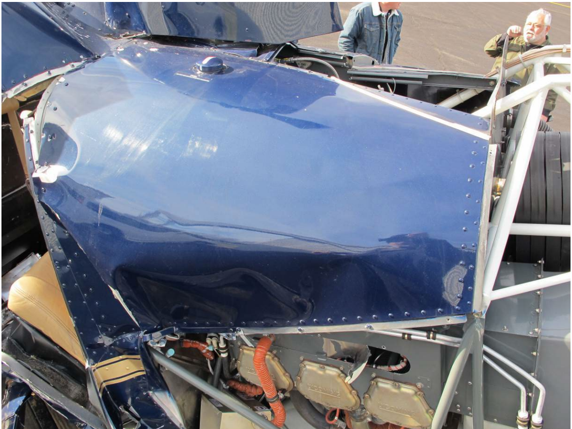
Main fuel tank.
