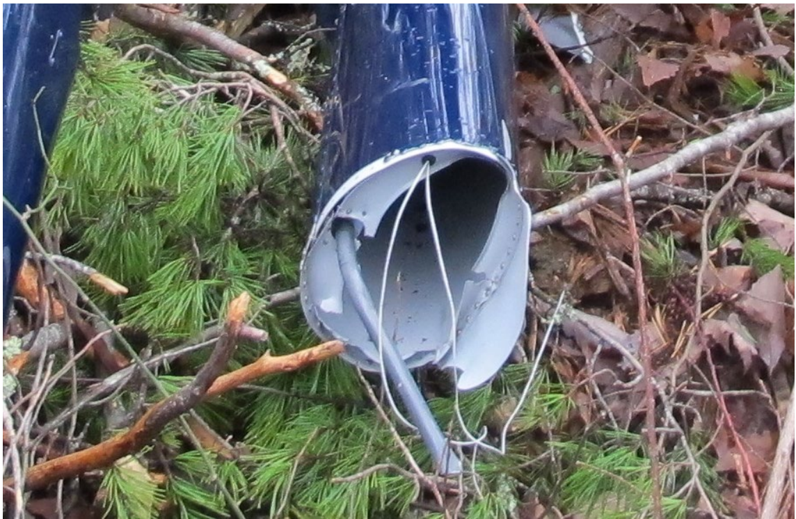
Separation between tailcone bays 6 and 7.
