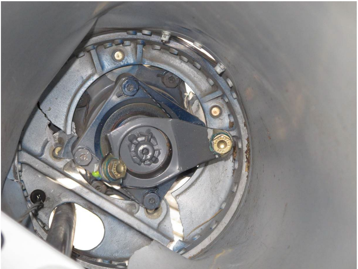
Tail rotor gearbox input yoke portion of aft flex coupling.
