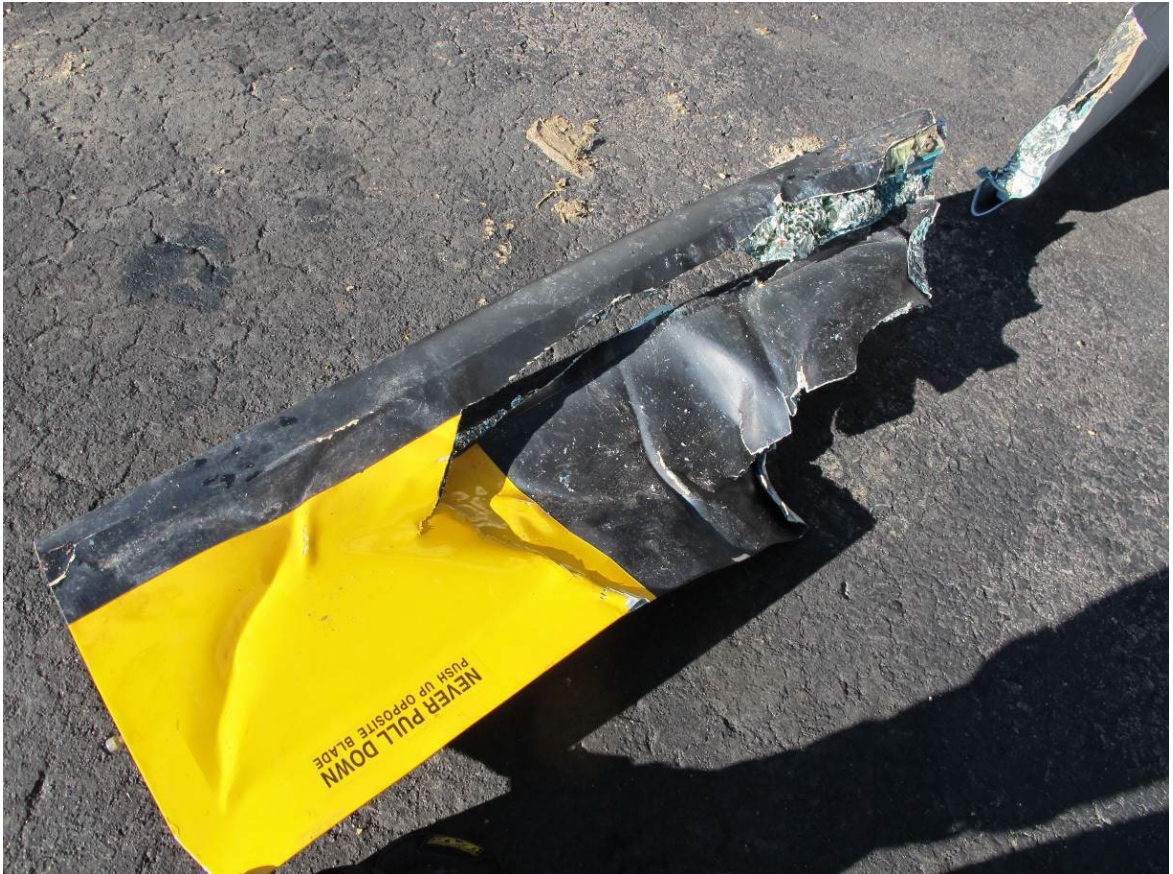
Above and below: Tip section of main rotor blade serial number 12234.
