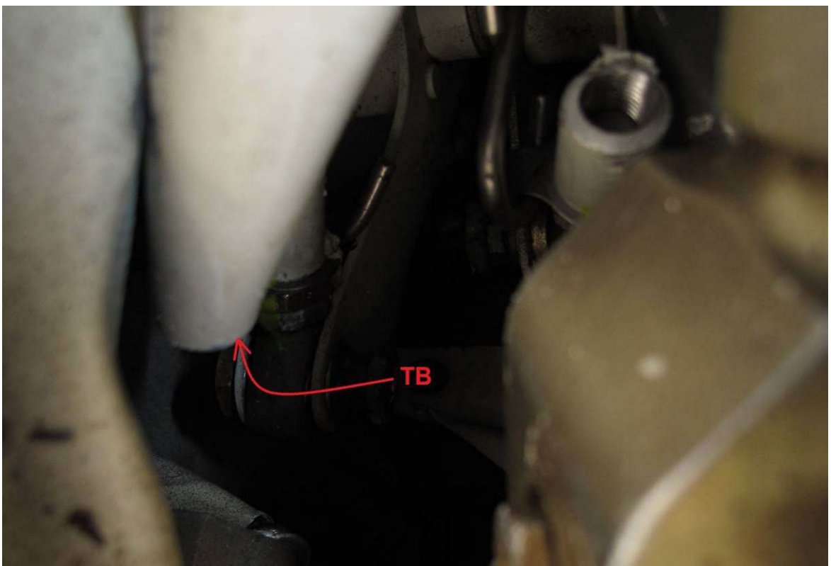
Above and below: Disconnect TB at aft end of C121-9 push pull tube.
