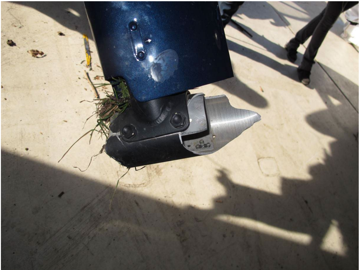
Disconnect in left skid at front strut.
