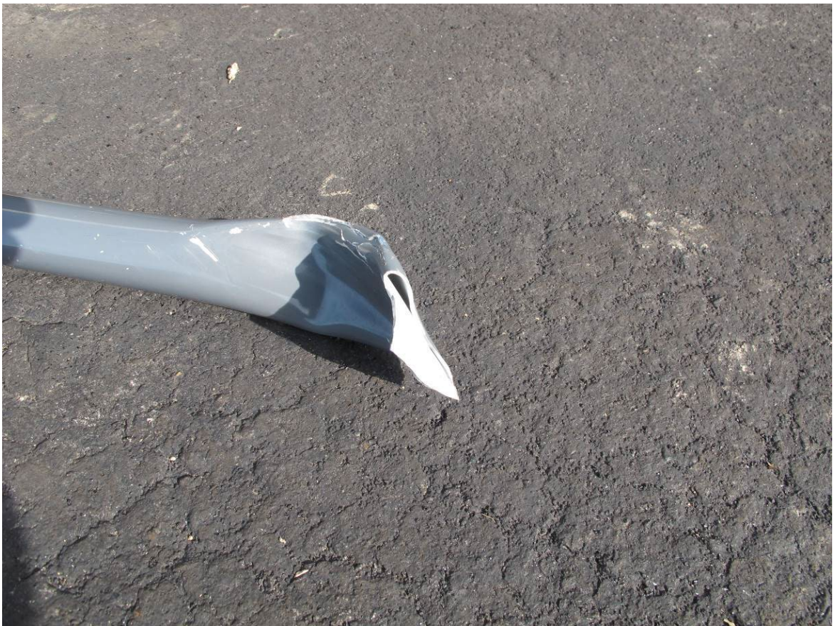
Disconnect surface on forward section of tail rotor driveshaft.
