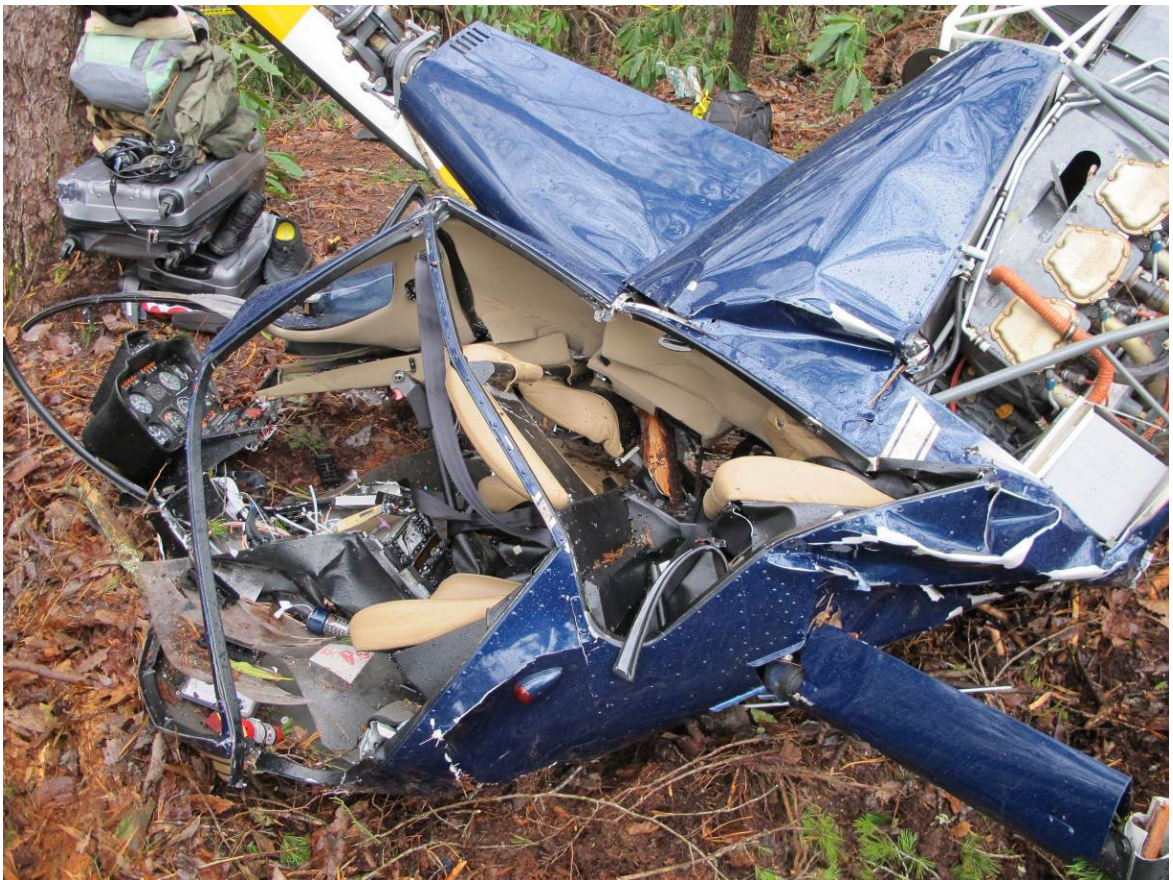
Left side door frame and cabin structure.
