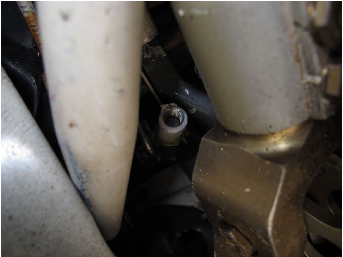
Disconnect B at aft end of C121-19 push pull tube.
