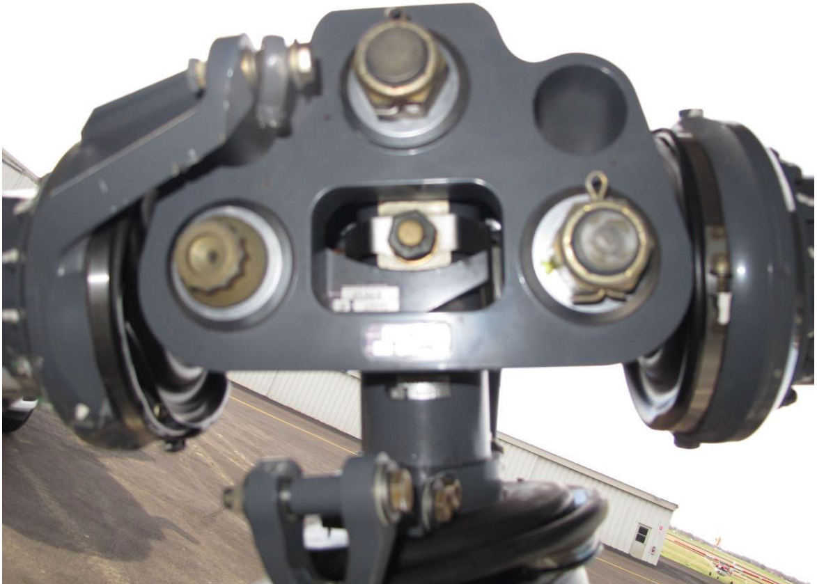
Droop stop for main rotor blade serial number 12234.
