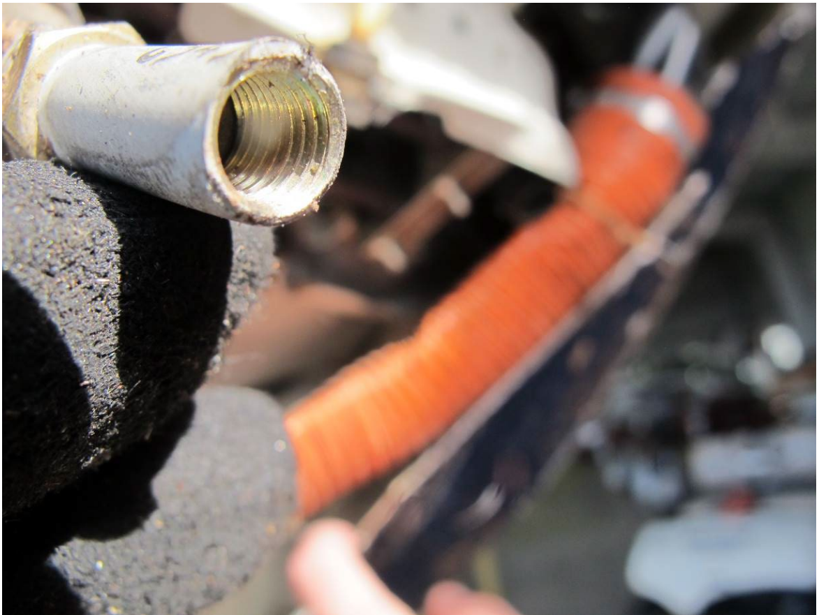
Above and below: Disconnect TA at forward end of C343-11 push pull tube.
