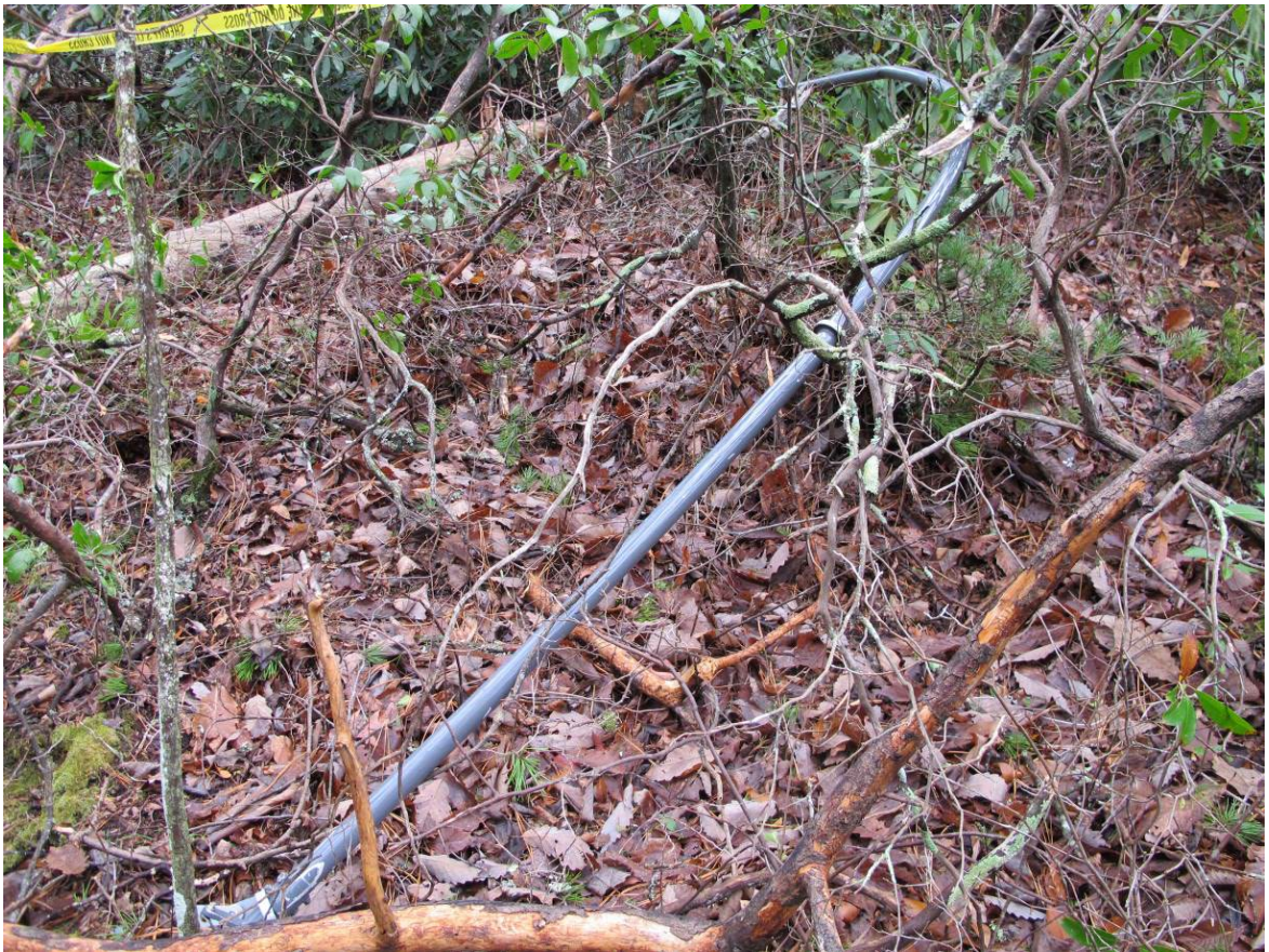
Forward section of tail rotor driveshaft.
