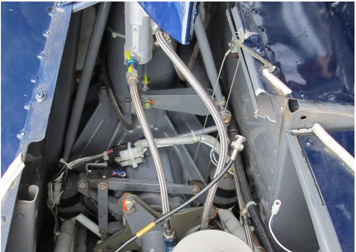
Main rotor gearbox.
