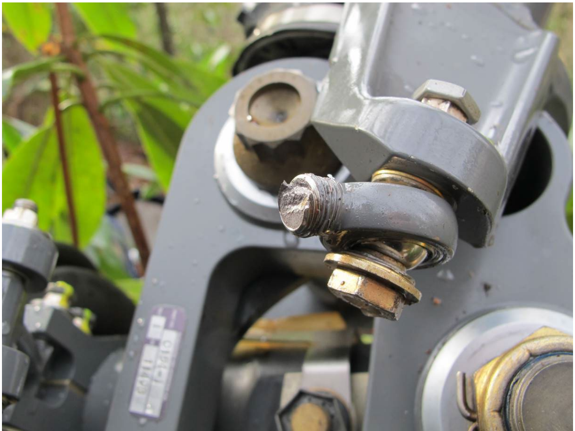
Disconnect D in upper rod end of C258-6 pitch link.
