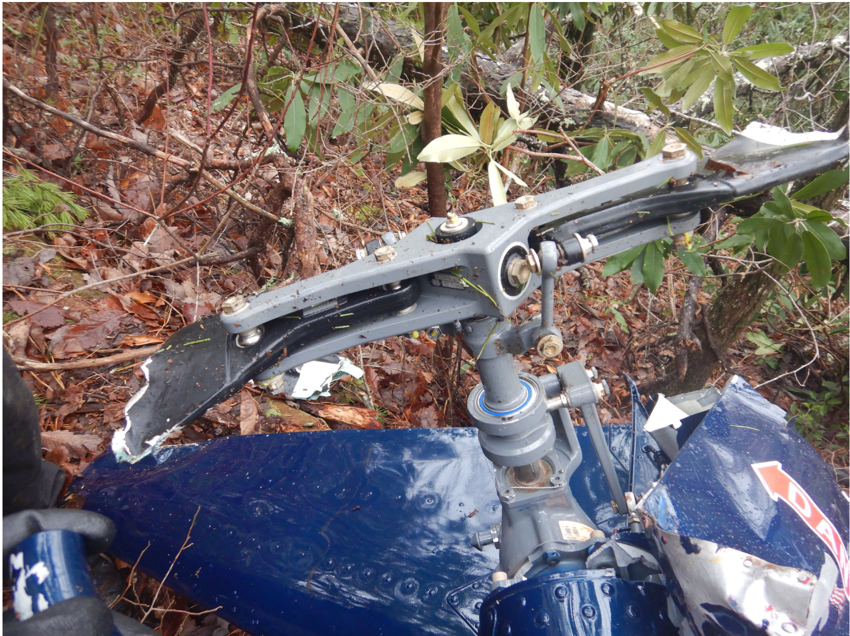
Photo 8 – Tail Rotor Hub (NTSB Photo)
