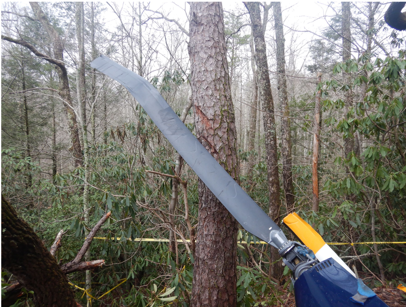
Photo 6 – Main Rotor Blade and Hub (NTSB Photo)
