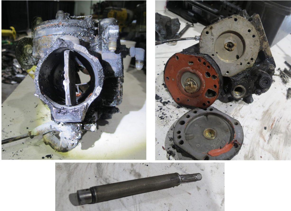
Figure 28 - Fuel Servo - Intact (Top Left) Partially Disassembled (Top Right) Fuel Inlet Screen (Bottom)
