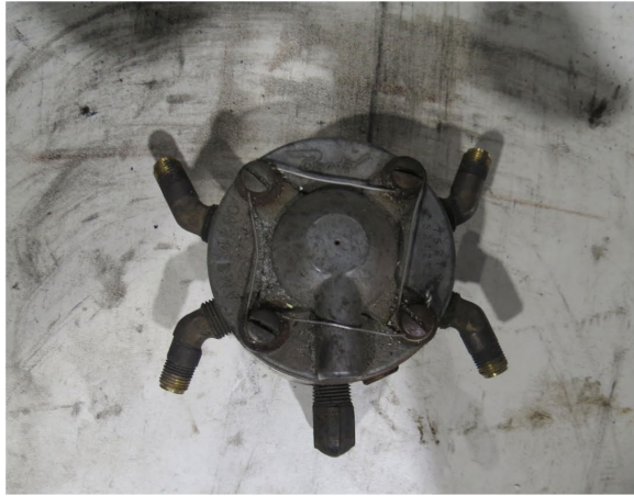
Figure 26 - Fuel Flow Divider - Intact (Left) Partially Disassembled (Right)
