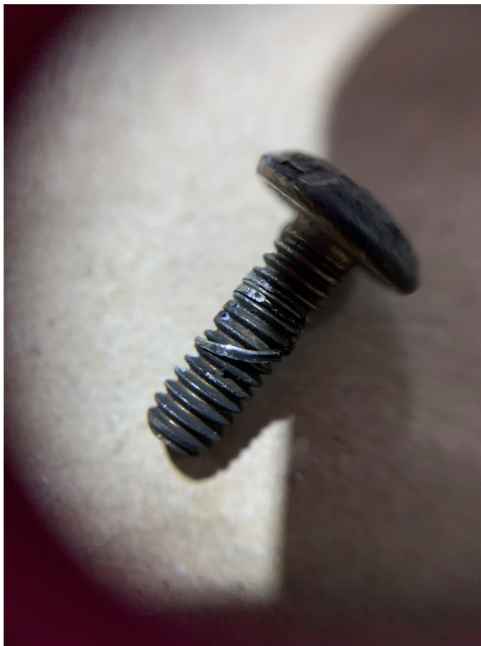
Figure 10 Right Speedbrake Mounting Bolt (Left) and Corresponding Hole in Speedbrake Assembly (Right)
