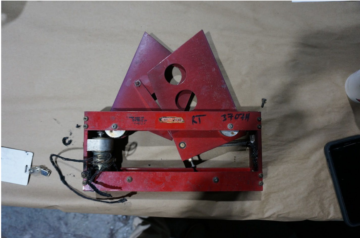
Figure 11 - Right Speedbrake Positioned Where Panels Rubbed Each Other, When Manually Extended
