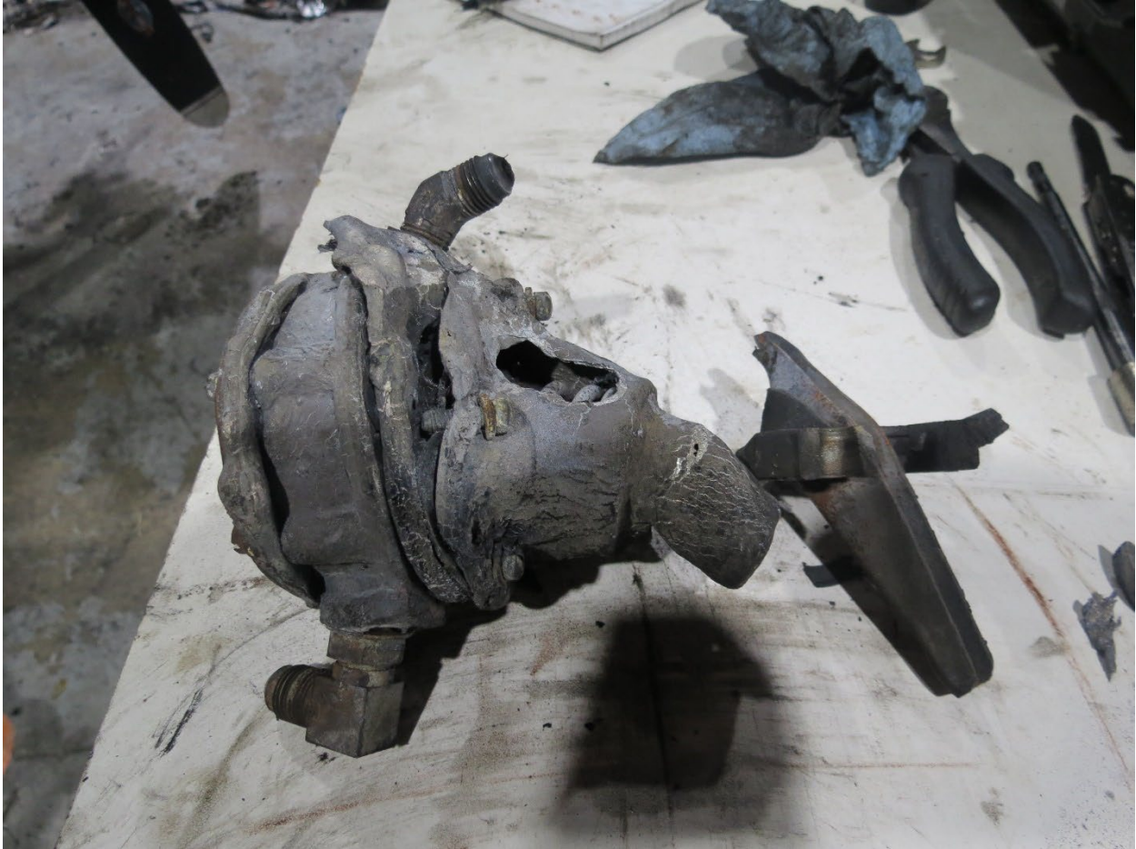
Figure 25 Engine Driven Fuel Pump
