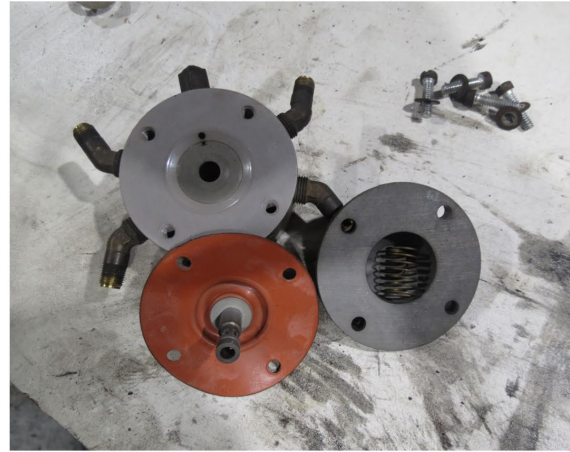
Figure 26 - Fuel Flow Divider - Intact (Left) Partially Disassembled (Right)
