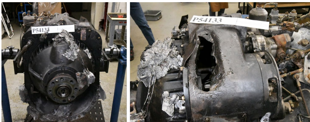
Photo 41- (L) Nose Cone, Inlet, (R) AGB Case Hole
