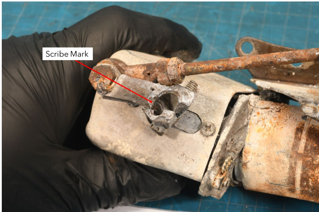
Photo 11- Fuel Shutoff Valve, Input Shaft Scribe
