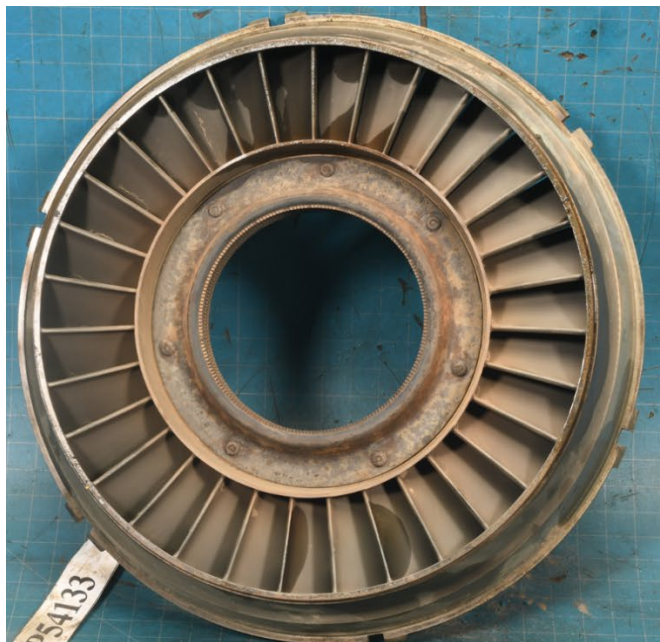
Photo 55- 3 rd Stage Turbine Stator, (L) Pressure Side, (R) Suction Side
