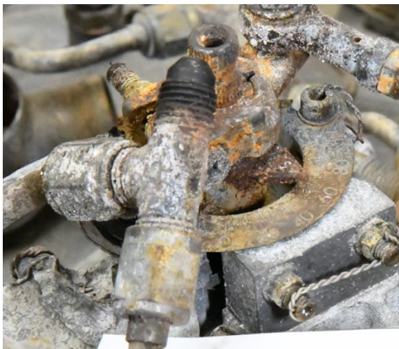
Photo 43- (L) Fuel Control Unit Power Lever Linkage Dial Indicator, (R) Propeller Pitch Control Dial Indicator.
