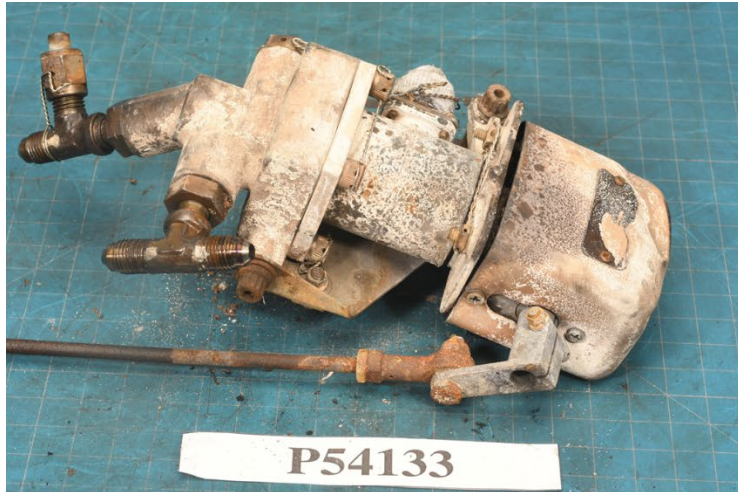
Photo 44- (L) Fuel Shutoff Valve, (R) Input Shaft Scribe
