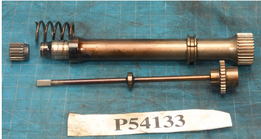
Photo 47- High Speed Pinion Power Coupling Shaft and NTS Quill Shaft
