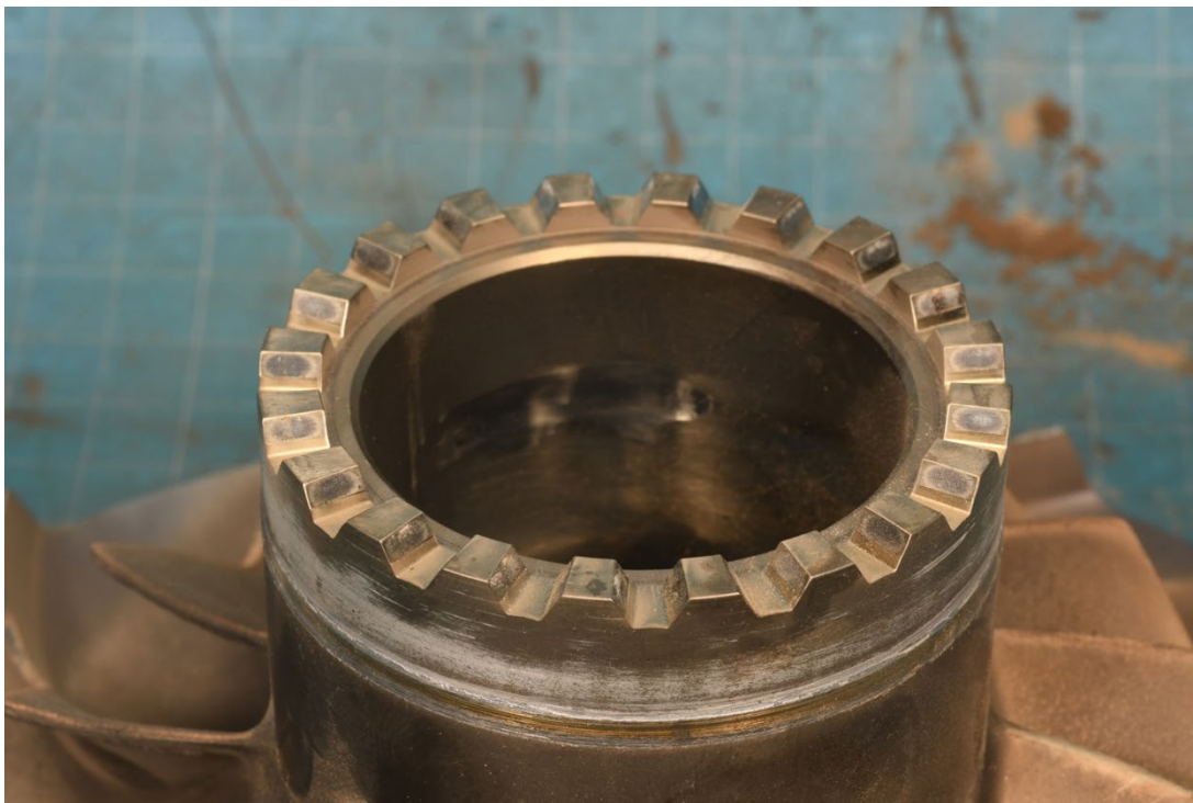
Photo 62- 2 nd Stage Compressor Impeller Hub Rotational Scoring
