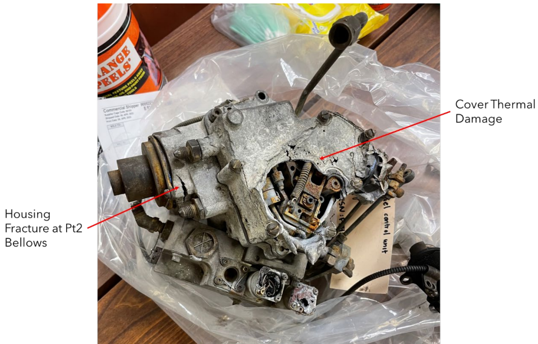
Photo 64- FCU, as Received at Woodward
