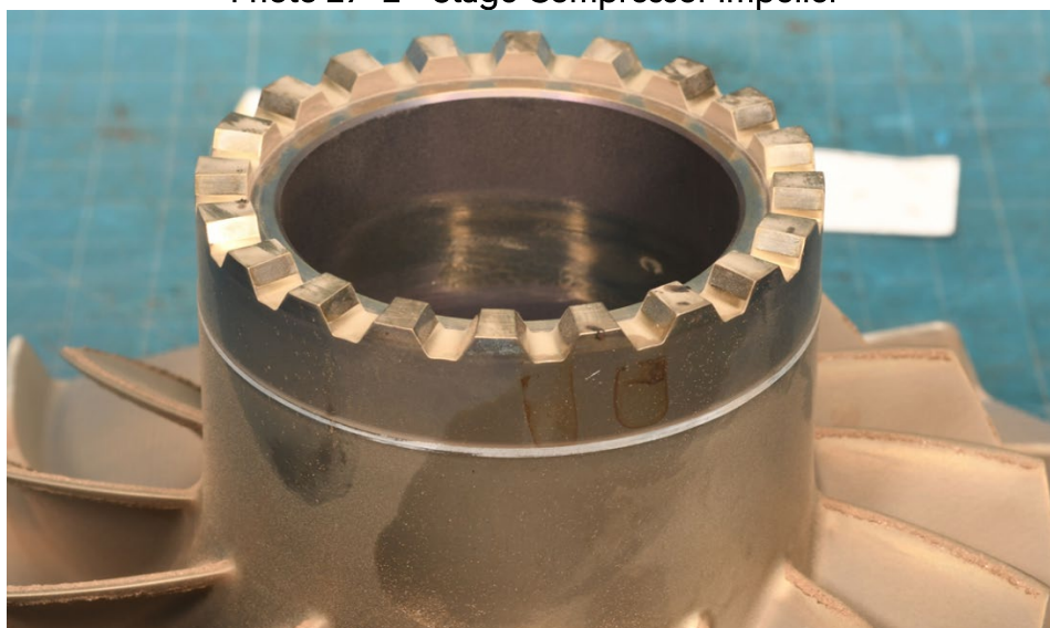
Photo 28- 2nd Stage Compressor Impeller Hub Curvic Scoring
