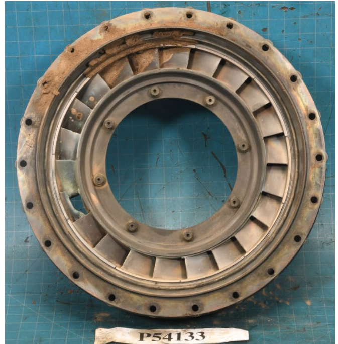
Photo 50- 1 st Stage Turbine Stator, (L) Pressure Side, (R) Suction Side
