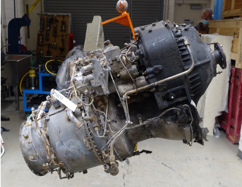
Photo 39- No. 2 Engine, Right Side, As Received (Upside Down Relative to Installed Orientation)
