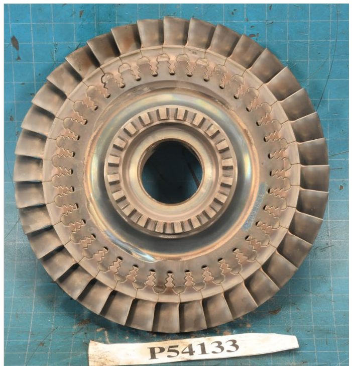
Photo 51- 1 st Stage Turbine Rotor, (L) Leading Edge, (R) Trailing Edge
