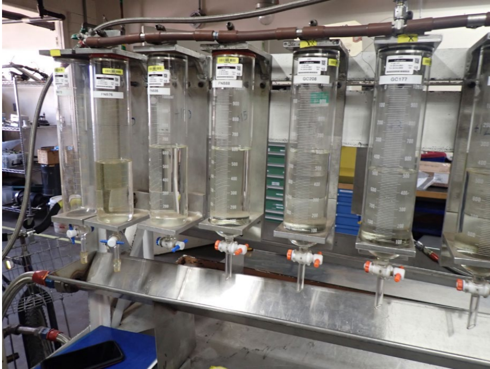
Photo 32- Fuel Nozzle Flow Test Setup (Photo Courtesy of Honeywell)
