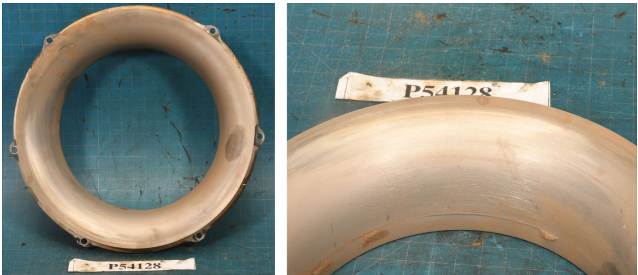
Photo 26- 1 st Stage Compressor Shroud
