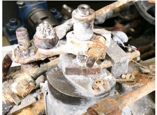
Photo 9- (L) Fuel Pump and Fuel Control, (R) Fuel Control Power Lever Linkage Dial Indicator
