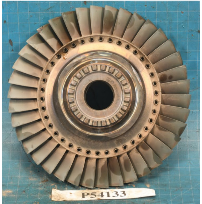
Photo 54- 2 nd Stage Turbine Rotor, (L) Leading Edge, (R) Trailing Edge
