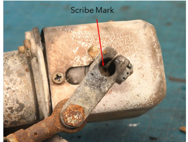
Photo 44- (L) Fuel Shutoff Valve, (R) Input Shaft Scribe
