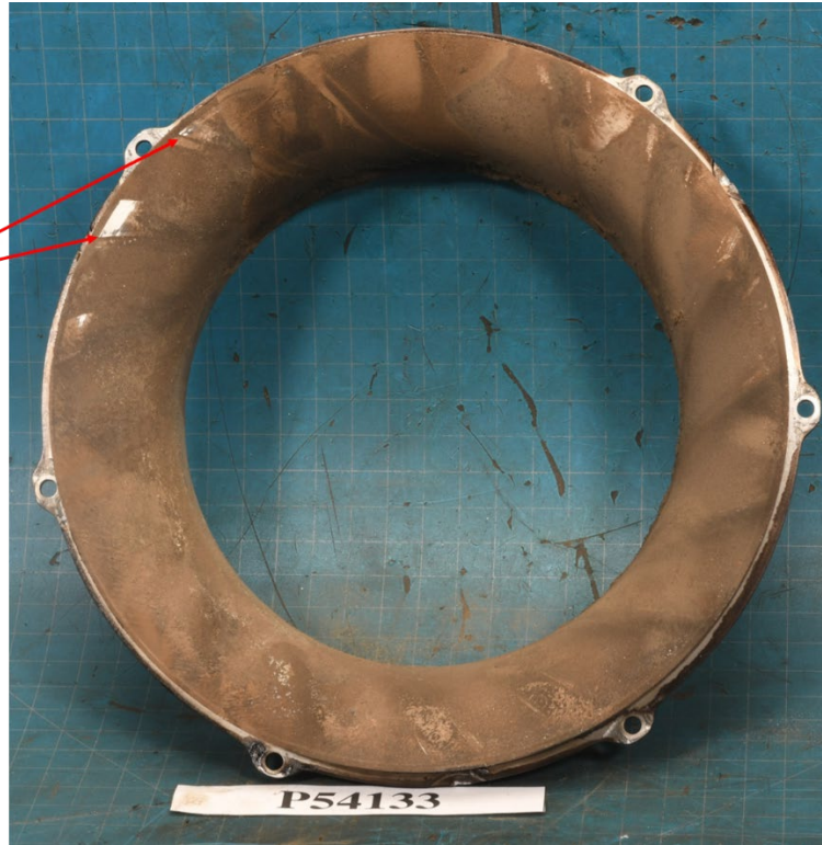
Photo 60- 1 st Stage Impeller Shroud, Rotational Scoring
