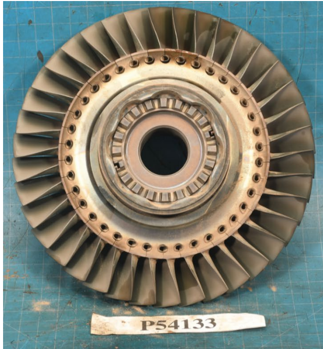
Photo 54- 2 nd Stage Turbine Rotor, (L) Leading Edge, (R) Trailing Edge
