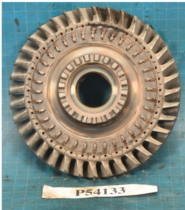
Photo 51- 1 st Stage Turbine Rotor, (L) Leading Edge, (R) Trailing Edge
