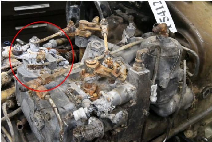
Photo 9- (L) Fuel Pump and Fuel Control, (R) Fuel Control Power Lever Linkage Dial Indicator
