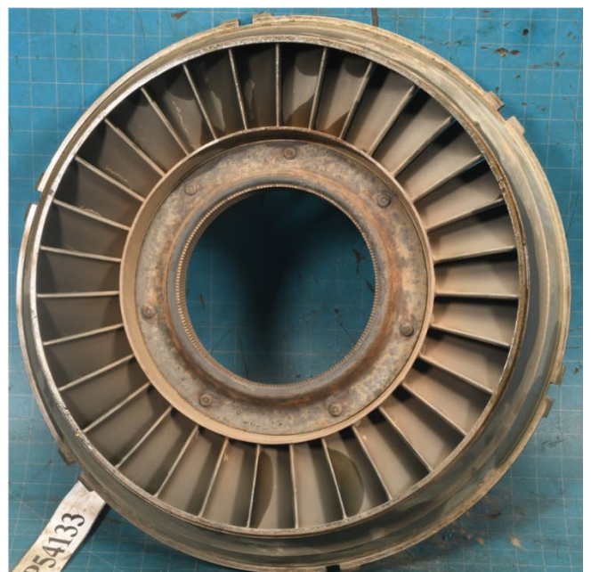
Photo 55- 3 rd Stage Turbine Stator, (L) Pressure Side, (R) Suction Side
