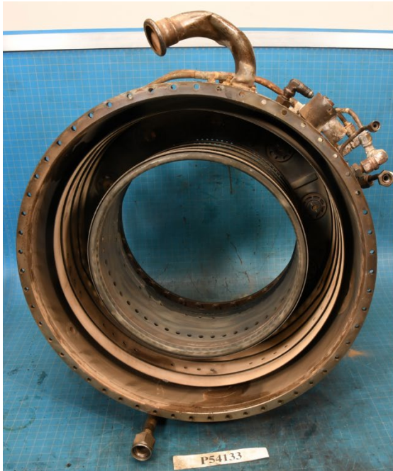
Photo 57- (L) Combustion Liner, (R) Fuel Nozzles
