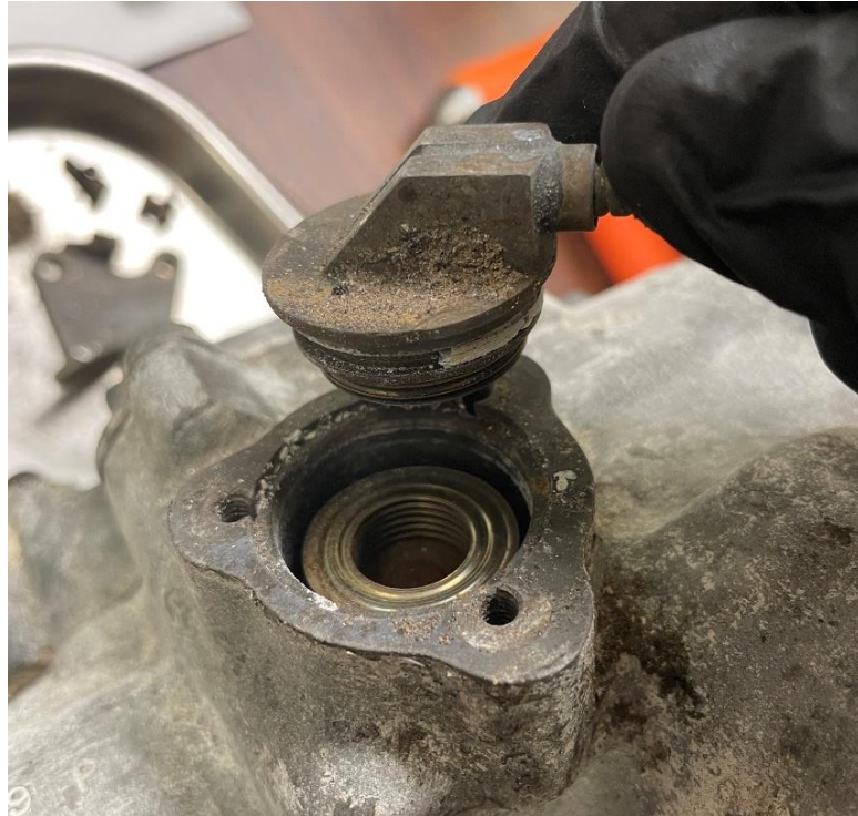
Figure 1. T2 Sensor Bellows Removal
