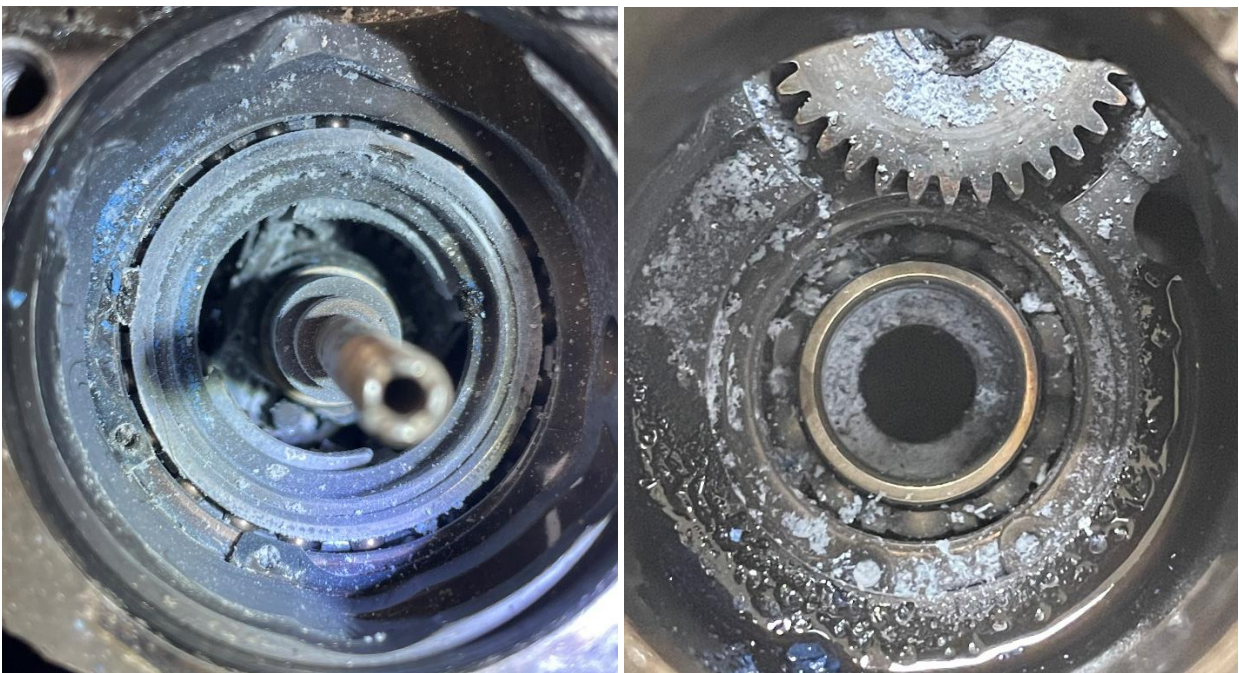
Figure 5. Debris on Underspeed Governor and Housing Bore
