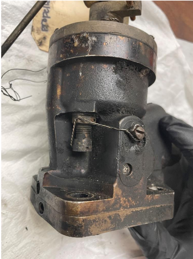
Figure 3 Missing Magnetic Coil Wires
