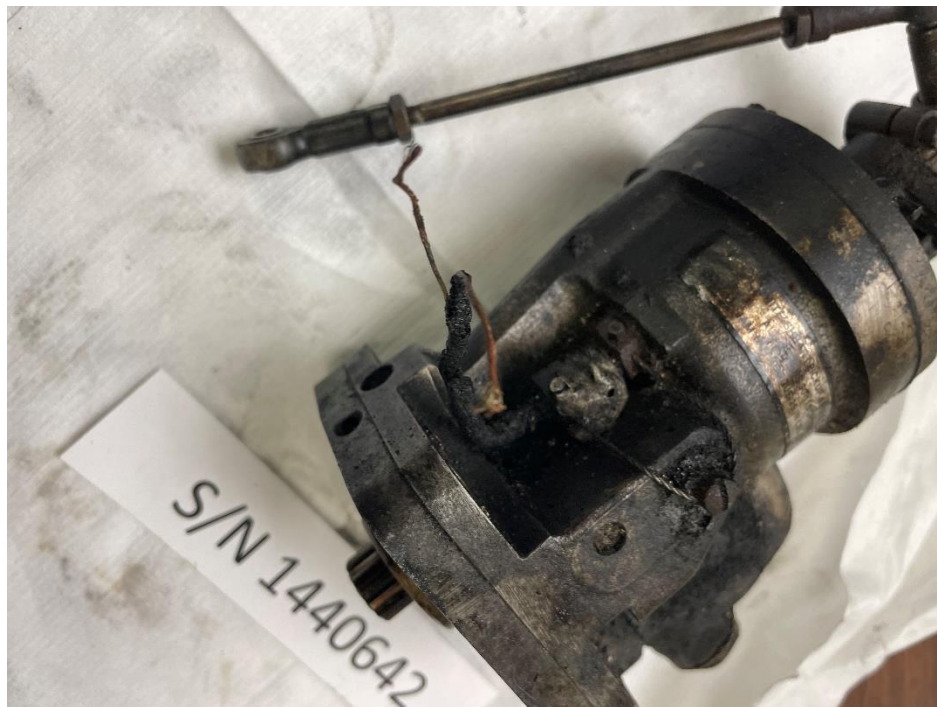
Figure 2 Severed Magnetic Pickup Coil Wire
