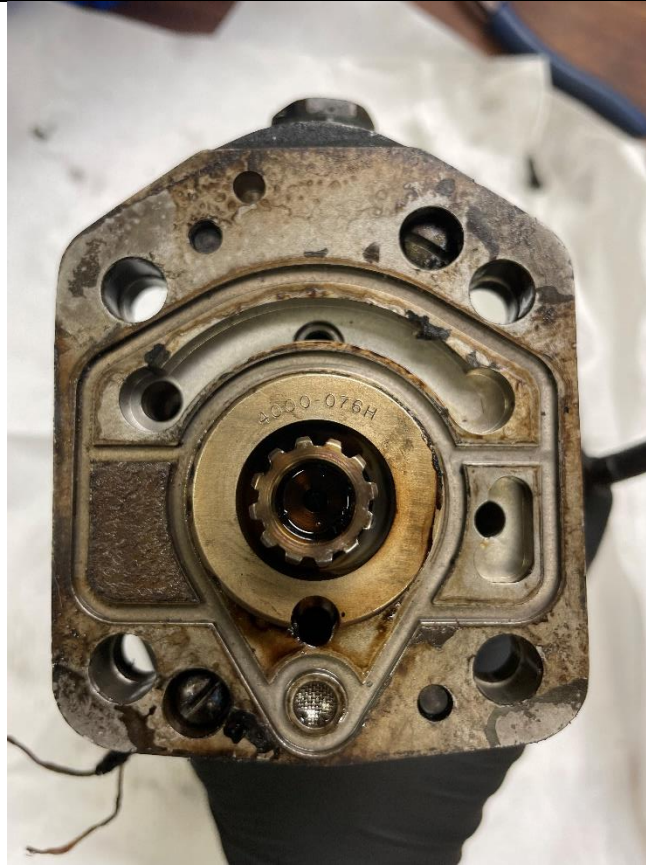
Figure 3 Missing Baseplate Packing
