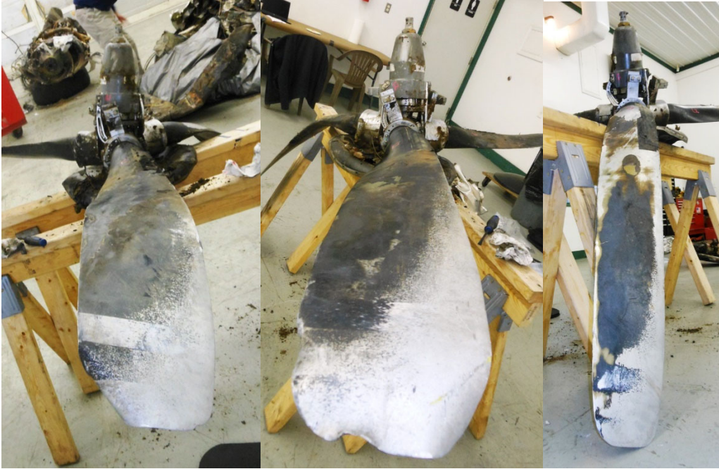
Photo #28 - Left propeller blade damage, as-presented
