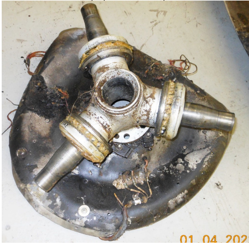
Photo #26 - Left propeller hub and spinner bulkhead
