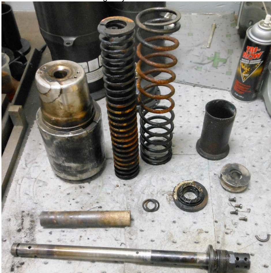
Photo #7 - Right hydraulic unit disassembled
