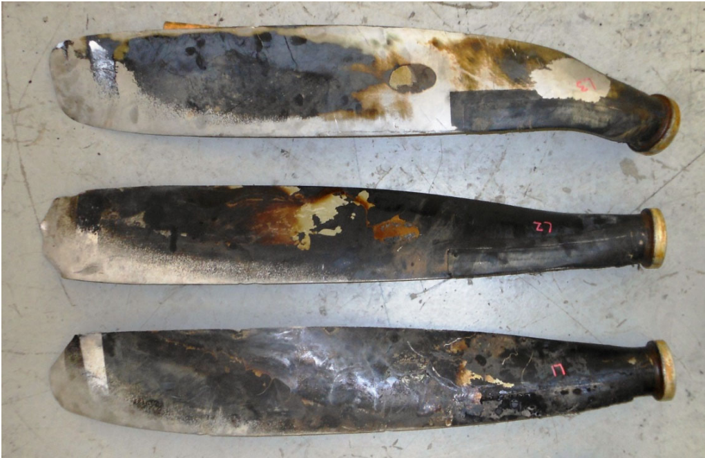
Photo #32 - Left blades camber side
