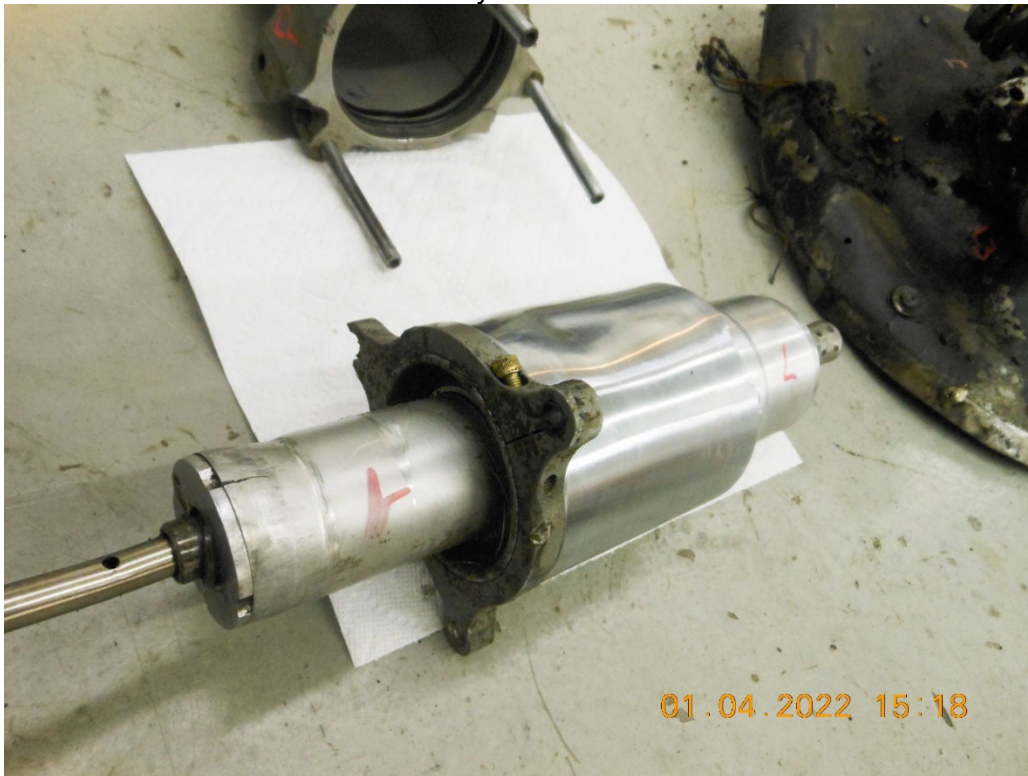
Photo #21 - Left hydraulic unit in final state
