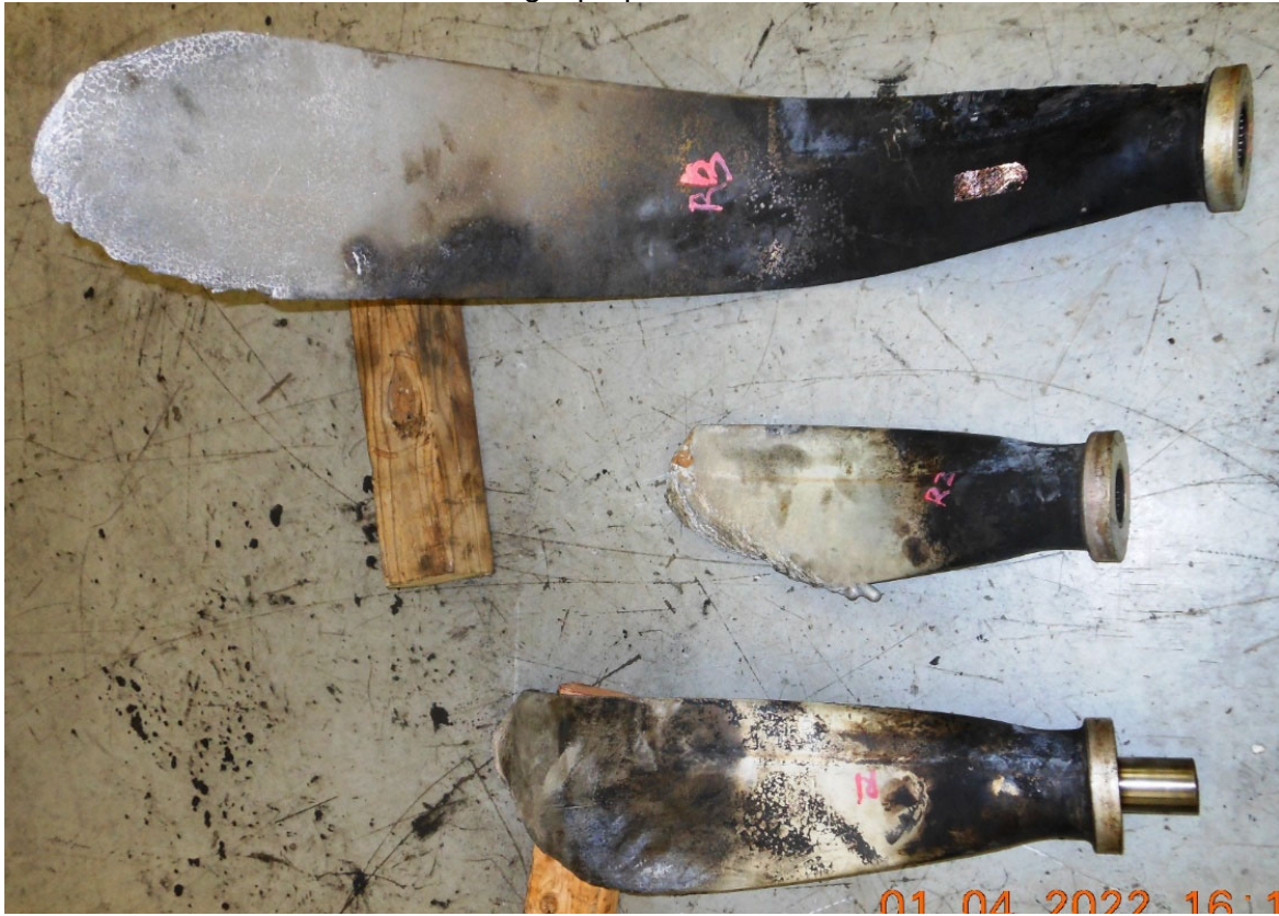
Photo #16 - Right propeller blades, face side
