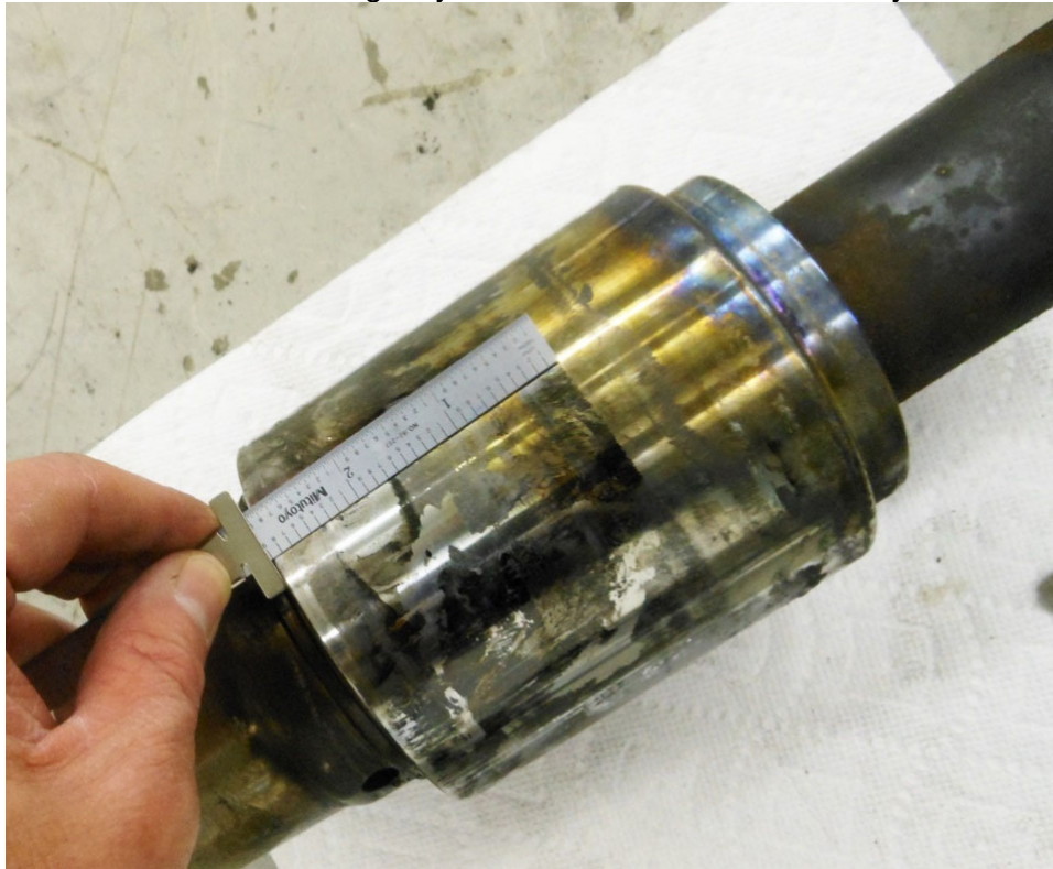
Photo #12 - Right cylinder discoloration discontinuity
