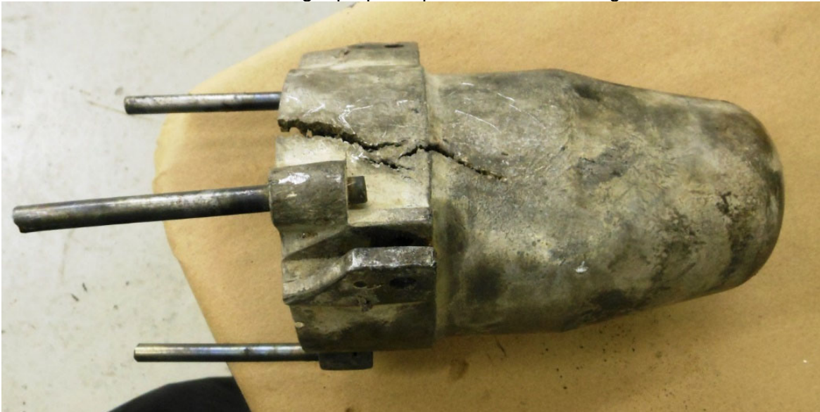
Photo #8 - Right propeller piston thermal damage
