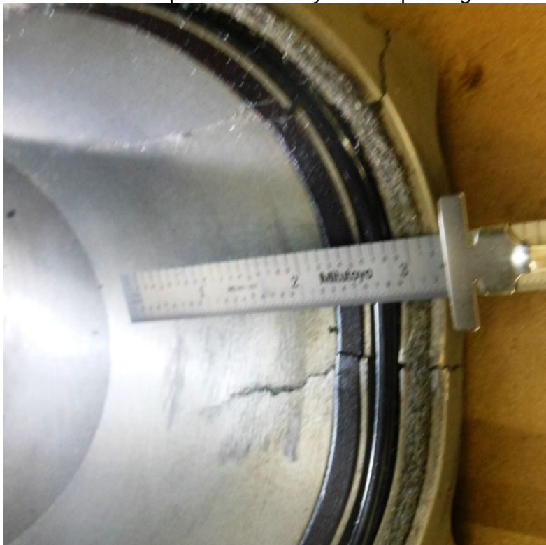
Photo #25 - Left piston internal cylinder impact signatures
