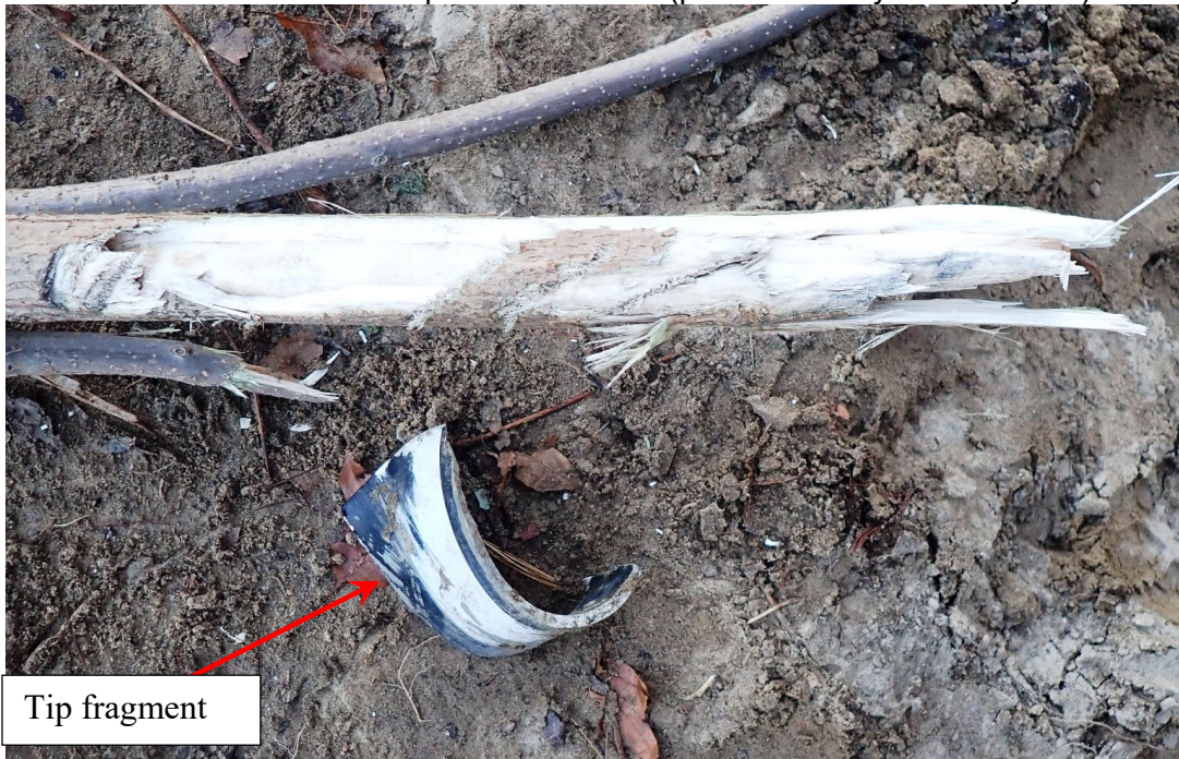
Photo #2 – Fractured tip at crash scene (photo courtesy of Honeywell)
