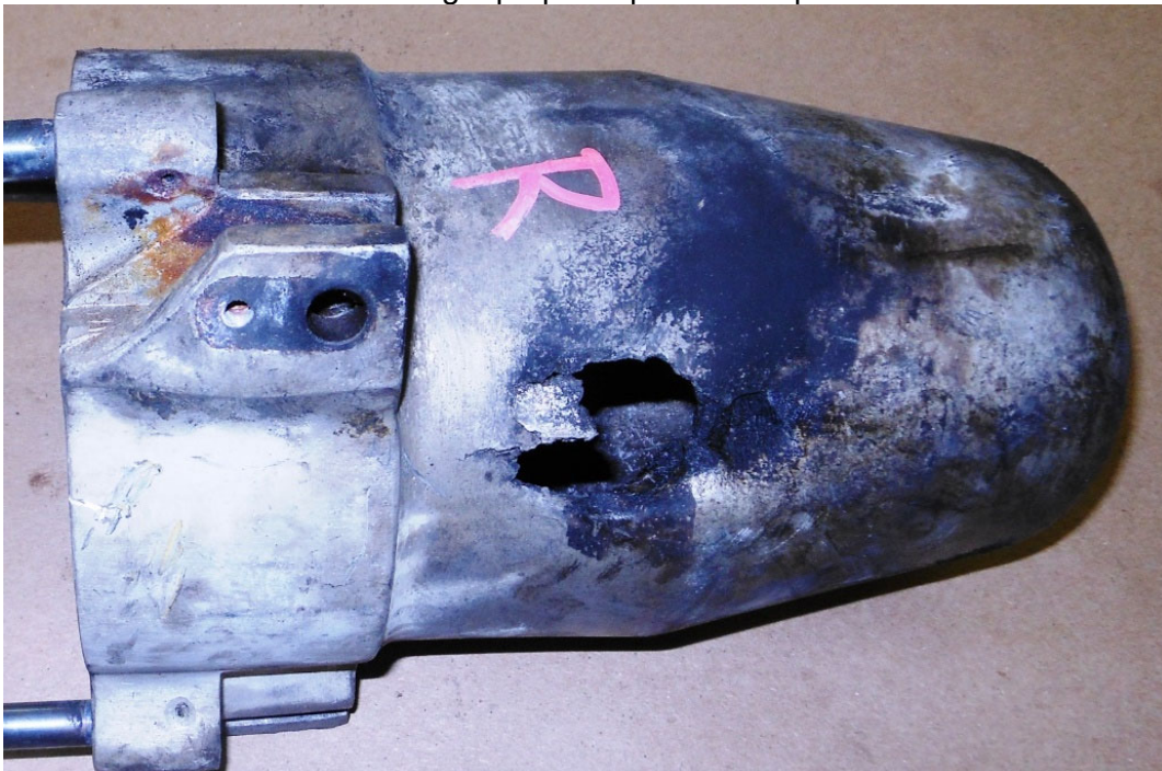
Photo #9 - Right propeller piston hole/puncture
