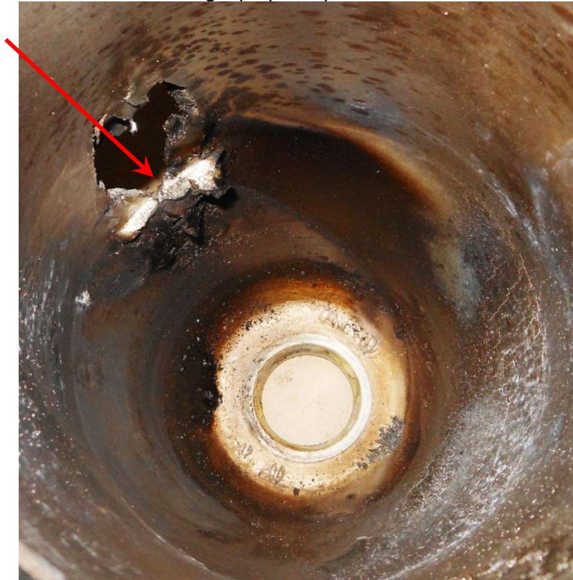
Photo #10 - Right propeller piston internal surface
