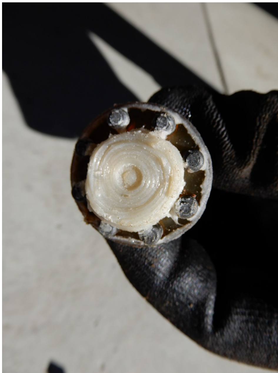
Photo 7 – Vacuum Pump Drive (NTSB Photo)
