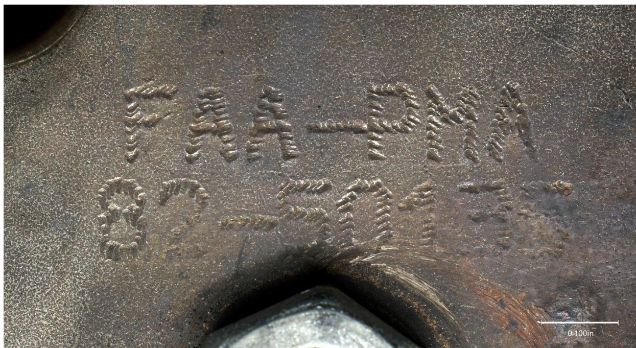
Figure 7: Image of information imprinted on the rotor hub: “FAA-PMA” and “82-50135”.
