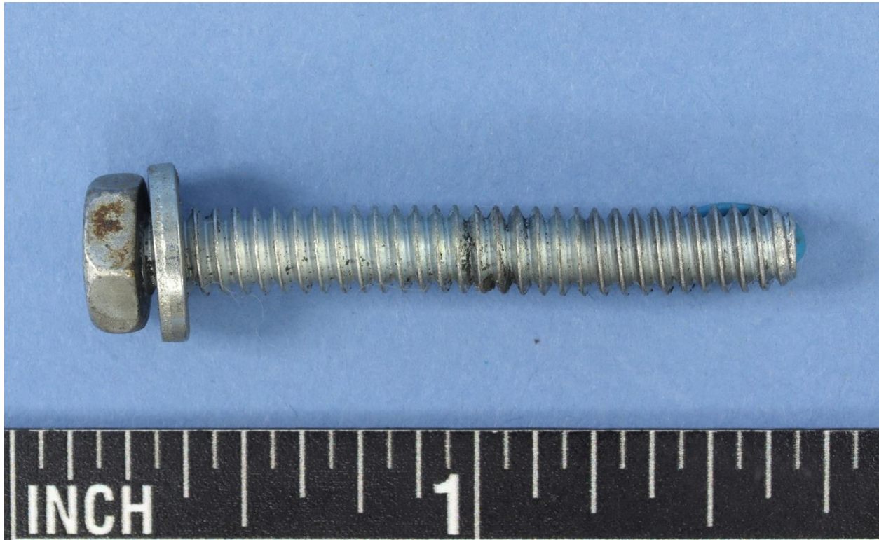
Figure 3: Image of the screw after it was removed from the pump. There was no apparent locking compound on the threads and the threaded section was bent.
