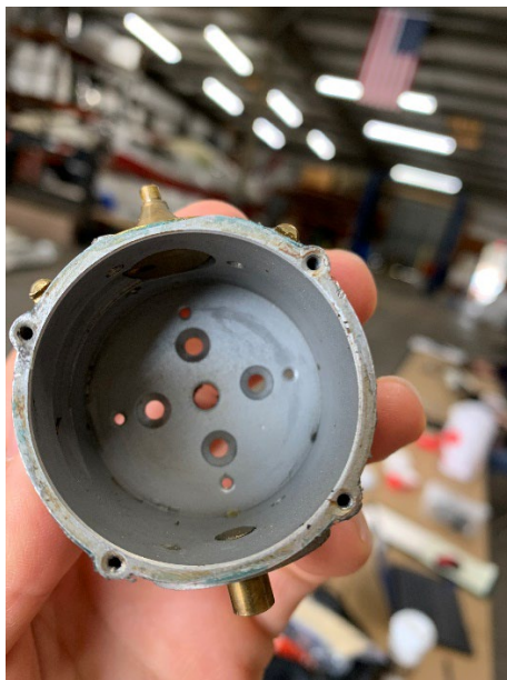
Photos 10-13: View of the attitude indicator gyro and its casing disassembled postaccident
