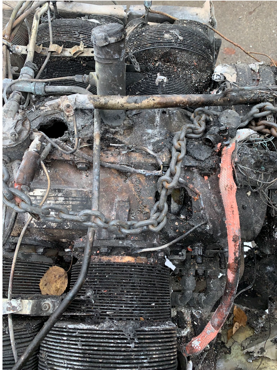
Photo 9 – View of top side of engine showing 2 holes.
