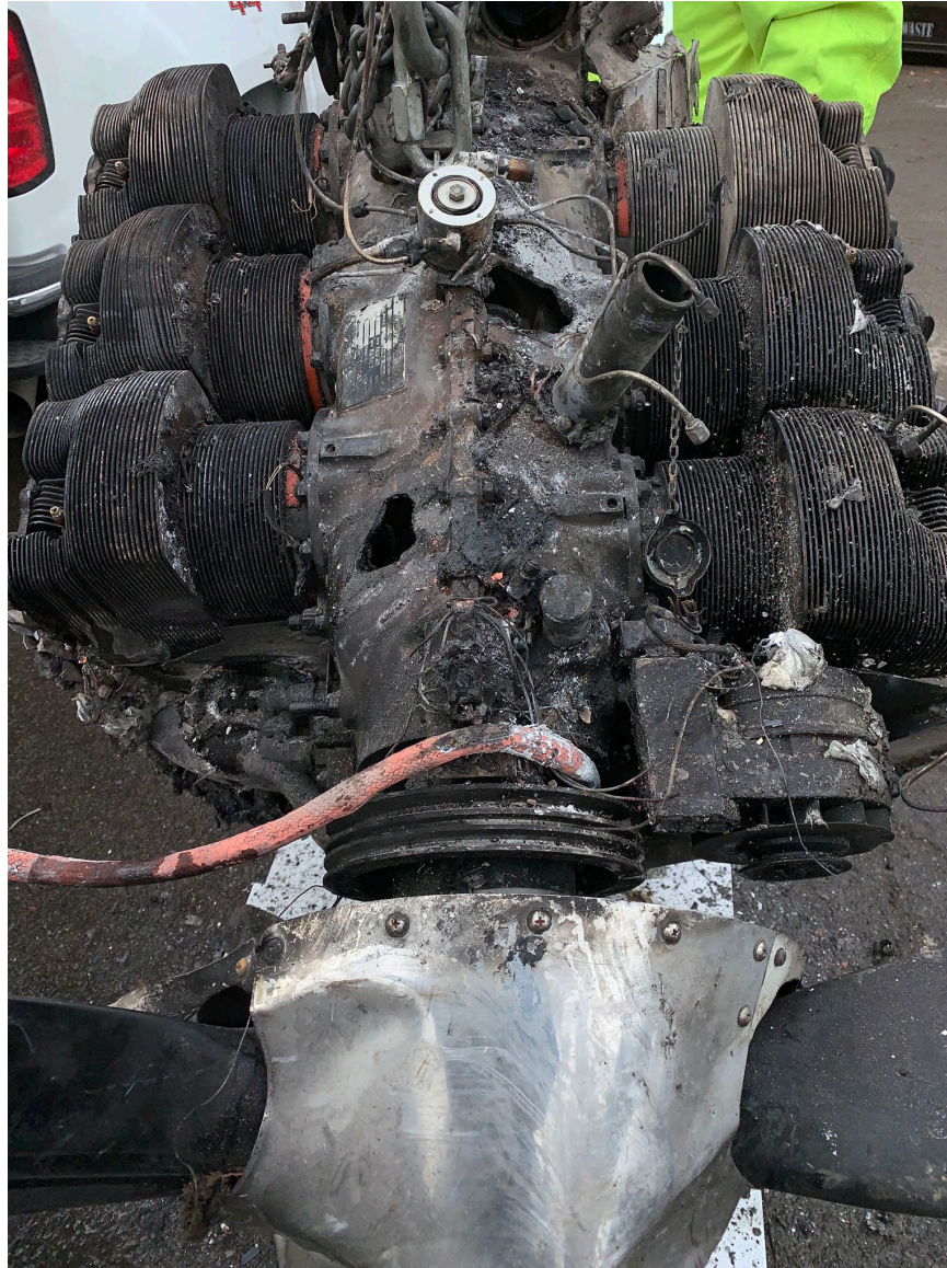
Photo 10 – Entire top view of engine showing holes in case and propeller spinner.
