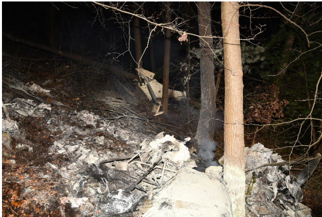
Figure 1 Main wreckage smoldering in foreground and empennage up hill about 30 ft away.
