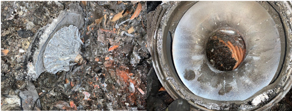
Figure 3 Turbo and compressor wheel showing static impact marks.
