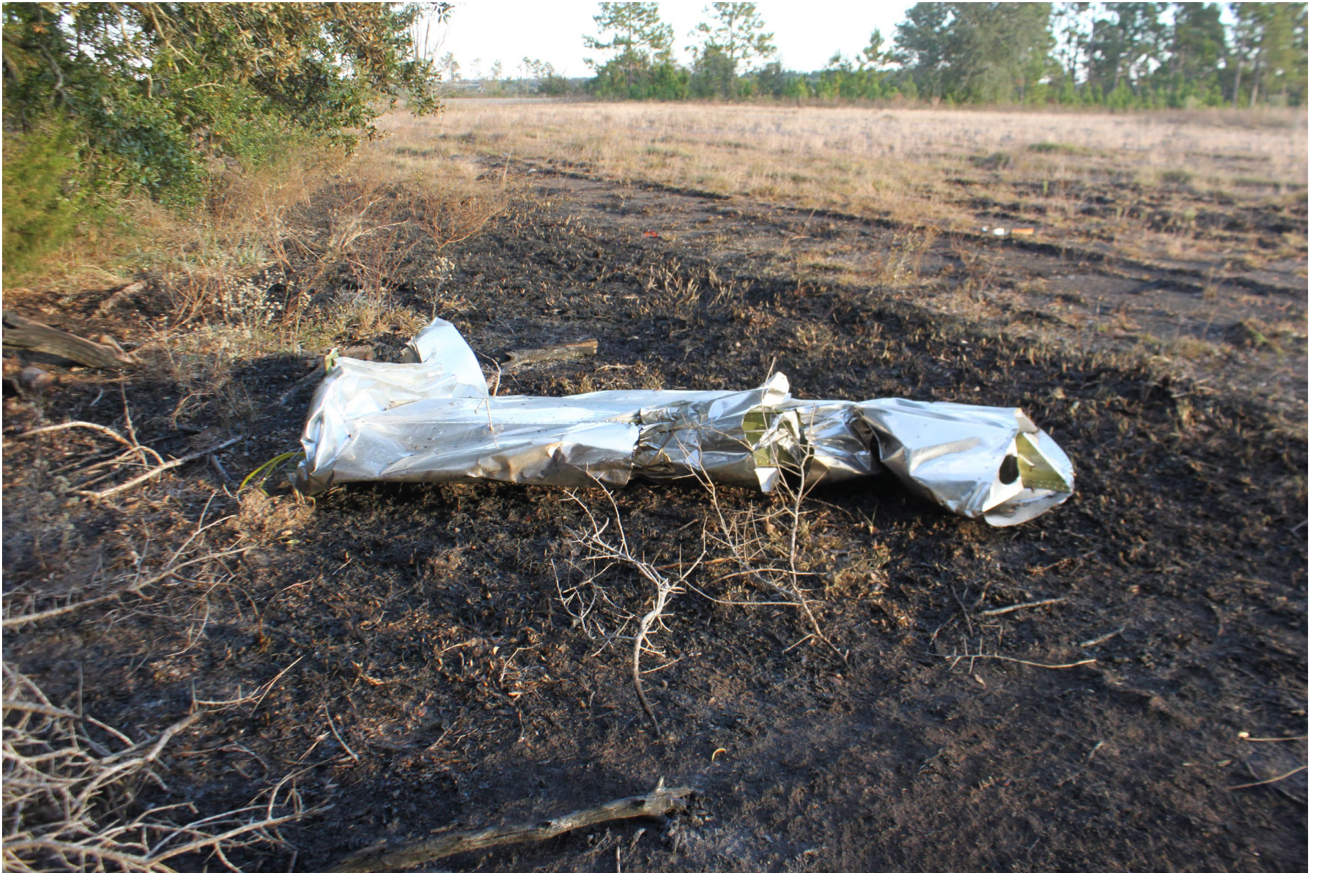
Photo 3 - NTSB Digital Photograph. View of the Separated Right Wing.
