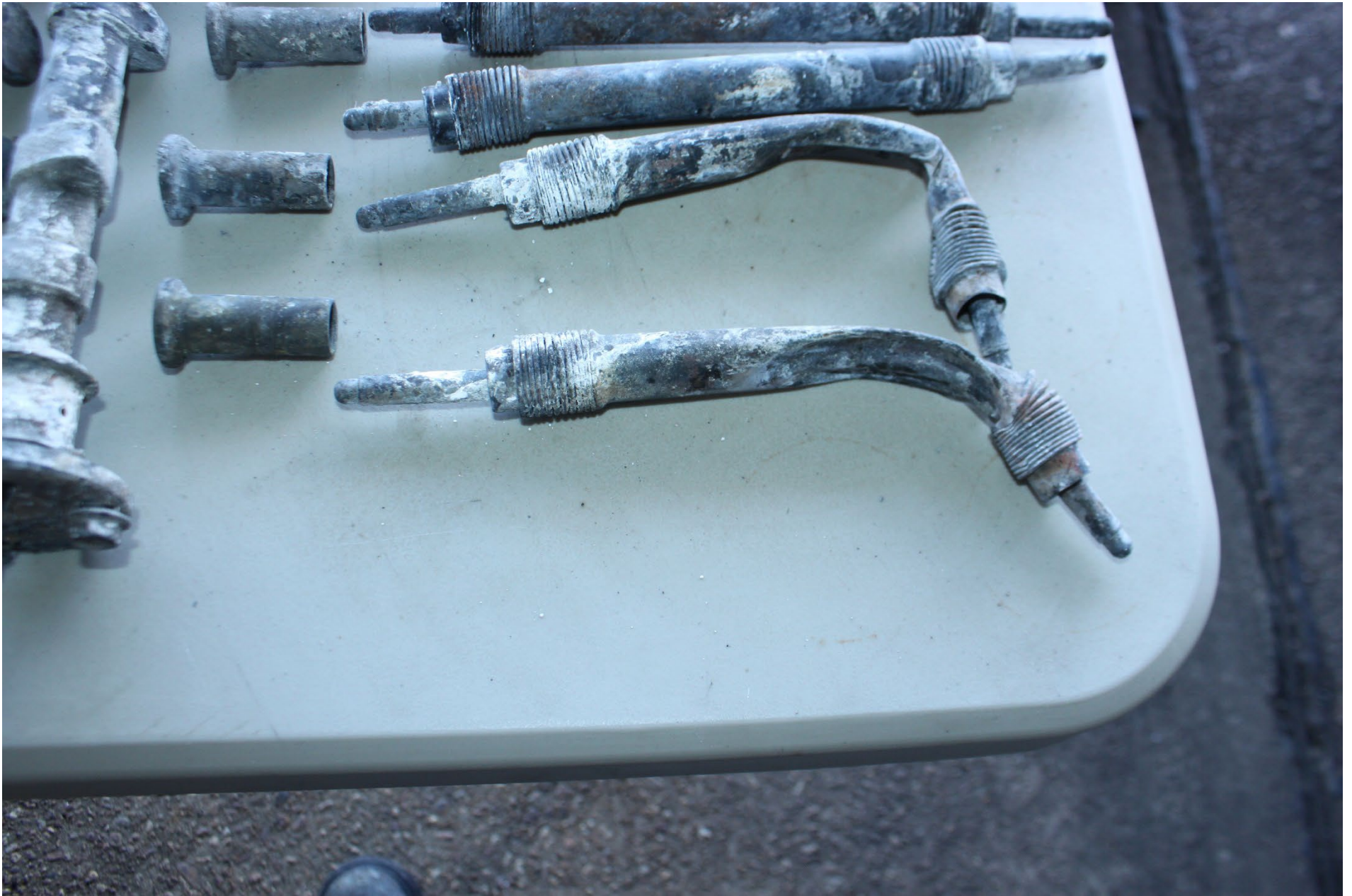
Photo 7 - NTSB Digital Photograph. View Depicting the Pushrods and Pushrod Housings from the Nos. 1 and 2 Cylinders. Note the Near 90 degree Bending of Two of them.
