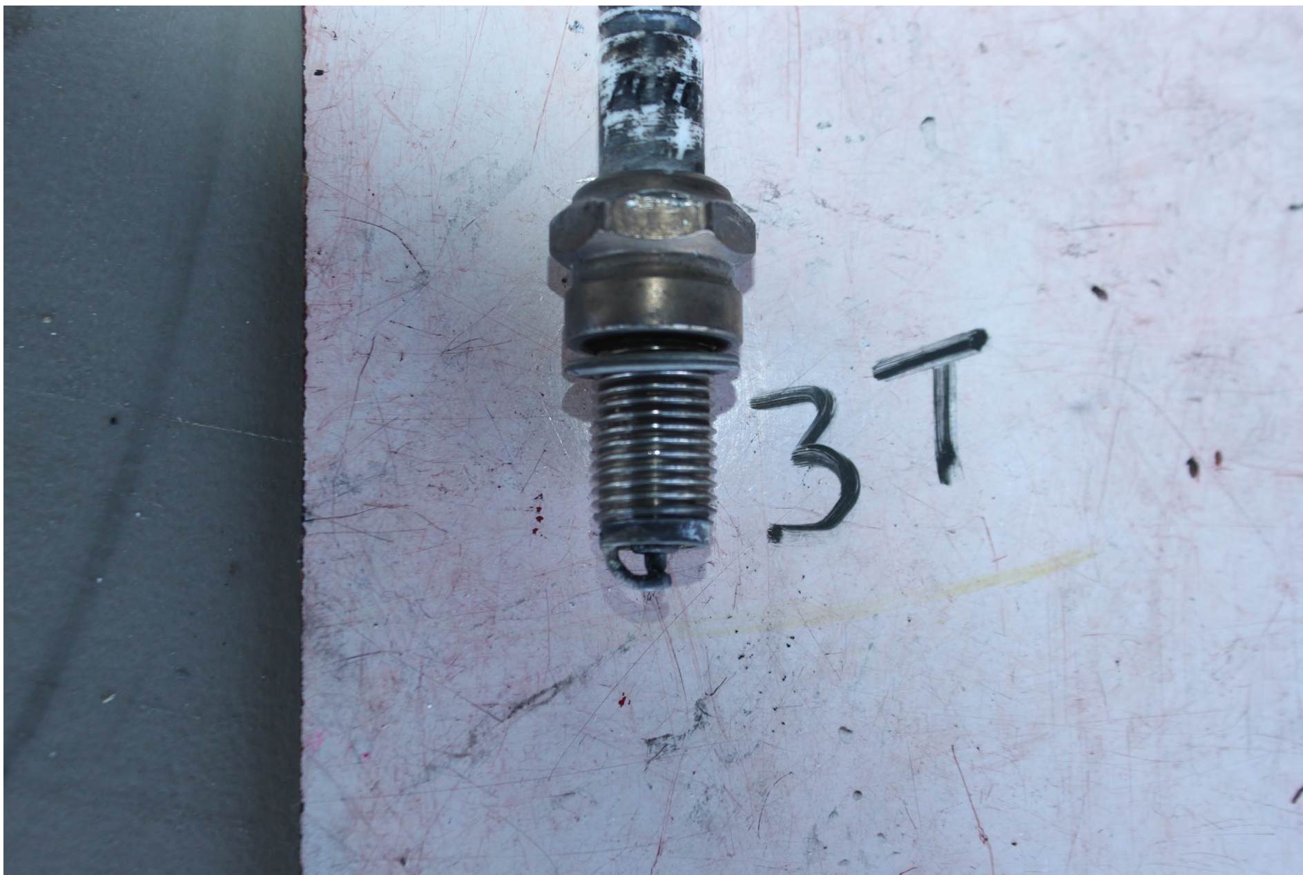
Photo 6 - NTSB Digital Photograph. View of the No. 3 Top Spark Plug. Note the Ground Electrode Touching the Center Electrode.
