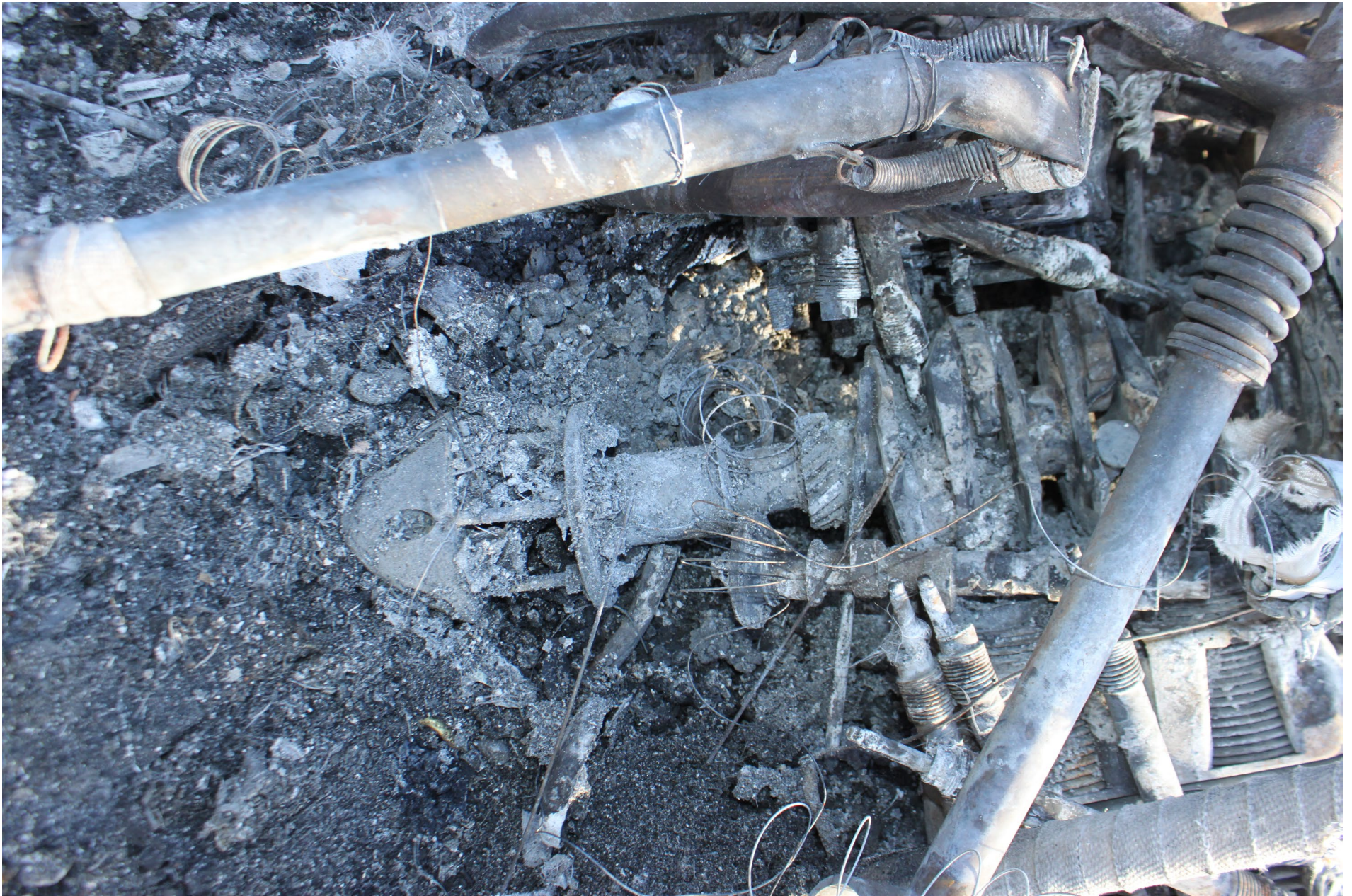
Photo 5 - NTSB Digital Photograph. View of the Extensively Heat Damage Crankcase Halves. Note the visible Crankshaft, camshaft, and Valve Train Components.
