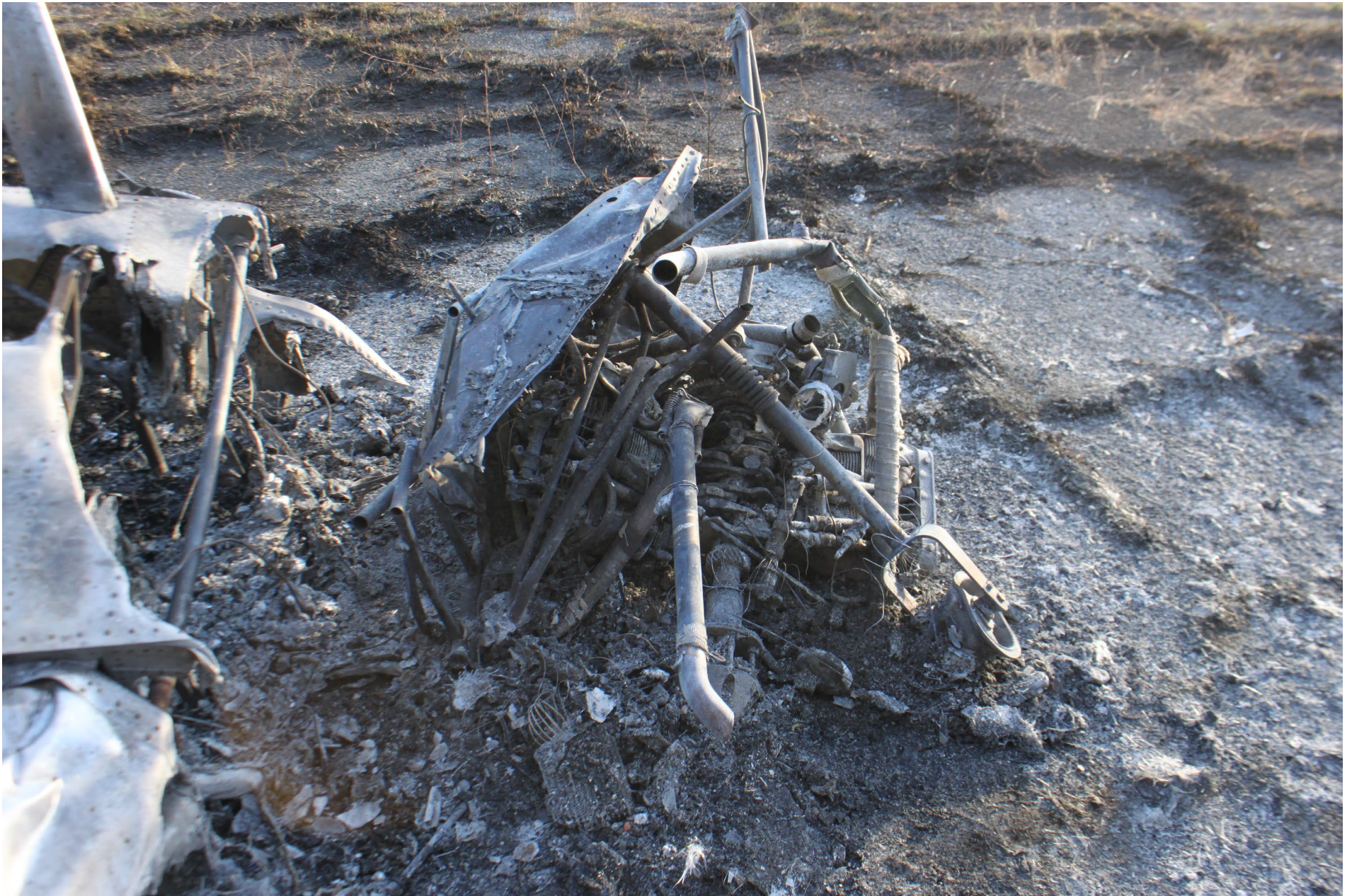
Photo 4 - NTSB Digital Photograph. View of the Firewall and Remains of the Engine Assembly. Note the Extensive Fire Damage.
