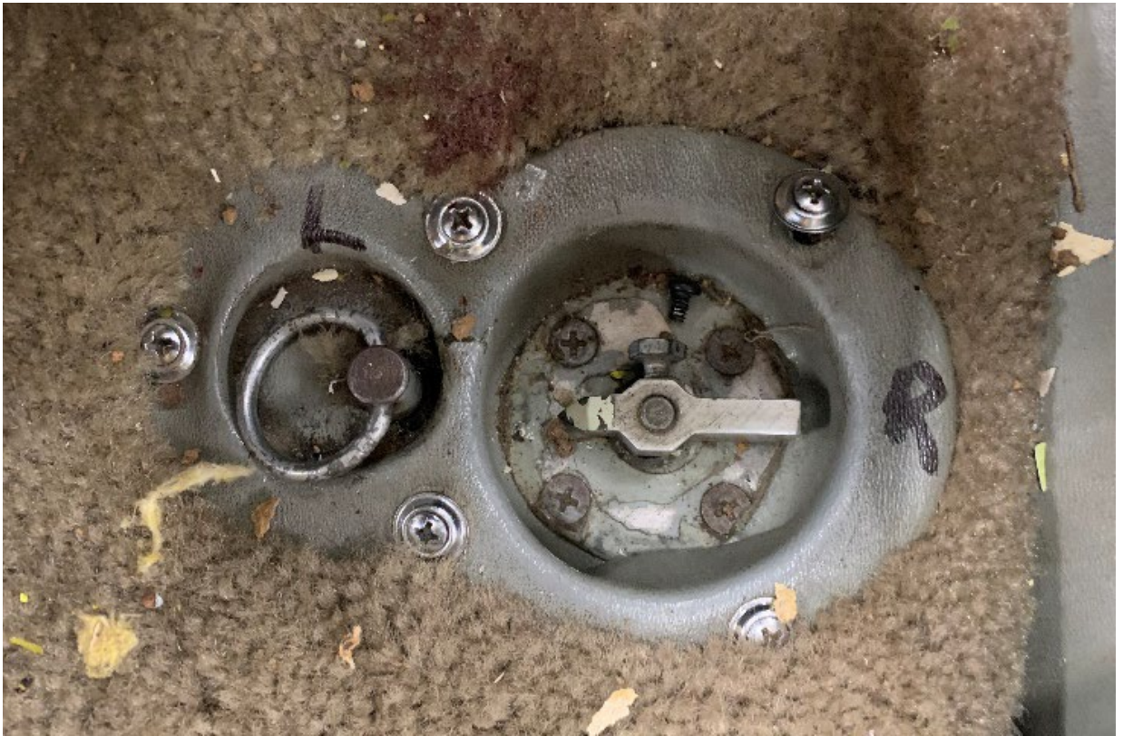
Figure 7. View of fuel selector as found.
