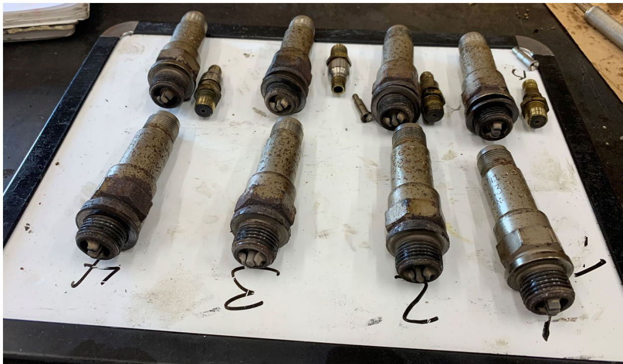
Figure 10. Spark plugs and fuel injector nozzles.
