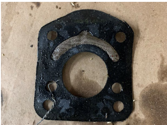
Figure 14. View of propeller governor screen.
