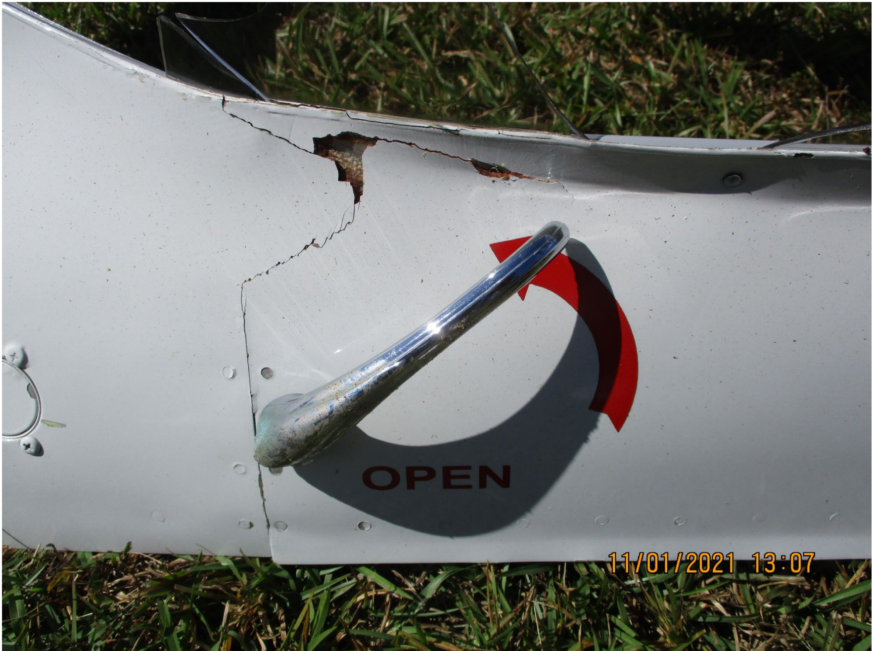
Photo 5 – canopy handle in open position
