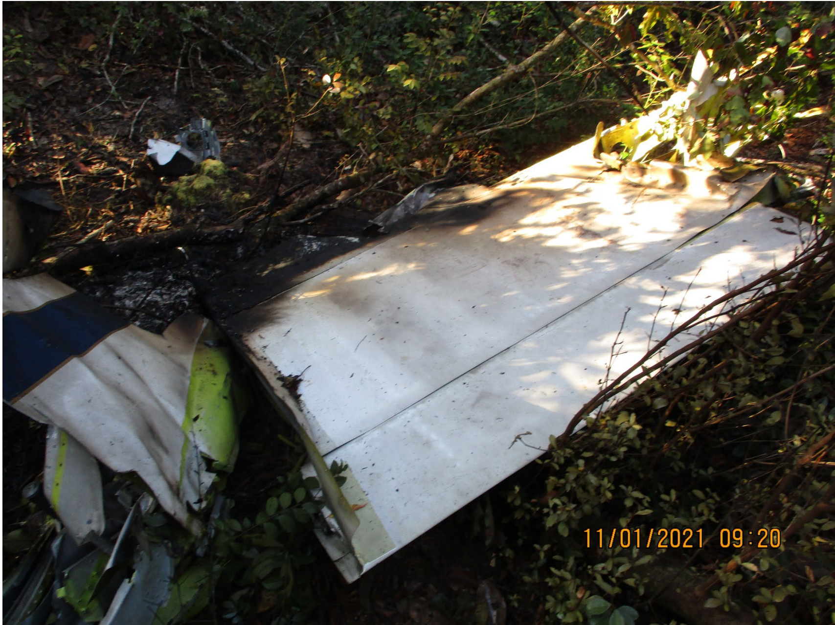
Photo 2 – wing section burnt
