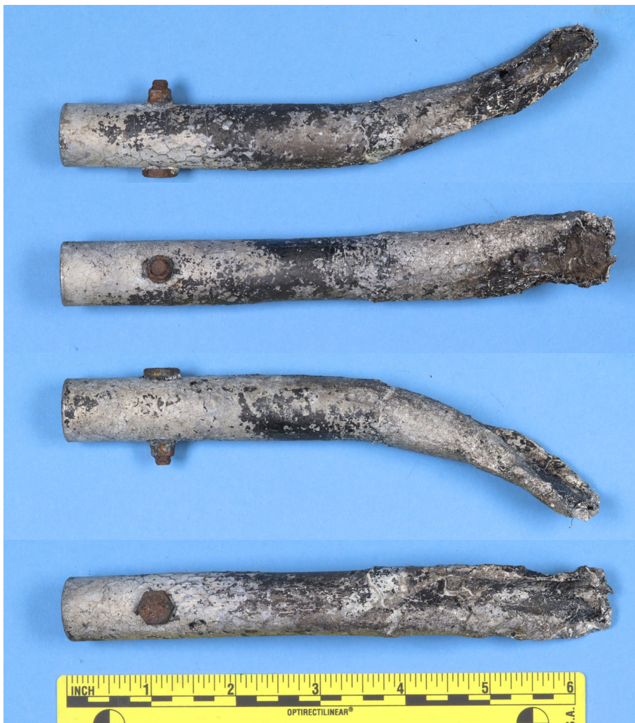
Figure 1 Four views of the fire-damaged pushrod piece.
