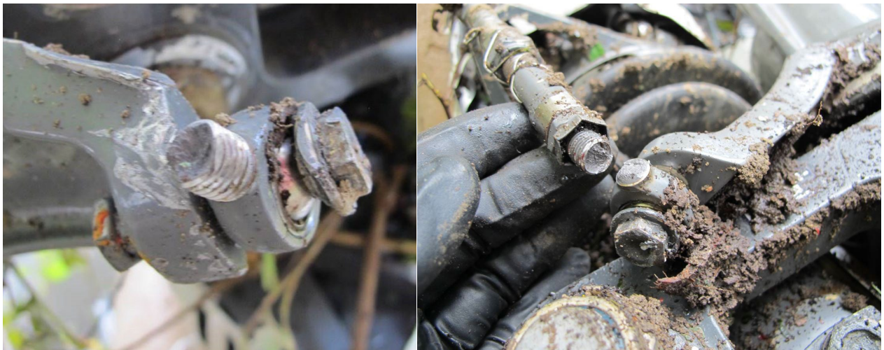
Figure 24 - Fractures at Upper ends of the Two Main Rotor Pitch Change Links
