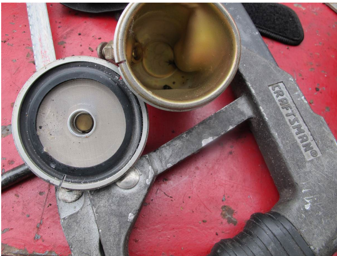
Figure 18 - Gascolator - Top (and Screen) Removed
