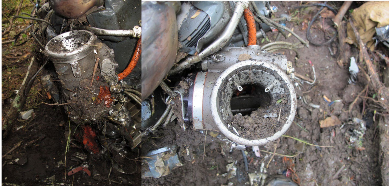
Figure 58 - Fuel Servo as Found
