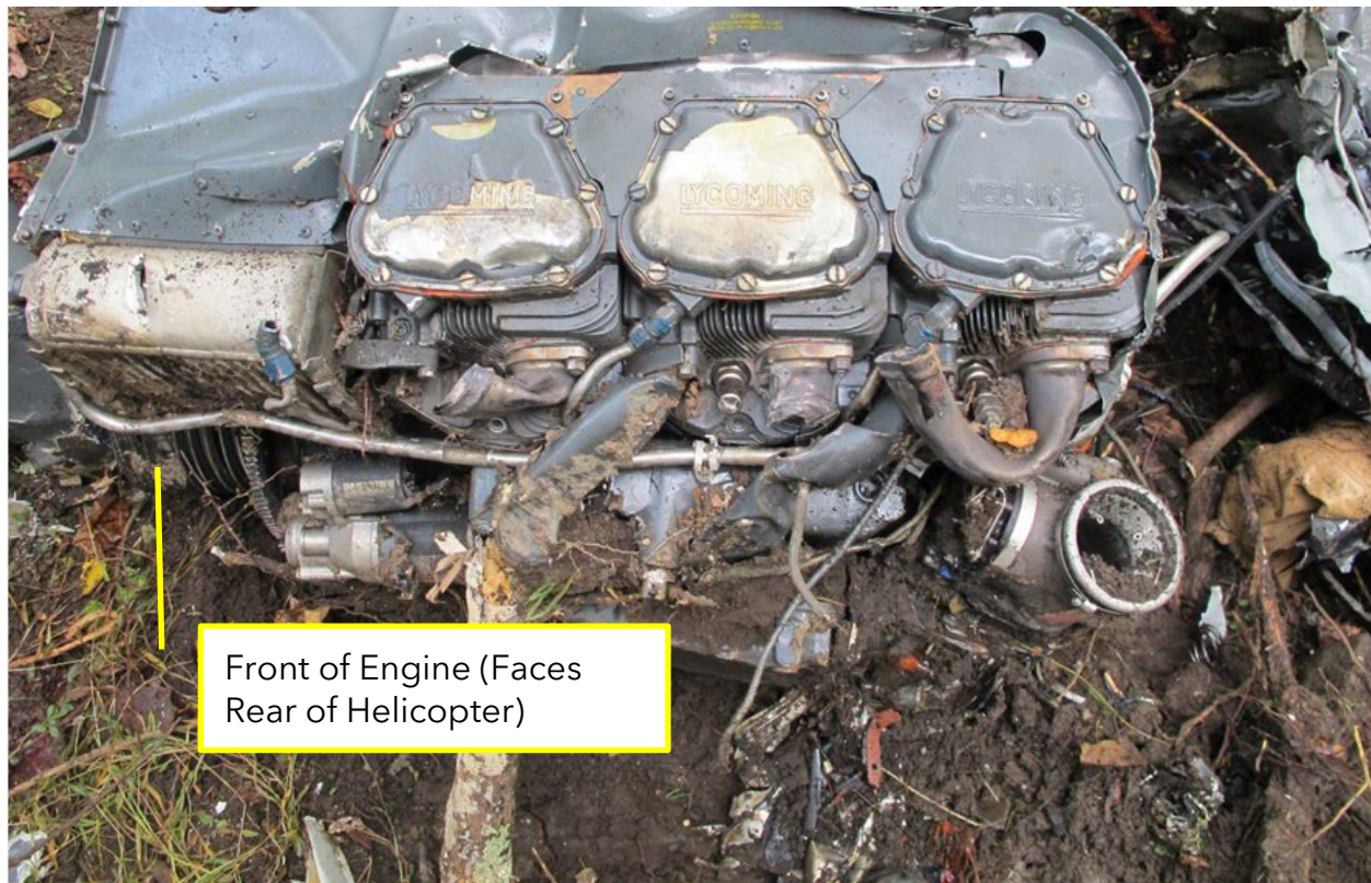
Figure 46 - Engine - View of Left Side (Note: The engine Faces Rearward in in the Helicopter)
