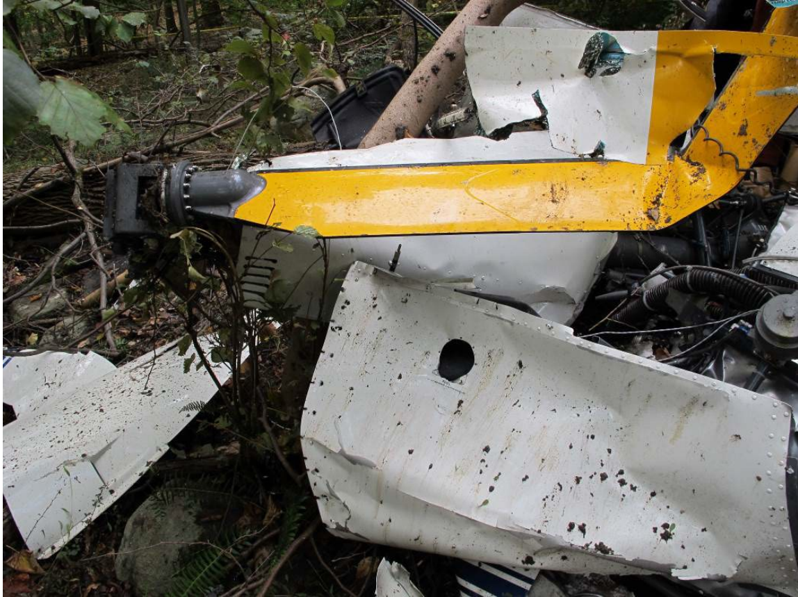
Figure 33 - Inboard Section of Main Rotor Blade S/N 10110
