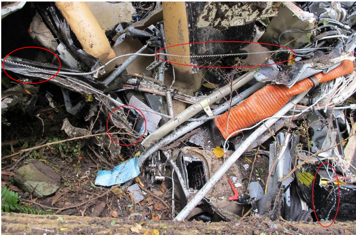
Figure 59 - Mixture Control Wire Sheathing Stretched Areas
