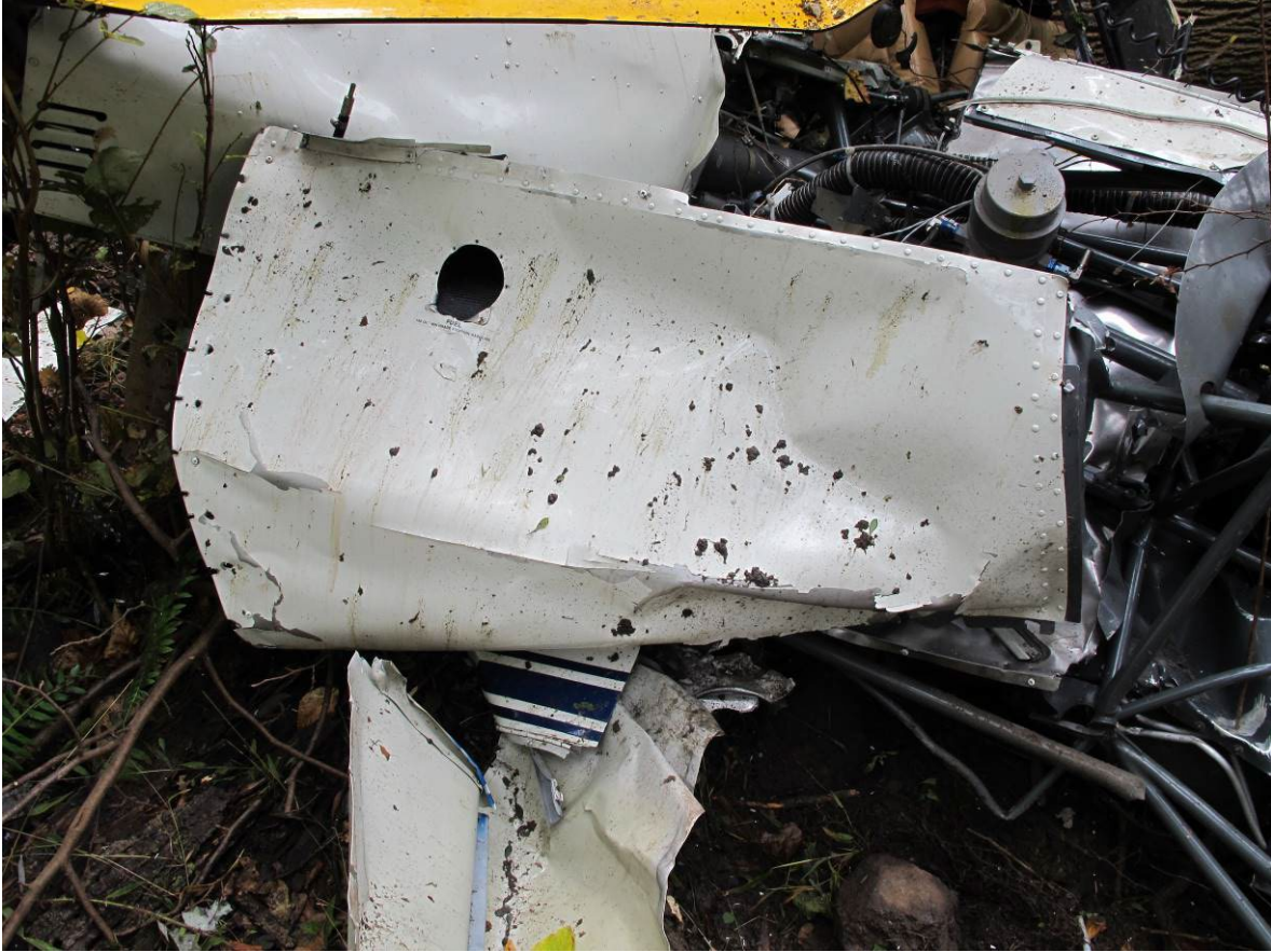
Figure 12 - Main Fuel Tank Shell
