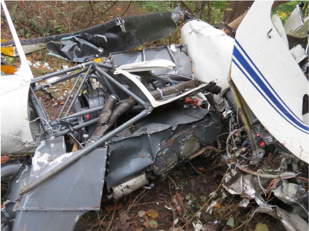
Figure 44 - Engine as Found
