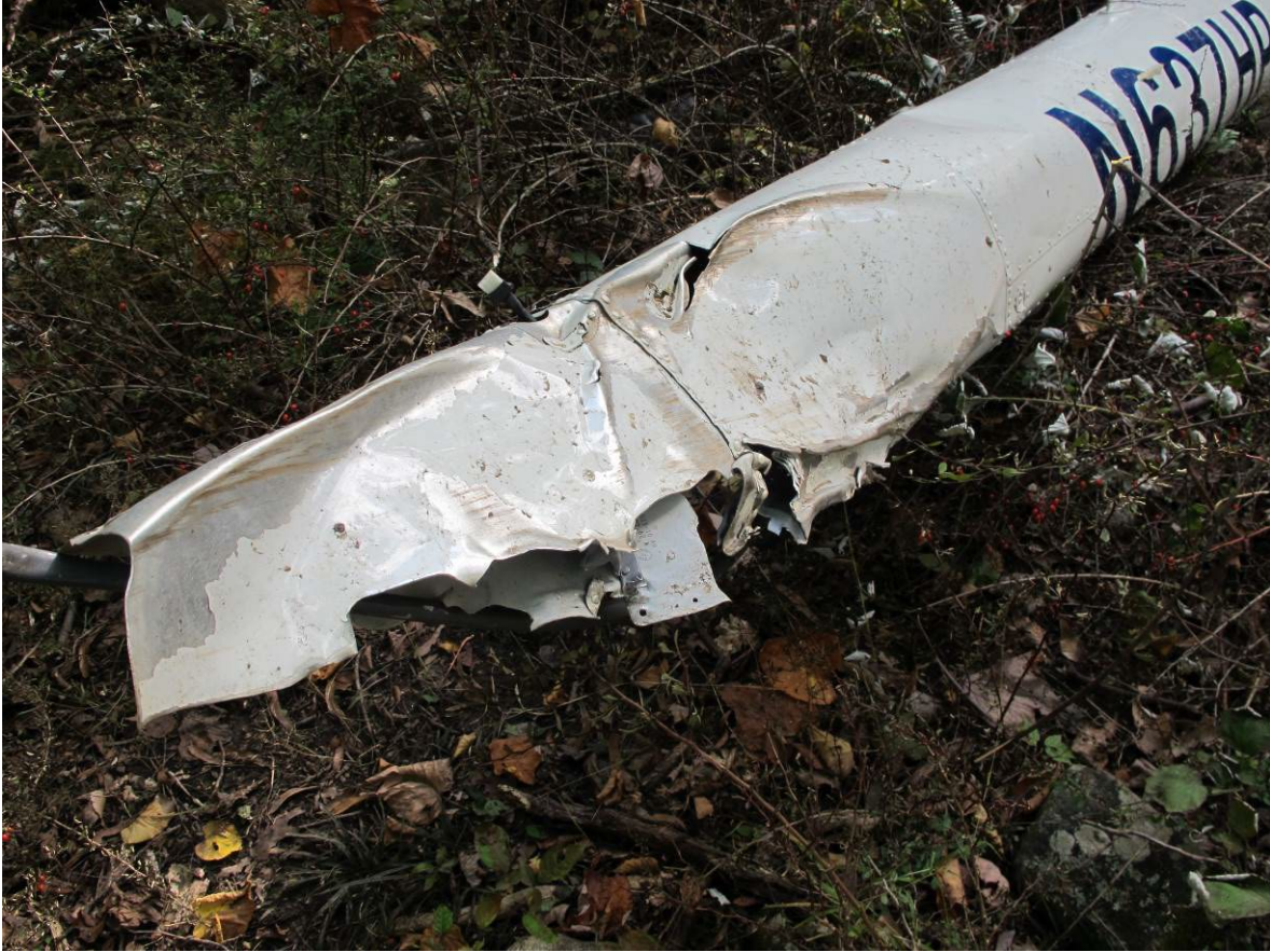
Figure 6 - Damage to Tailcone Bays 5 and 6
