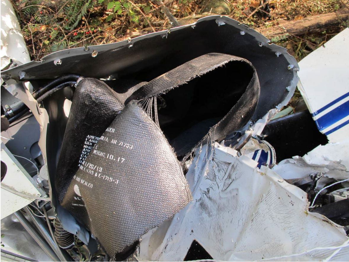
Figure 13 - Main Fuel Tank Bladder
