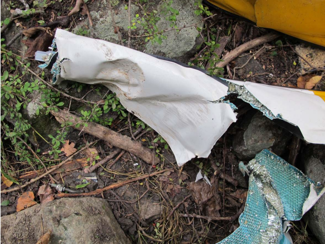
Figure 37 - Outboard Section of Main Rotor Blade S/N 10100 - Brown Residue on Upper Surface
