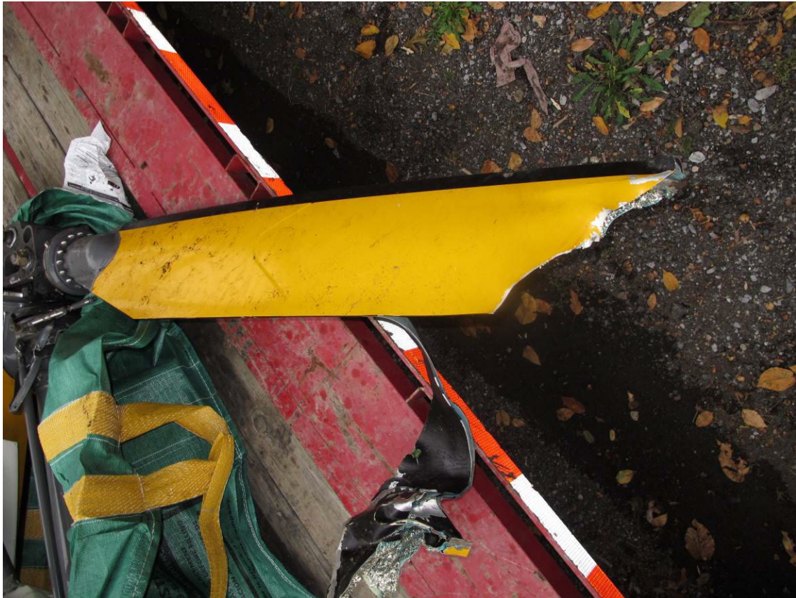
Figure 38 - Inboard Section of Main Rotor Blade S/N 10122
