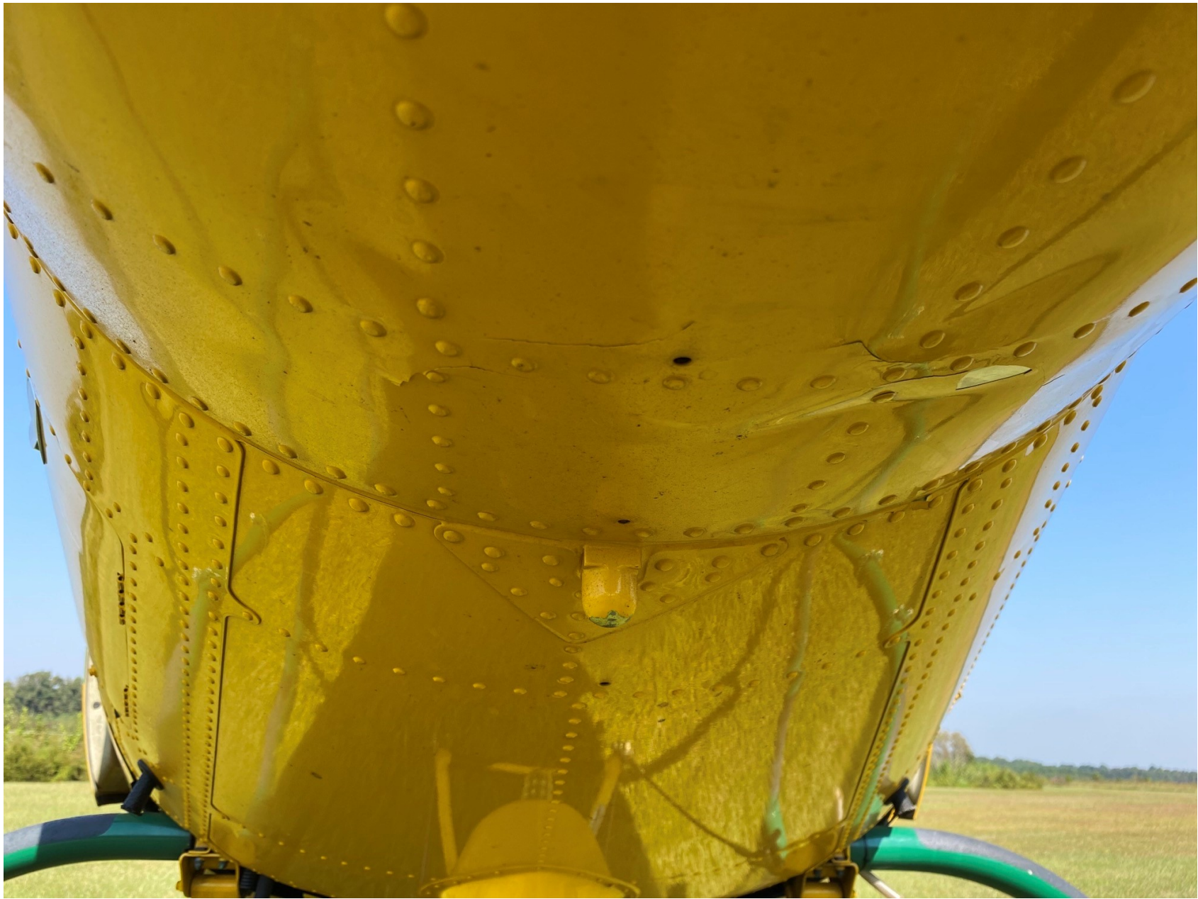
Photo 2 – View of bottom of tail boom showing buckling and cracked paint (Airbus Photo)
