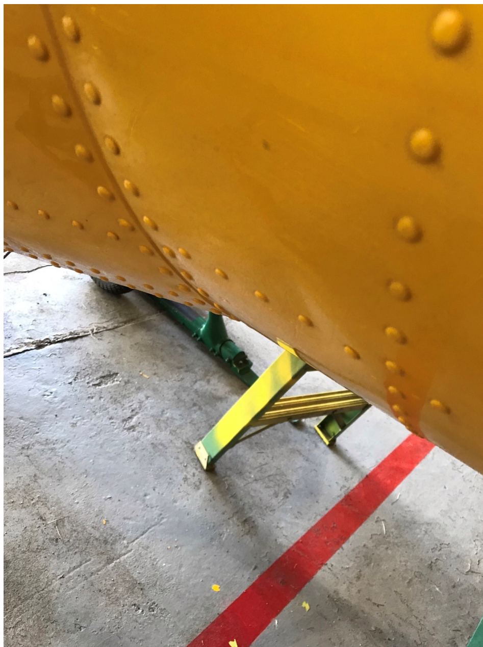
Photo 1 – View of left side of tail boom showing buckling (Airbus Photo)
