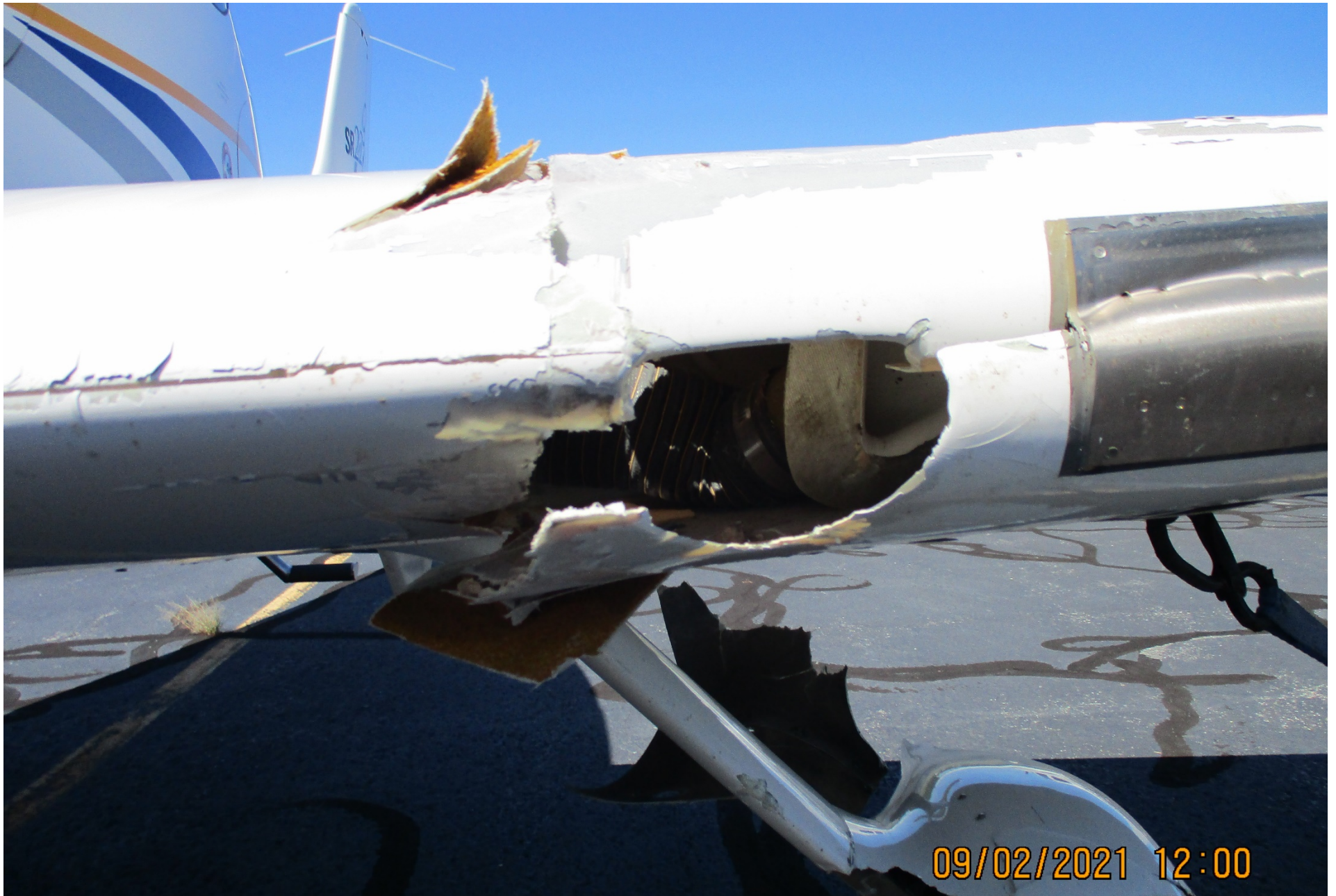
Photo 2 – view of left wing leading edge damage.
