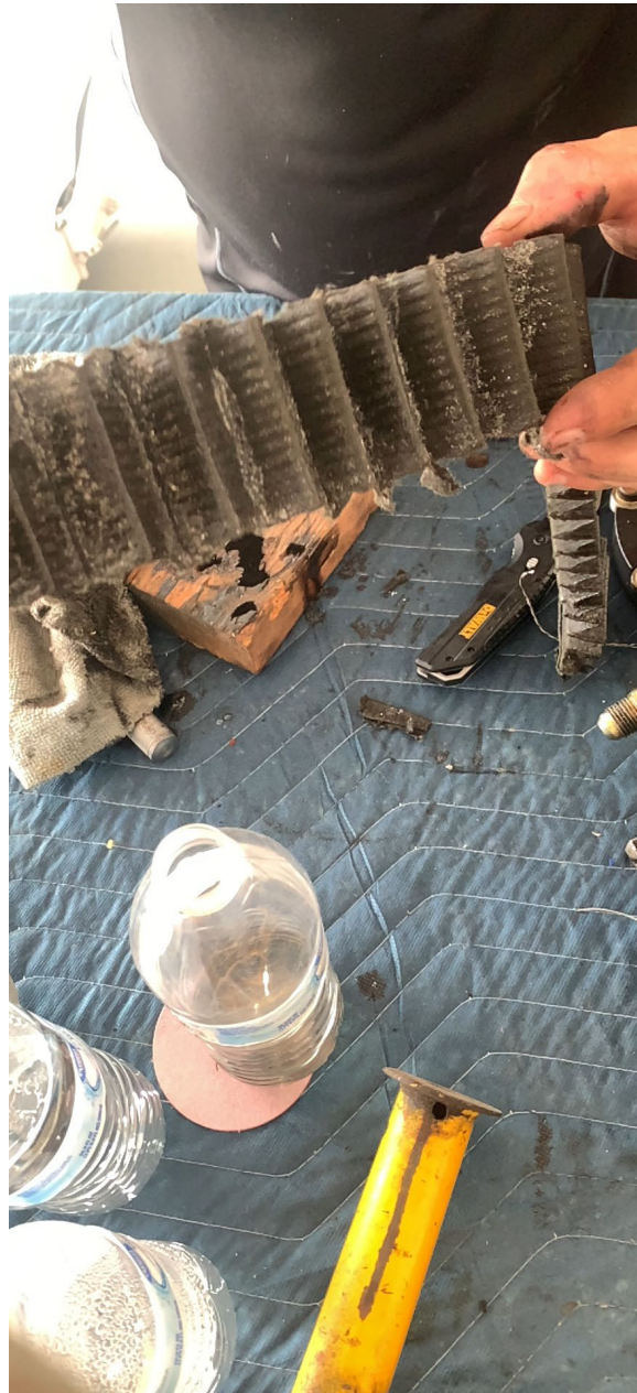
Photo 3 – Photograph From Owner/Operator. View of the Oil Filter Element. Note the non-ferrous Particles.
