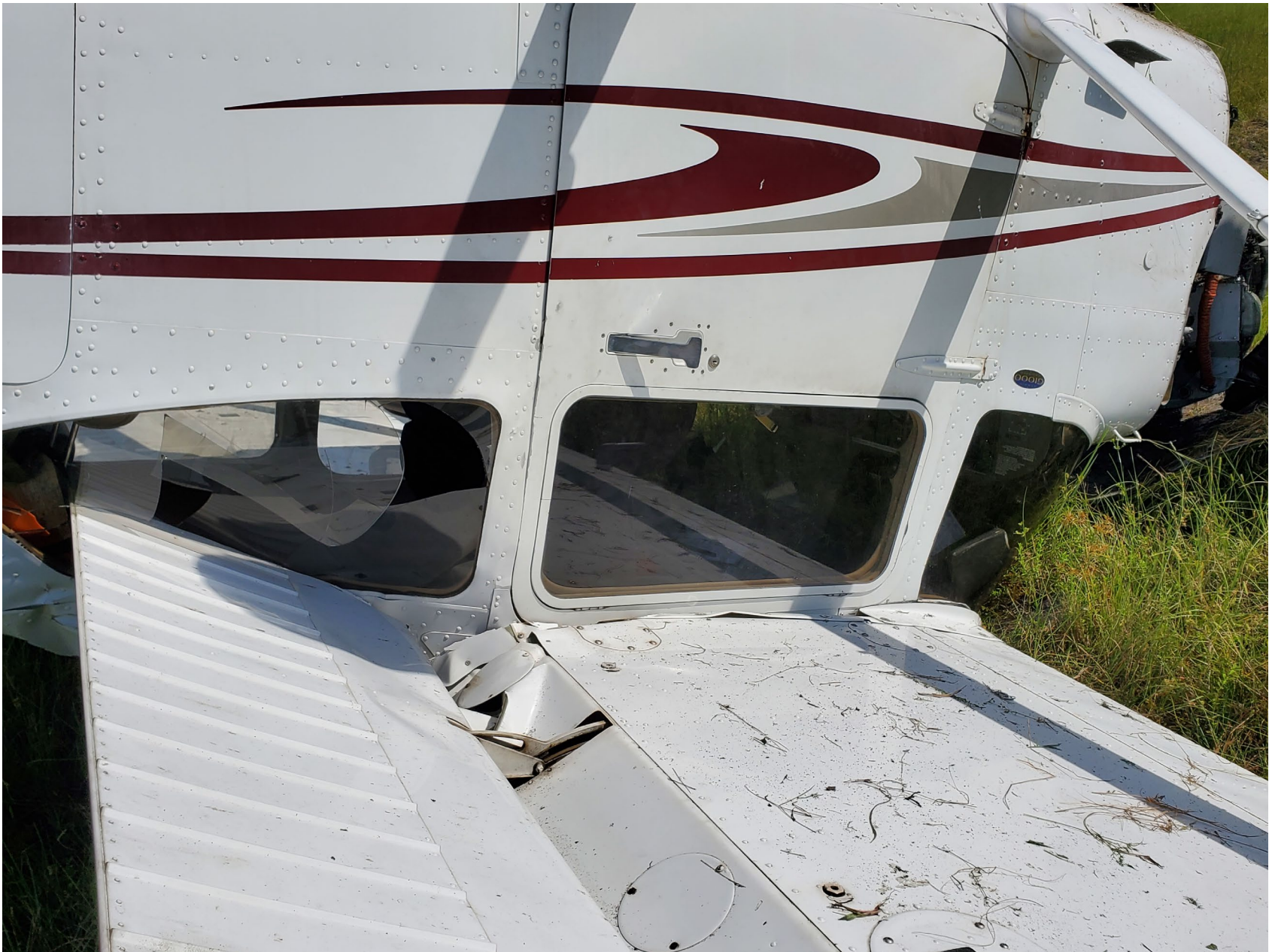
Photo 2 - FAA Digital Photograph. View of the Bottom Side of the Inboard Section of the Left Wing Noting Structural Damage.
