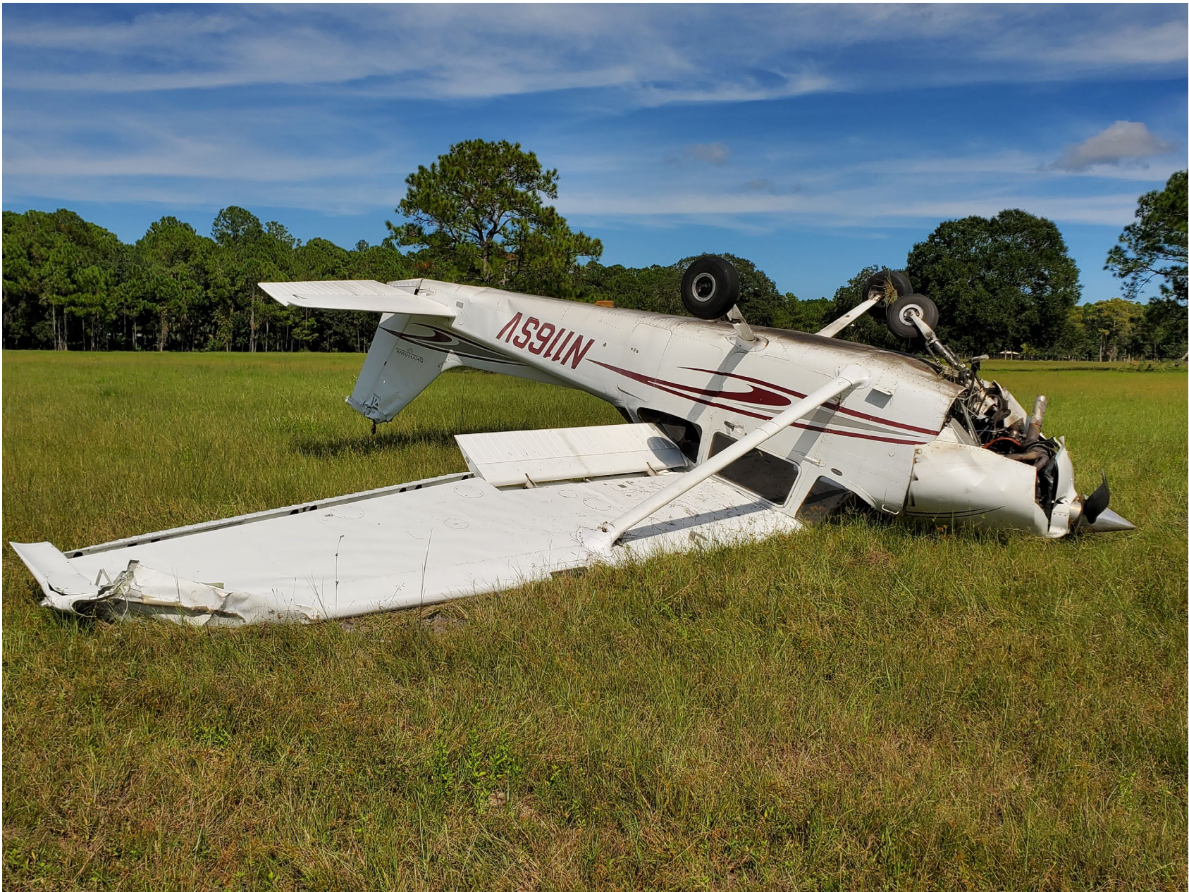
Photo 1 – FAA Digital Photograph. Left Forward View of the Inverted Airplane at the Accident Site. Note the damage to the Left Wing, and Bottom and Side of the Fuselage near the Left Horizontal Stabilizer.
