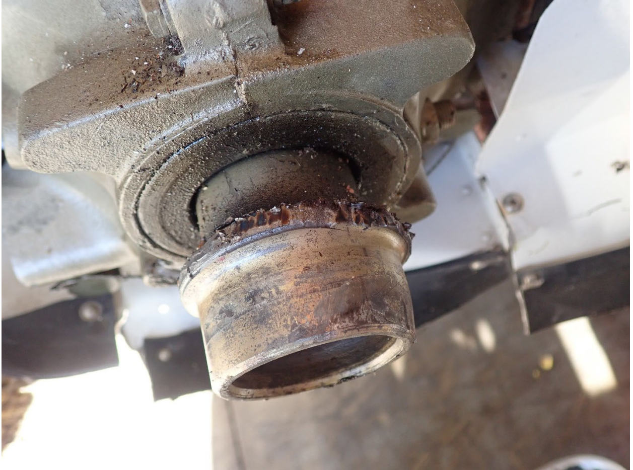
Figure 19 - Propeller Flange Fracture - Crankshaft Side
