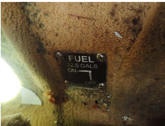
Figure 8 - Fuel Selector Placard
