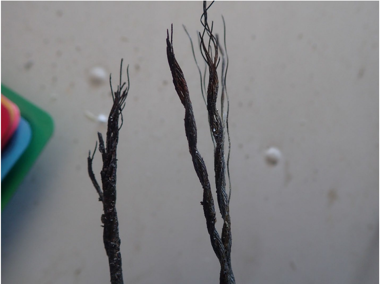
Figure 3 - Left Flap Cable Fracture
