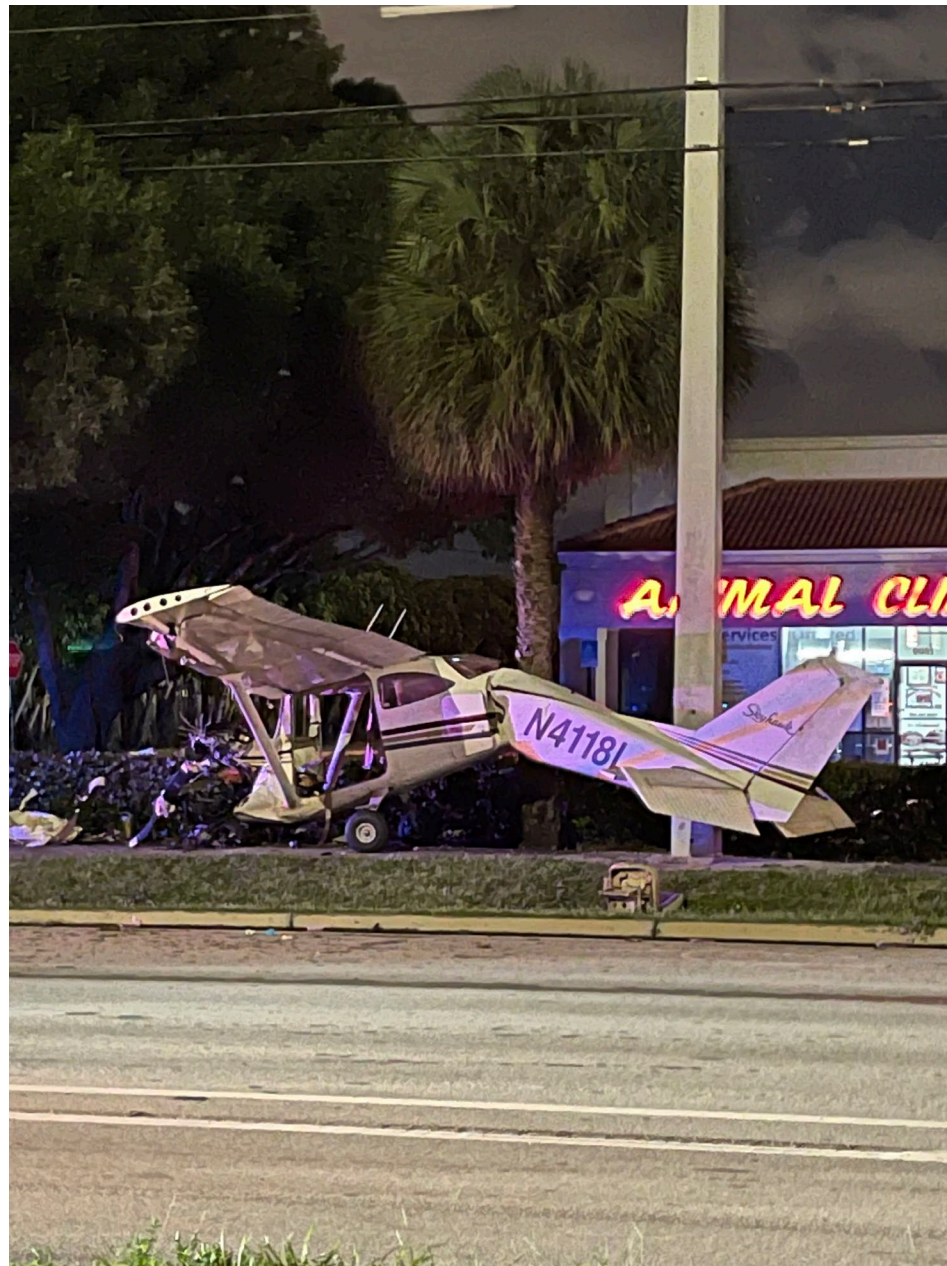
Photo 1 – FAA Digital Photograph. Left Side View of the Airplane at the Accident Site. Note the Substantial Damage to the Fuselage.
