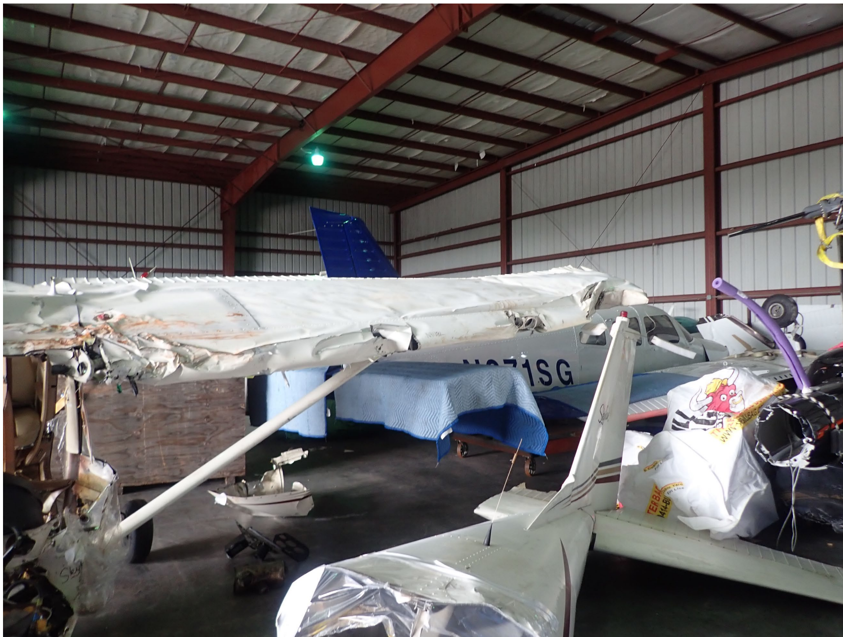
Photo 3 – Textron Aviation Digital Photograph. Front View of the Left Wing and Aft Empennage Separated For Recovery. Note the Substantial Damage to the Left Wing.
