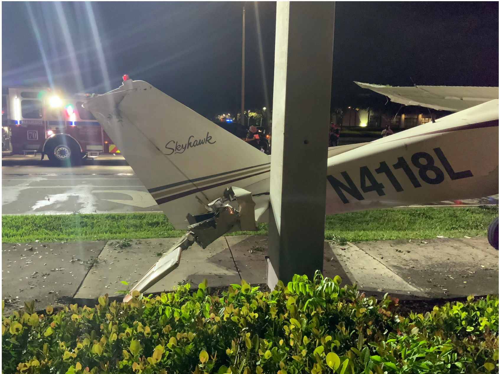
Photo 2 - FAA Digital Photograph. Right Side View of the Aft Empennage. Note the Substantial Damage to the Right Horizontal Stabilizer.
