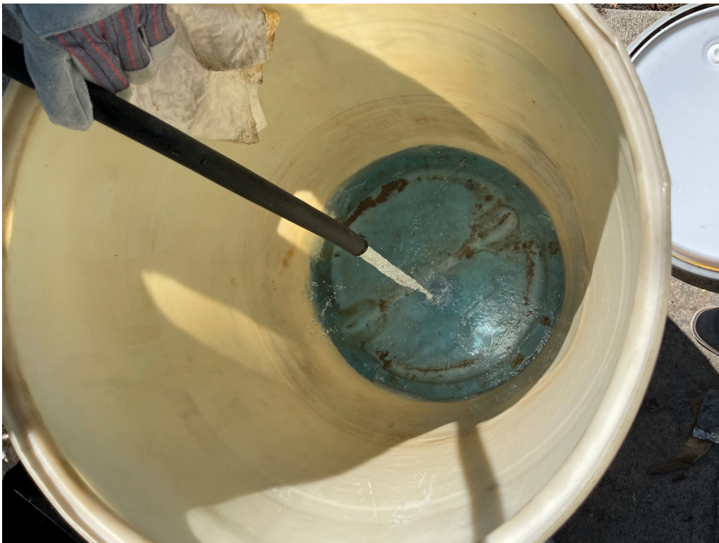
Figure 1: FAA Digital Photograph. View During Draining of the Fuel From the Left Fuel Tank.
