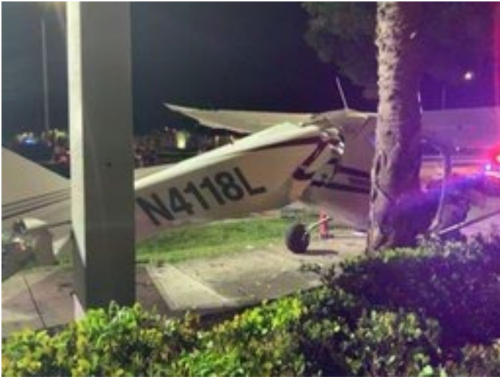
Figure 3: FAA Digital Photograph. Right side view of the Wreckage at the Accident Site. Note the Displaced Empennage.
