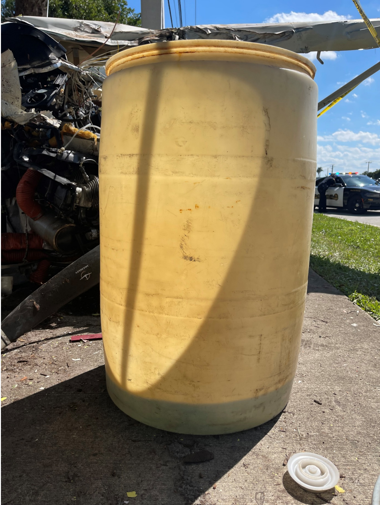
Figure 2: FAA Digital Photograph. View of the Fuel Drained from the Non-Breached Left Fuel Tank.
