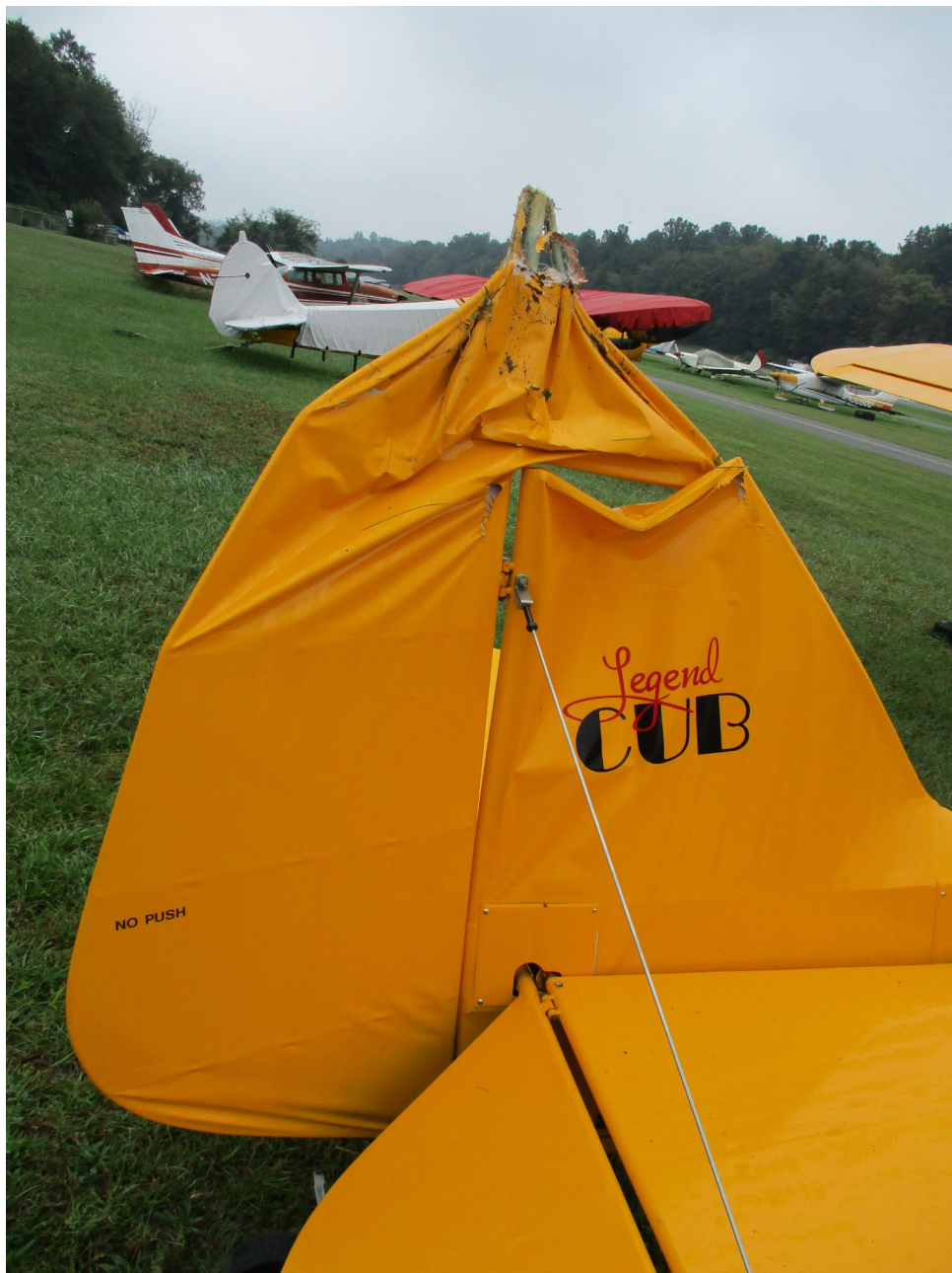
Photo 3 – Right side view of damaged vertical stabilizer and rudder. (Courtesy of FAA)
